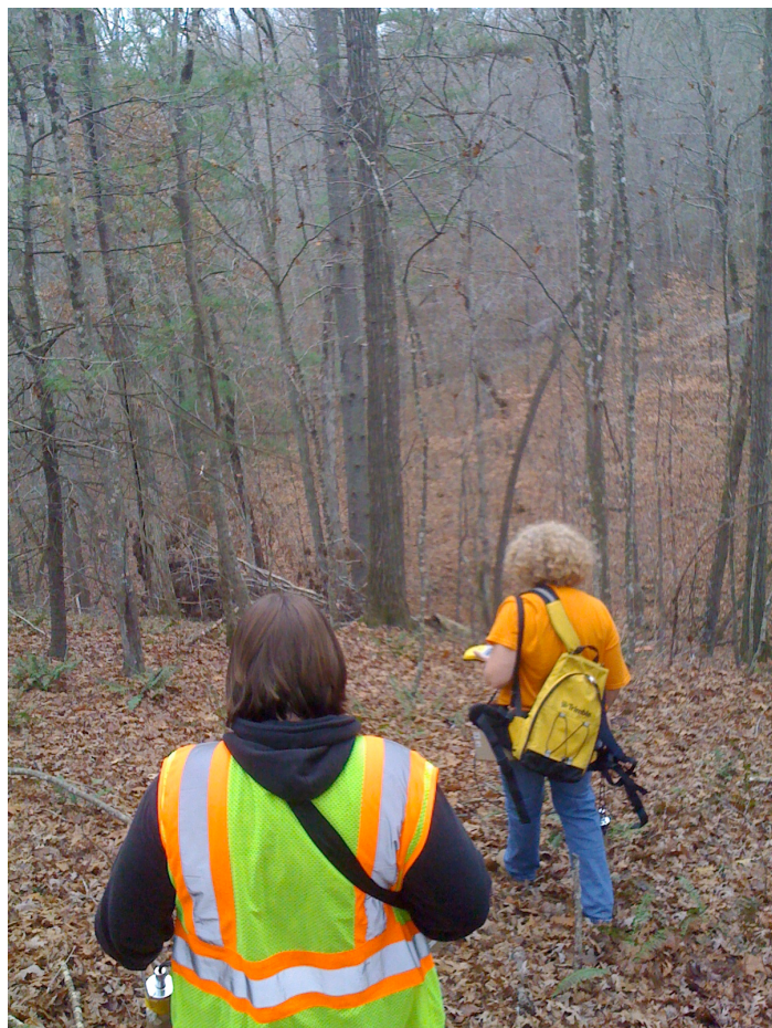
Figure A-2: Field Survey utilizing GPS Backpack and Portable NaI detector
