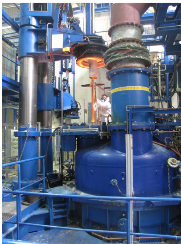
Fig.5: Maintenance of the plasma torch at GEKA
