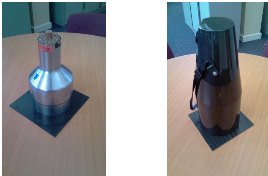
Figure 4a FIDLER probe on Am-241 planar source and 4b cased FIDLER probe (Groundhog Insight detector) on Am-241 planar source.
