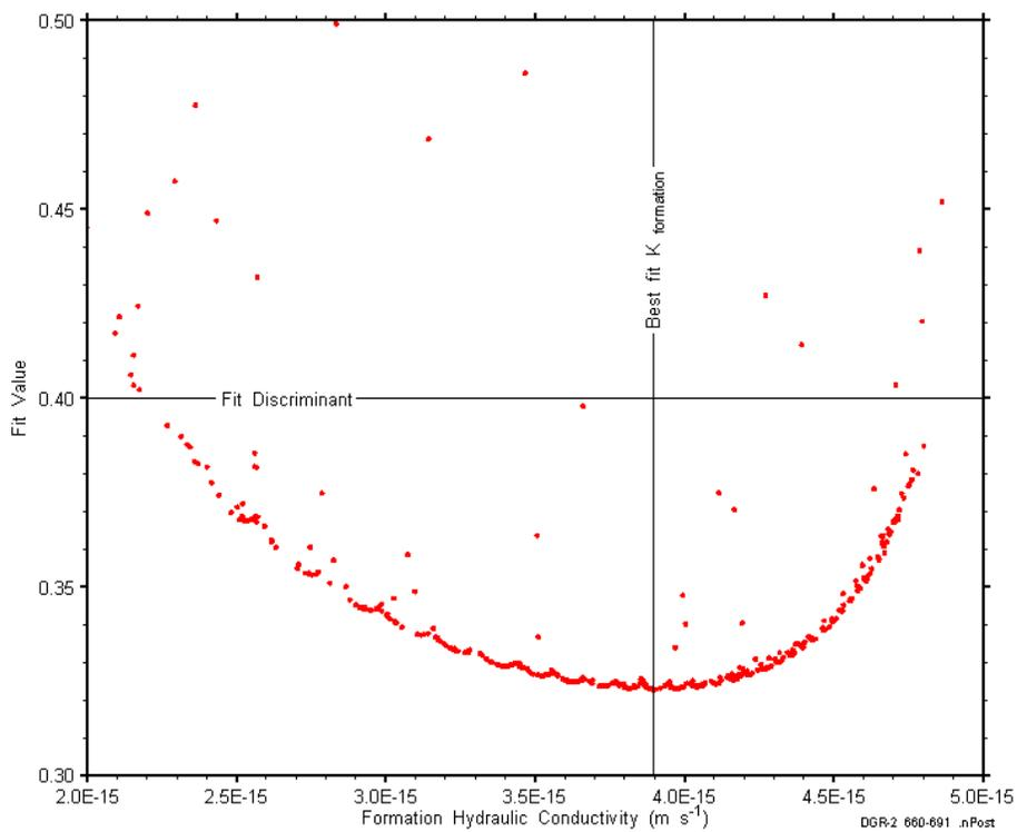
**Figure 5. XY-Scatter Plot Showing the Formation Hydraulic Conductivity Parameter Space Derived from the DGR-2 660.50-691.00 m Perturbation Analysis Along with the Fit Discriminant and Best-Fit Value**
