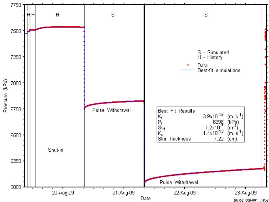
**Figure 7. Annotated DGR-2 660.50-691.00 m Testing Sequence Showing Best-Fit Parameter Estimates and 686 Accepted Simulations**
