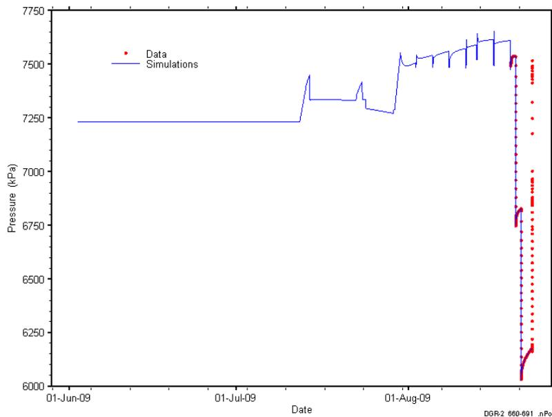
**Figure 3. Pressure History and Test Data for the DGR-2 660.50-691.00 m Testing Sequence Showing Best-Fit Simulations**
