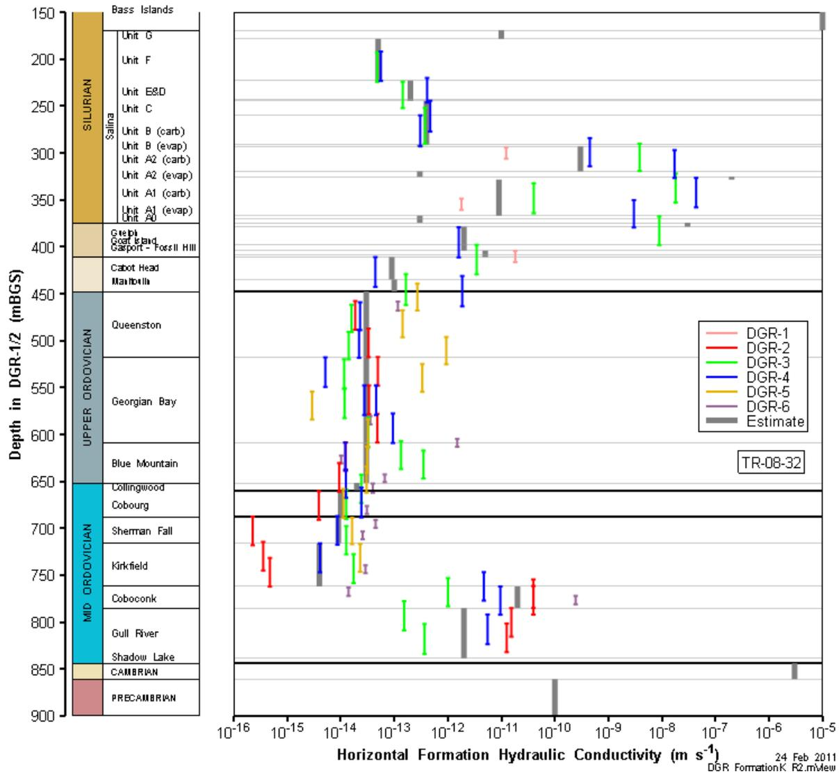
**Figure 8. Best-Fit Interval Horizontal Hydraulic Conductivities from Borehole Straddle-Packer Tests and Estimated Formation Average Values**
