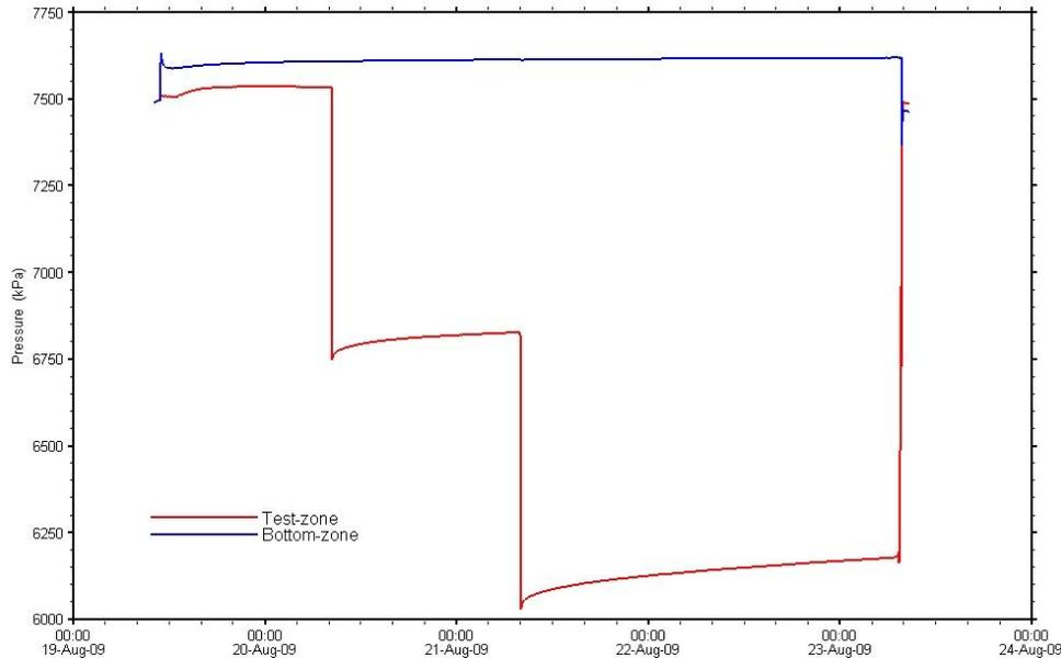
**Figure 2. DGR-2 660.50-691.00 m Test Interval and Bottom Zone Response**
