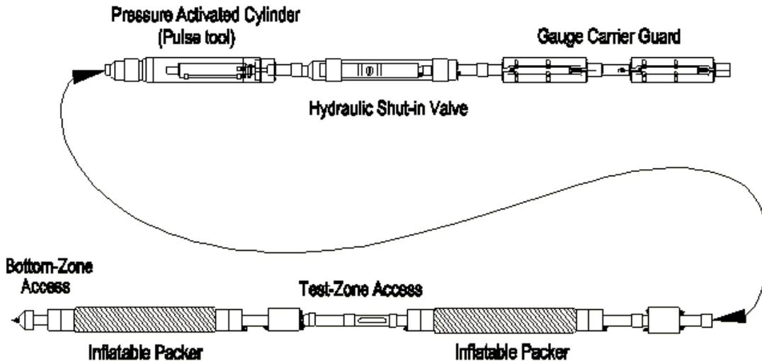
**Figure 1. Schematic of Straddle-Packer Test Tool**
