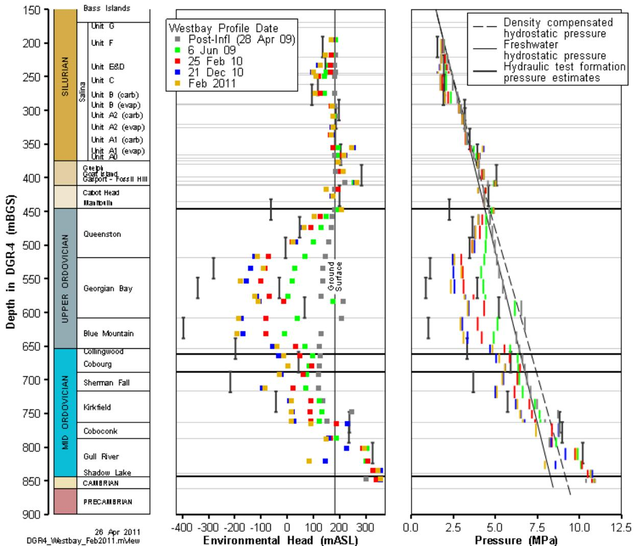
**Figure 9. Measured Westbay Pressures and Estimated Environmental Head Profile for Borehole DGR-4**
