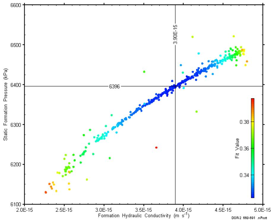
**Figure 6. XY-Scatter Plot Showing Estimates of Formation Hydraulic Conductivity and Raw Static Formation Pressure Derived from the DGR-2 660.50-691.00 m Perturbation Analysis**
