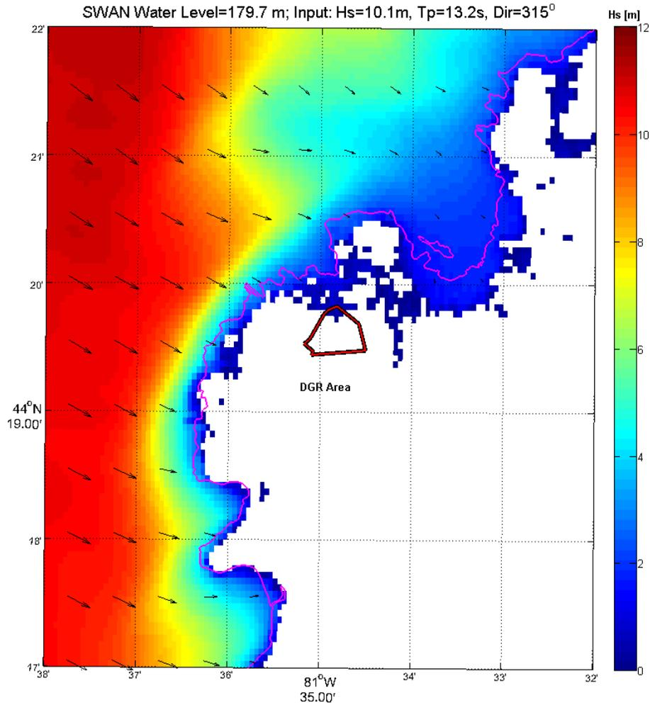
**Figure 9. SWAN wave height and direction propagation result over extreme still lake water level, including storm surge, of 179.7 m above chart datum IGLD 1985**
