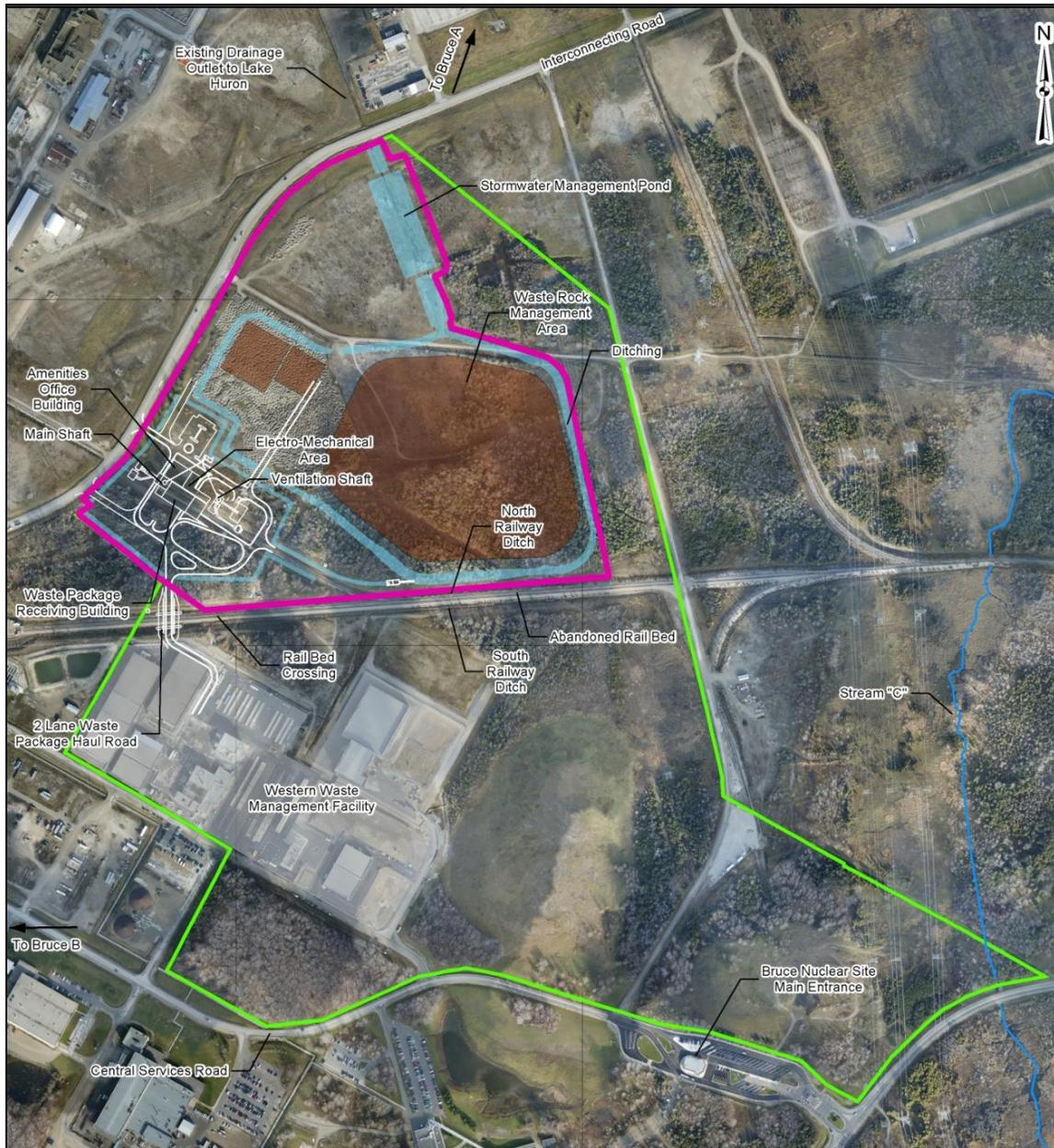
**Figure 1. Layout of the DGR project area**
