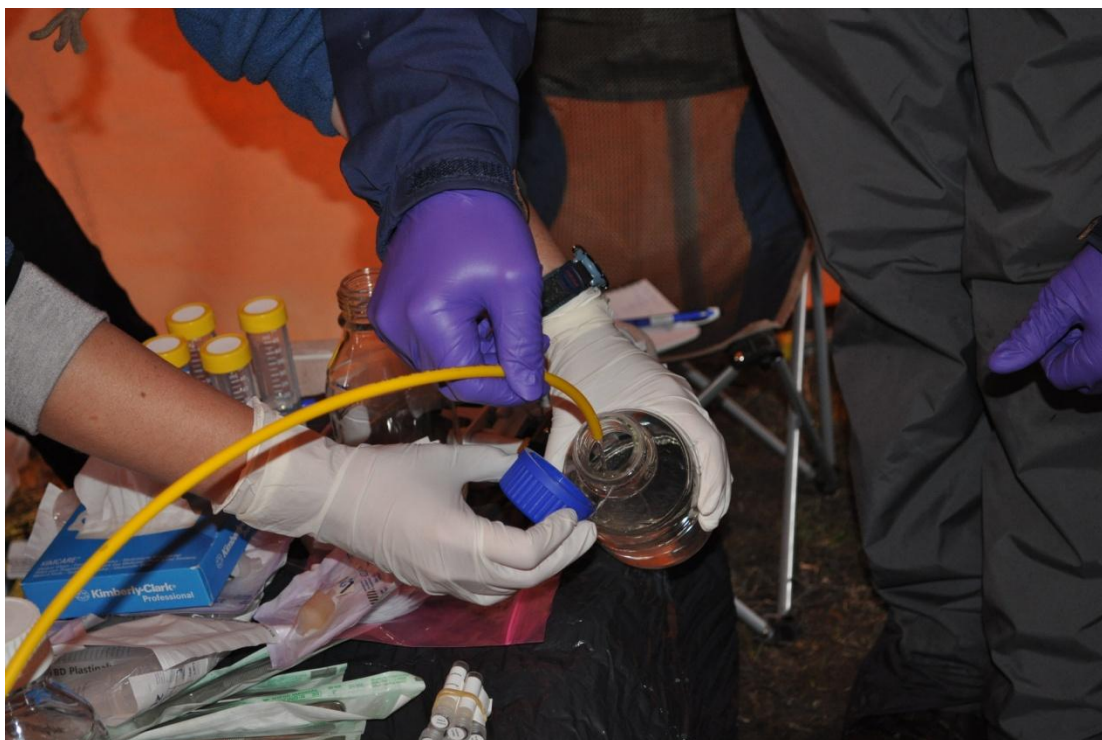
Figure 3. Collection of water samples for microbial analysis from borehole DH-GAP01.
