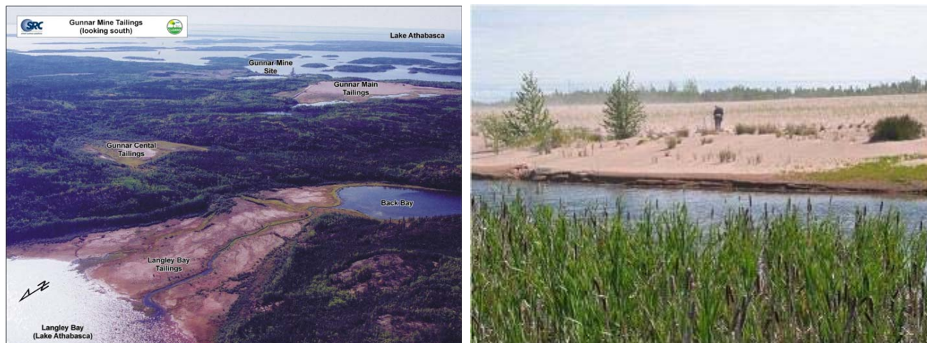
Figure 8. Overview of Gunnar unconfined tailings areas (left panel) and photo of wind blow at the surface of the Gunnar Main tailings (right panel) in 2008.
