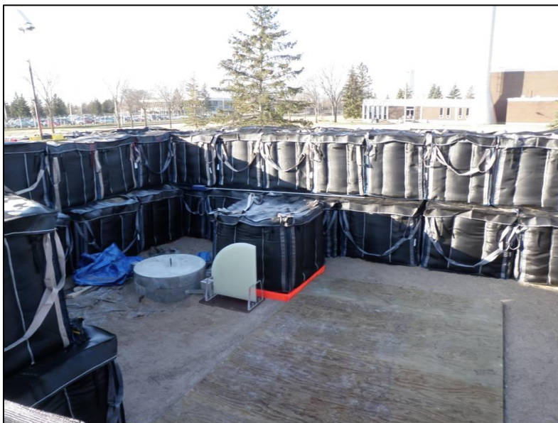
Figure 6. Mock standpipe and shielded enclosure set-up for axial radiography trials.
