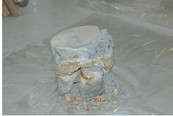
Figure 1. Surrogate cemented waste sample as removed from the pail.
