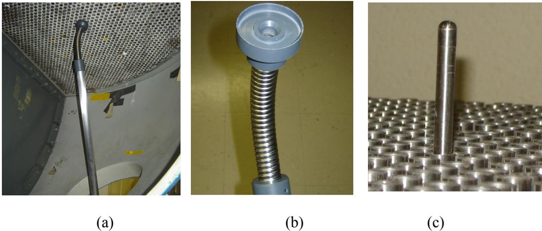
**Figure 4. CZT detector system showing (a) pole mounted delivery system inserted through man-way of mock-up (b) couplant used to engage with the tube sheet and (c) probe inserted through couplant into tube sheet**
