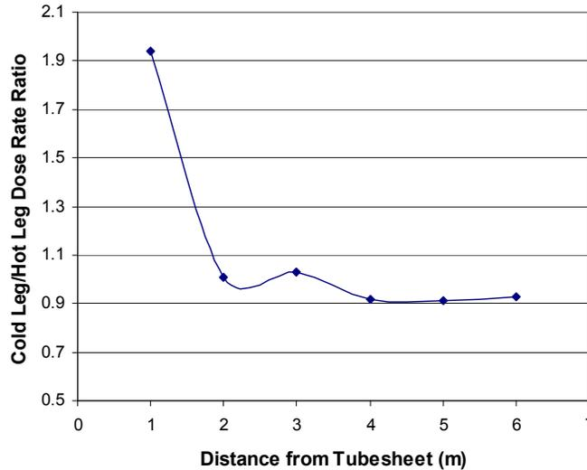
Figure 2. Variation in cold leg to hot leg dose rate ratio with distance from the tube sheet
