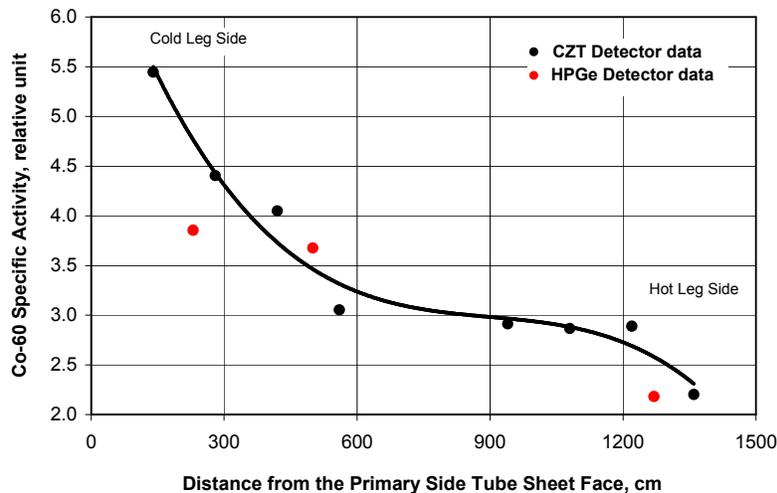
**Figure 5. Variation in measured Co-60 activity with tube length for an in-service steam generator**
