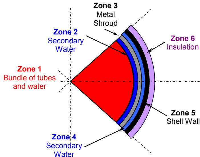
Figure 3. Shielding model for steam generator
