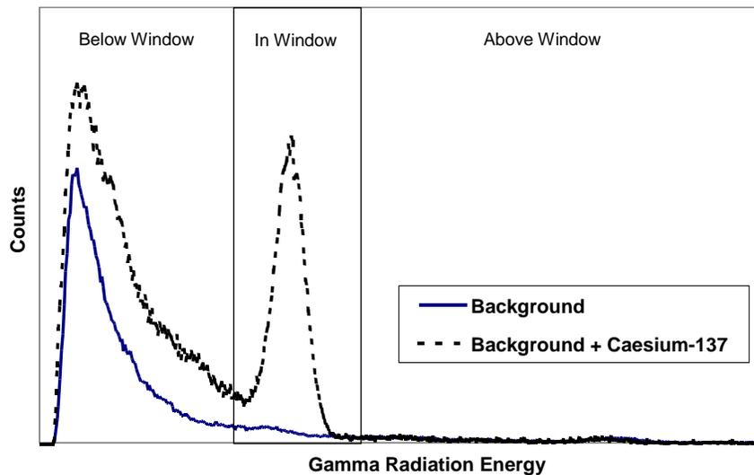
Figure 2 Low resolution spectrum of Cs-137
