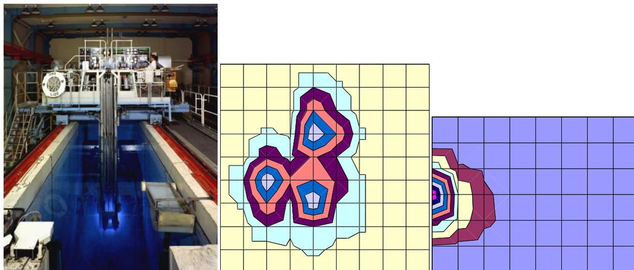
**Figure 3 (a) Lido swimming pool reactor showing the Cerenkov radiation; (b) gross gamma surface mapping of the inner wall of the bioshield; and (c) Co-60 activity profile into the wall of the bioshield.**
