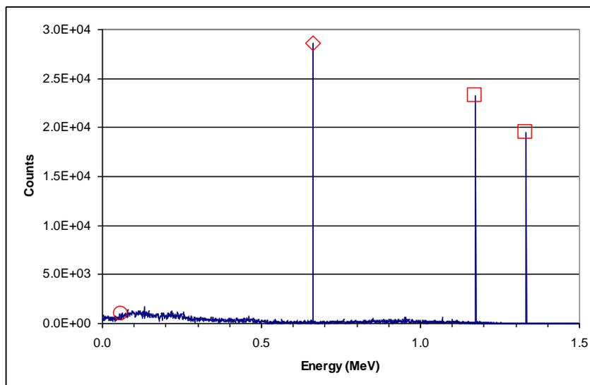
**Figure 1 High resolution spectrum of Cs-137 and Co-60**
