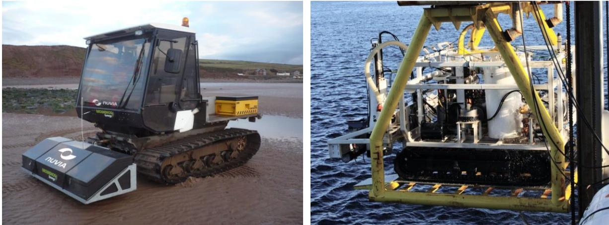
**Figure 5(a) Beach monitoring equipment, and (b) ROV deployed on the seabed for particle recovery.**
