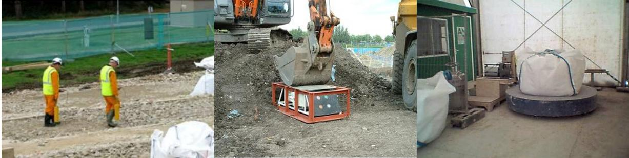
**Figure 6(a) Trench monitoring using Groundhog;
