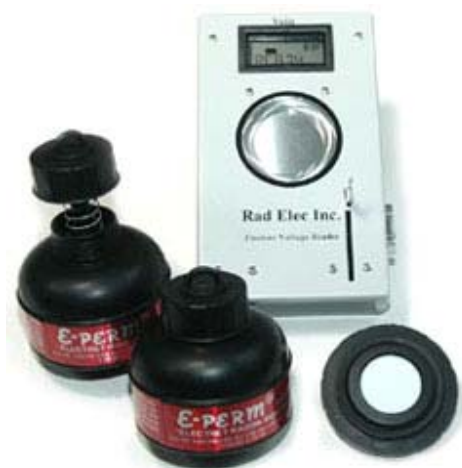
Figure 5: E-PERM Electret Detectors with Voltage Reader
