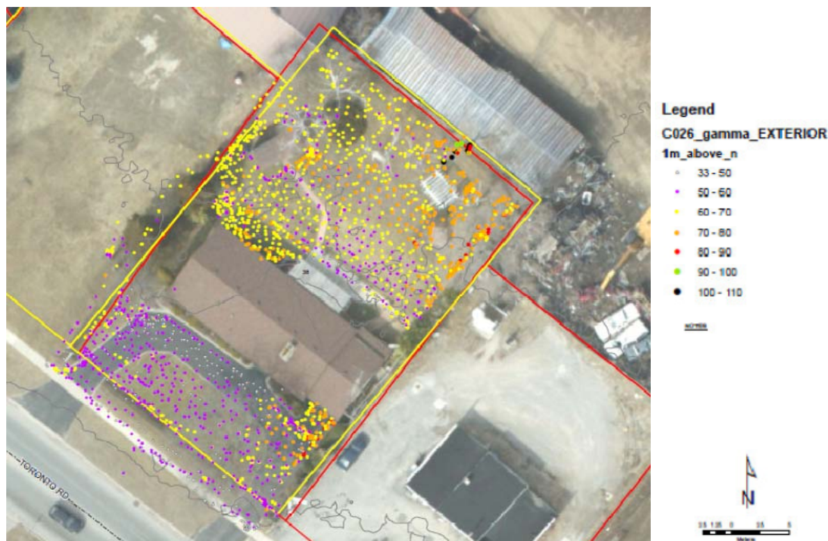
Figure 6. Example of Exterior Gamma Dose Rate Map of a Residential Site
