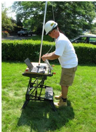
Figure 4: Recording Gamma Radiation in a Bore-Hole
