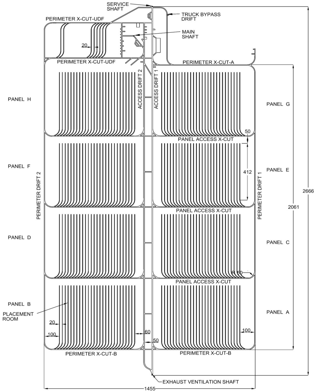
Figure 1. Plan layout of a proposed DGR using the HTP method [8].
