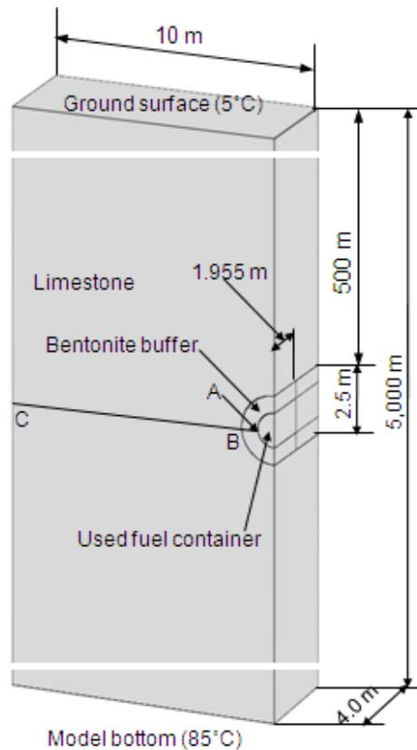
**Figure 3. Geometry and dimensions of the near-field model.**
