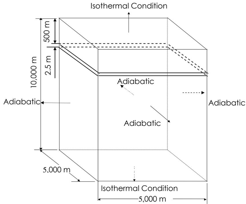
**Figure 7. Model geometry for a repository with infinite horizontal dimensions and the same density of thermal load as a repository with a finite horizontal repository.**
