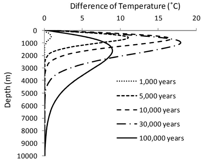
**Figure 9. Temperature differences along the vertical axis of the repository between using a horizontally infinite repository model and a finite repository model.**
