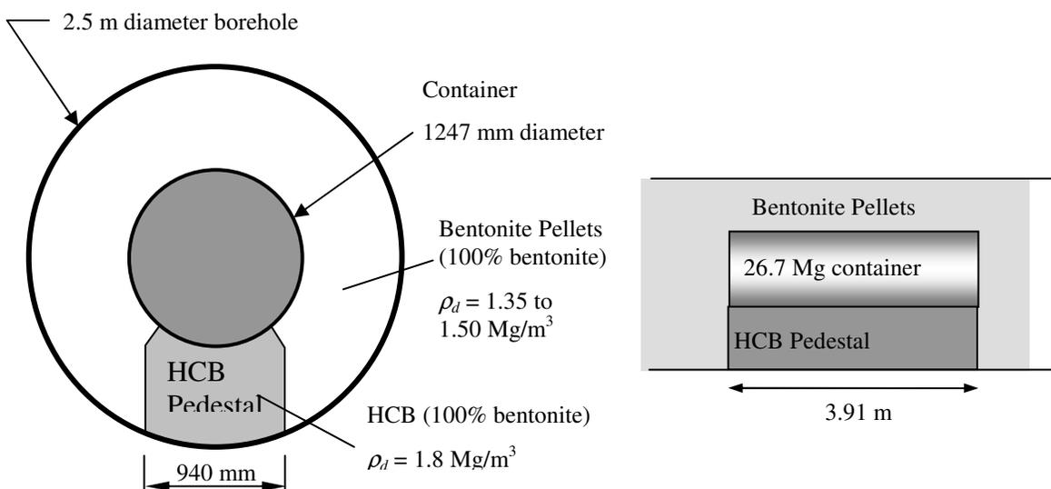
**Figure 2. Geometry of the horizontal canister (Container) placement option** (Figure provided by NWMO).
