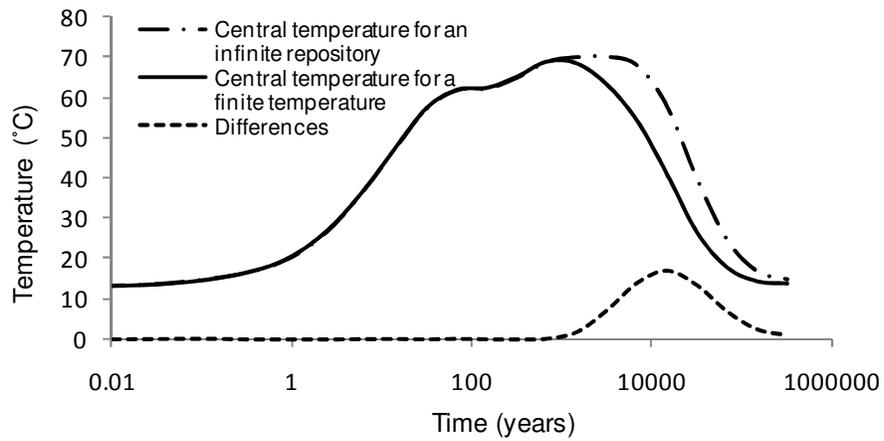
**Figure 8. Comparison of the central temperature between a finite repository and a horizontally infinite repository and their difference.**
