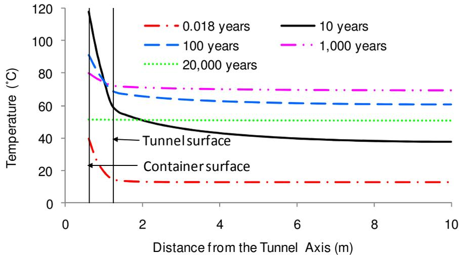
**Figure 5. Temperatures versus distance from tunnel axis along the horizontal line ABC (see Figure 3 for location) at five different times.**
