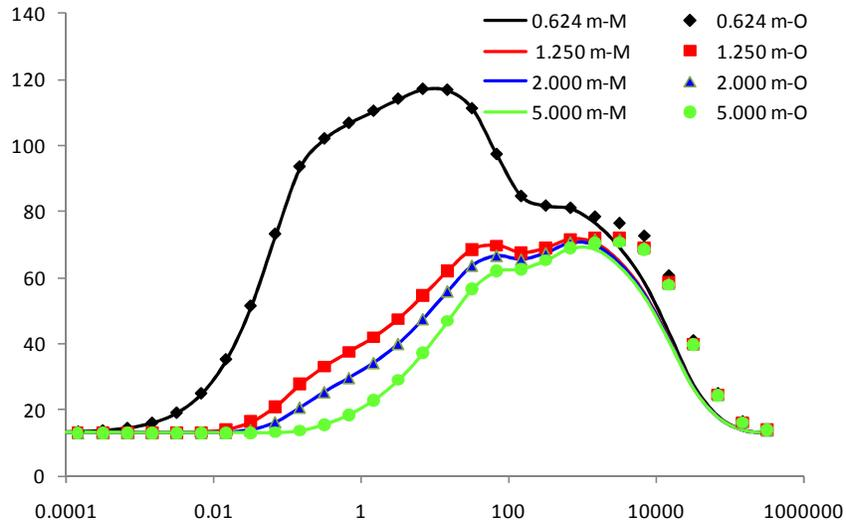
**Figure 10. Comparison of original and modified near-field temperatures at four different locations for a finite repository (In the legend: -M is modified, -O is original).**
