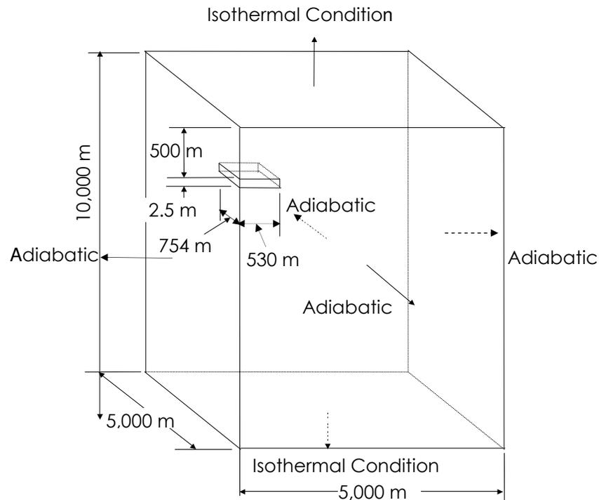
**Figure 6. Model geometry for a finite repository with the same total thermal load without considering the auxiliary unheated spaces.**
