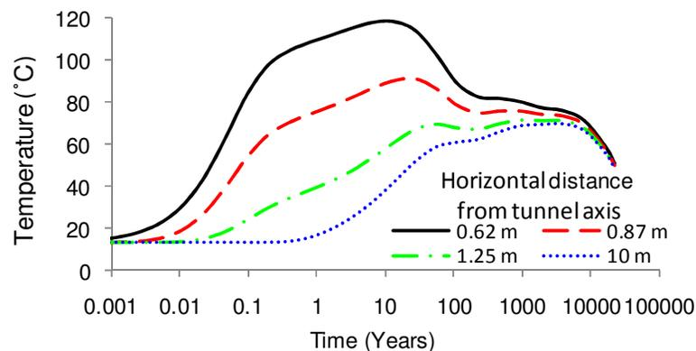
**Figure 4. Temperatures versus time at different distances from the tunnel axis along the horizontal line ABC.**
