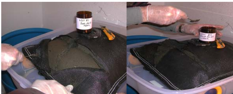
Figure 7: Bench Scale Test of Polymer Additive and Sediment Containment Bag Dewatering System
