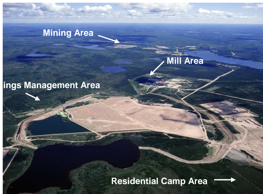
Figure 2. Aerial view of the Cluff Lake Project in 1999 during operations showing the four major areas of the site.
