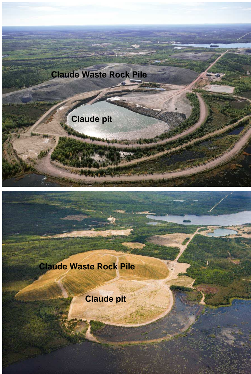
Figure 3. Mining area with Claude pit and Claude Waste Rock Pile in 1999 (top panel) during operations and in 2008 (bottom panel) after physical decommissioning.
