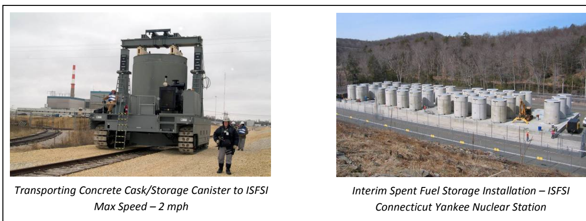
Figure 6. Transferring Fuel to ISFSI.
