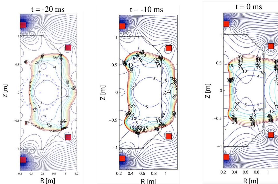
Figure 4 Temporal evolution of stray field in the plasma initiation phase, from left,  $-20$ ,  $-10$  and  $0$  ms (breakdown occurs), respectively. The cross markers represent the objective points in the least square fitting to solve the outer PF coil currents.
