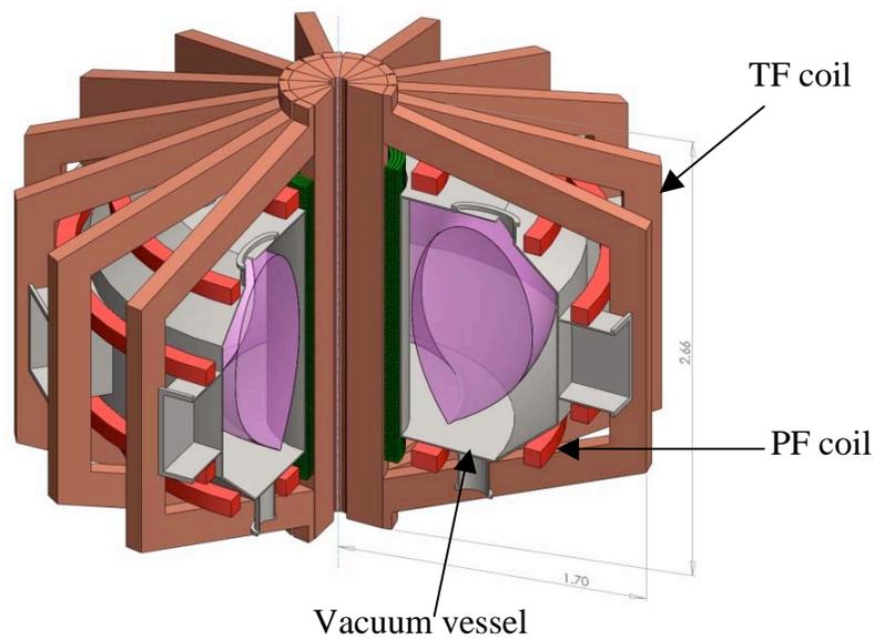
Figure 1 3D cut-away view showing the TF and PF systems and the vacuum vessel.
