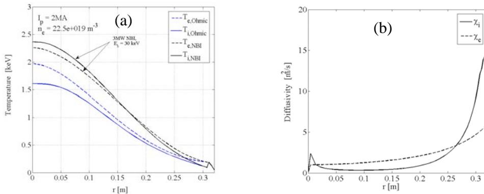
Figure 6 (a)  $T_i$  and  $T_e$  profiles for discharges with Ohmic heating and 3 MW NBI heating using ASTRA. (b)  $\chi_i$  and  $\chi_e$  profiles used in the simulation,  $\chi_i$  is neoclassical and  $\chi_e$  is parabolic, fitted using MAST data.
