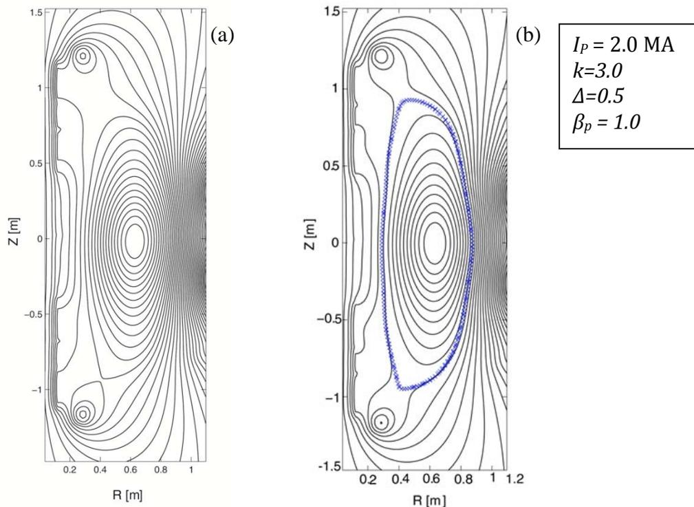
Figure 2 (a) SND configuration:  $I_p = 2.0 \text{ MA}$ ,  $k = 3.0$ ,  $\Delta = 0.5$  and  $\beta_p = 0.9$ , (b) DND configuration:  $I_p = 2.0 \text{ MA}$ ,  $k = 3.0$ ,  $\Delta = 0.5$  and  $\beta_p = 1.0$ . Line with markers shows the last closed flux surface (LCFS) in the DND configuration.
