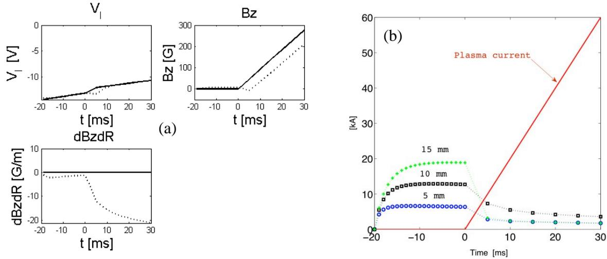
Figure 5 (a) Time traces of the parameters in STOR-U current start-up. (b) Wall thickness dependence of the eddy currents in the current start-up phase.
