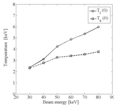
Figure 7 Predicted central ion and electron temperatures dependence on beam energy in on-axis NBI, plasma conditions:  $I_p = 2\text{ MA}$ ,  $n_e = 20e+019\text{ m}^{-3}$ .
