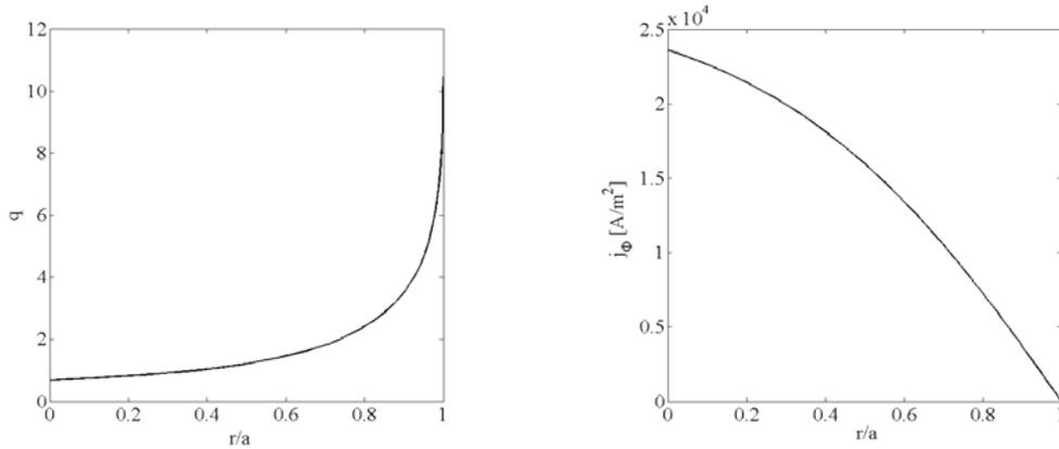
Figure 3 Radial profiles of safety factor  $q$  and toroidal current density  $j_\phi$  for the DND configuration.
