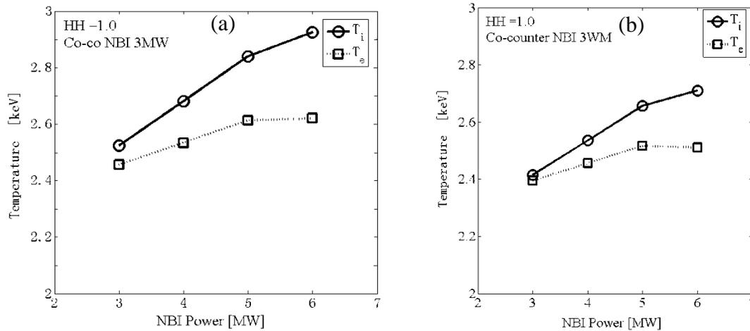
Figure 8 Central ion and electron temperature variations in co-co configuration (a) and co-counter configuration (b), plasma conditions:  $I_p = 2$  MA  $n_e = 20e+019$  m<sup>-3</sup>.
