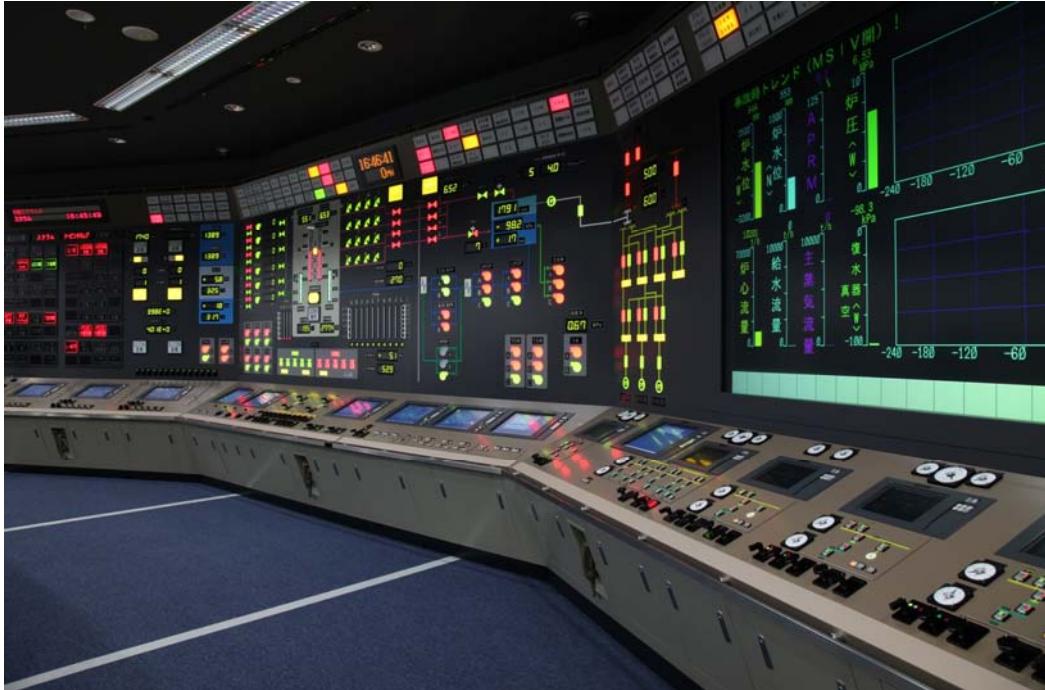
Figure 7 Overview of the latest ABWR simulator
