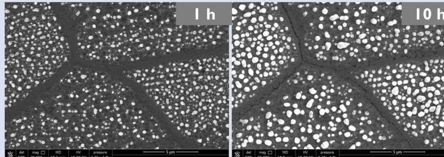
The surface coverage of nodules increases with exposure time mostly through growth of the existing nodules rather than nucleation of new ones. In some cases, adjacent nodules experience enough growth to impinge on one another and consolidate into one non-spherical nodule. Nodules close to the GB area grow less than the nodules in grain interiors and, in many places, stop growing altogether
