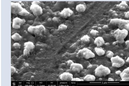
The relatively nodule-free zone along GBs undergoes changes as the exposure time increases. The initially smooth GB zone develops topographic contrast with increased exposure time.
