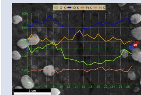
The nodule-free GB region shows enrichment in Ni and depletion in Cr and O. While most of the Ni diffuses towards the sample surface to form external nodules, Ni also diffuses towards GBs to relieve stress.
