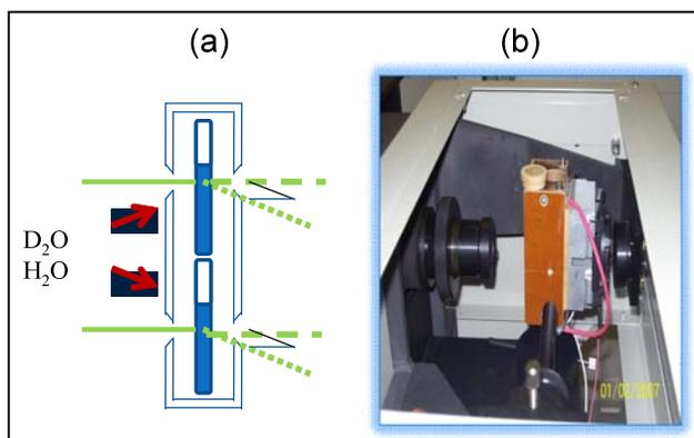
Figure 3 The proposed split cell design will analyze both light and heavy water simultaneously
