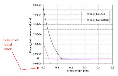
Figure 6: Fuel oxidation or reduction in radial cracks as a function of absolute radial position in the cracks from the r- $\theta$  model.
