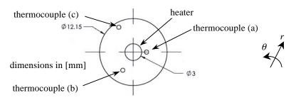
Figure 1: Radial cross section of planned test pellet with drill holes. The 3-mm diameter central hole is for the electrical heating wire. The smaller holes provide access for thermocouples and thermocouple wires. Thermocouple sites at: a) close to the pellet centre and near the heating element, (b) between the pellet centre and pellet outer surface and (c) near the outer surface of the pellet.
