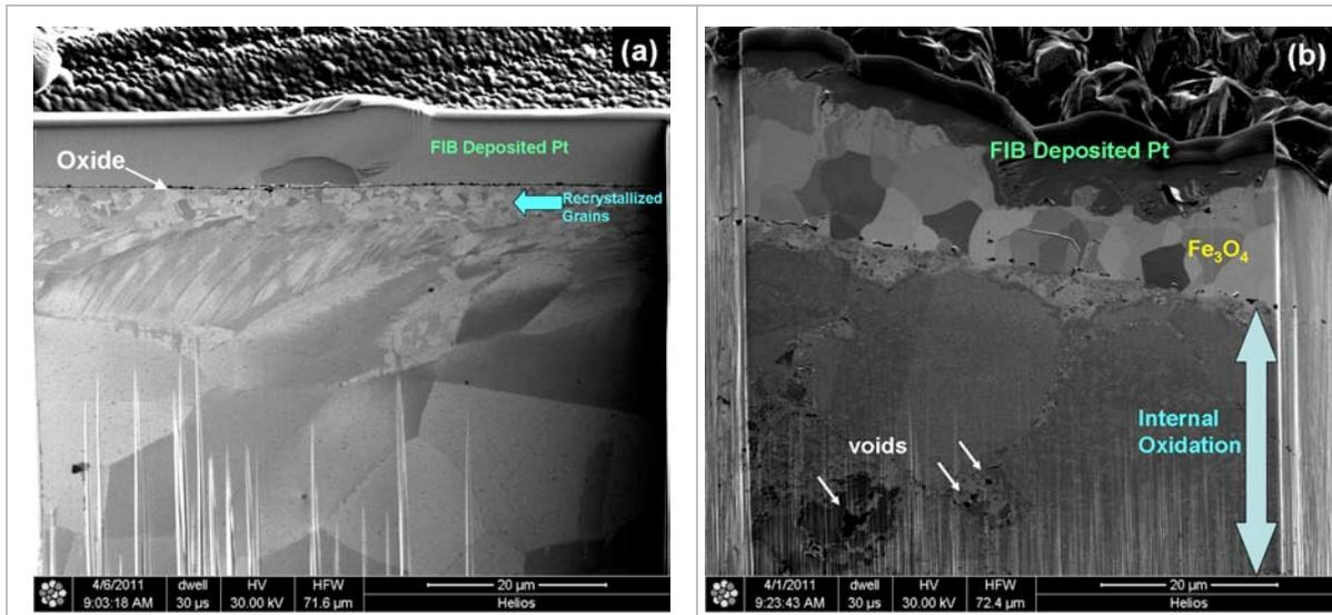
Figure 4 FIB cross section of the SCW tested 316L samples (a) machined surface, (b) 600-grit polished
