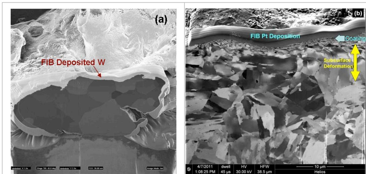
Figure 2. FIB images (a) atomized Fe-25%Cr particle for coating, (b) severely deformed structure in both coating and top surface of the P91 test coupon
