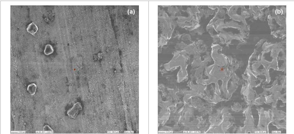
Figure 3 SEM images of surface morphology after SCW exposure (a) machined surface, (b) 600-grit polished.
