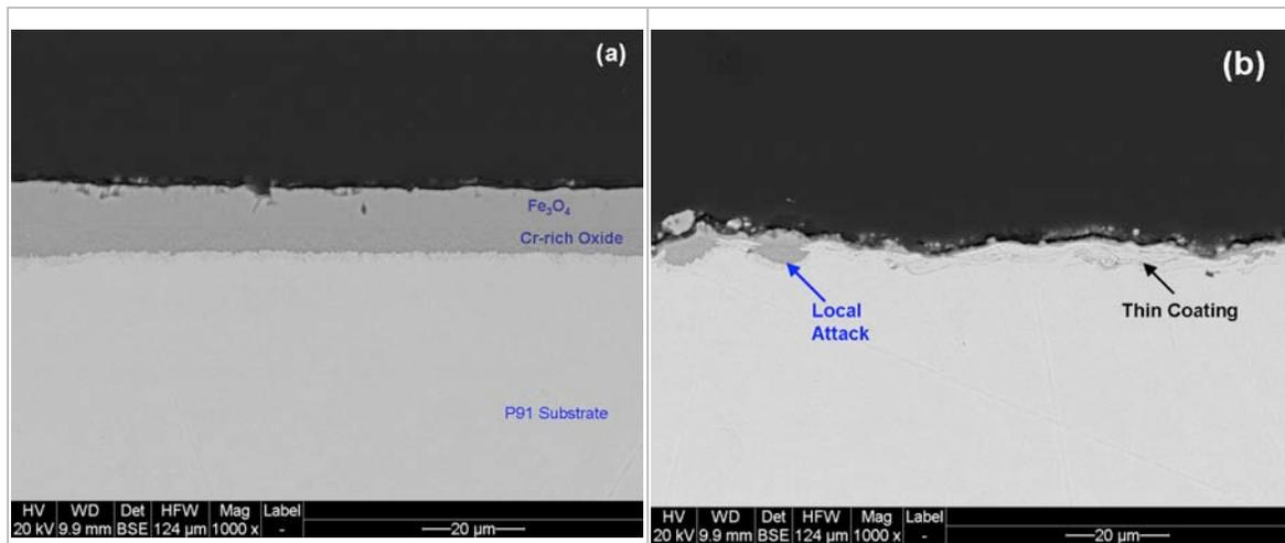
Figure 1 SEM images of test coupons after SCW test (a) bare P91 steel; (b) coated P91 steel
