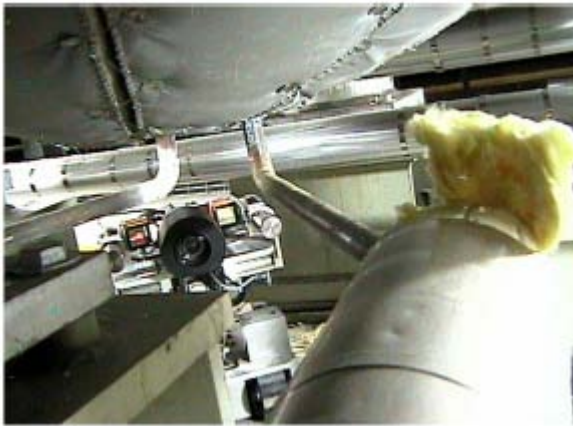
Fig. 12. Gamma Probe and Camera Robot locating debris.
