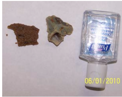
Figure 6: Two pieces of solid material floating on the open surface of the moderator were retrieved for material analysis. As shown, there is a variation in color, thickness and texture of the samples.
