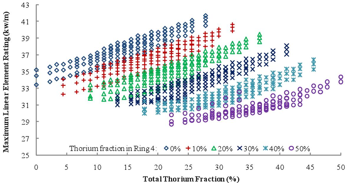
Figure 6: Maximum linear element rating as a function of thorium content
