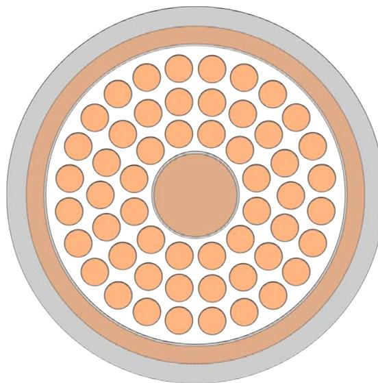
Figure 1: 54-element bundle contained within a HEC.
