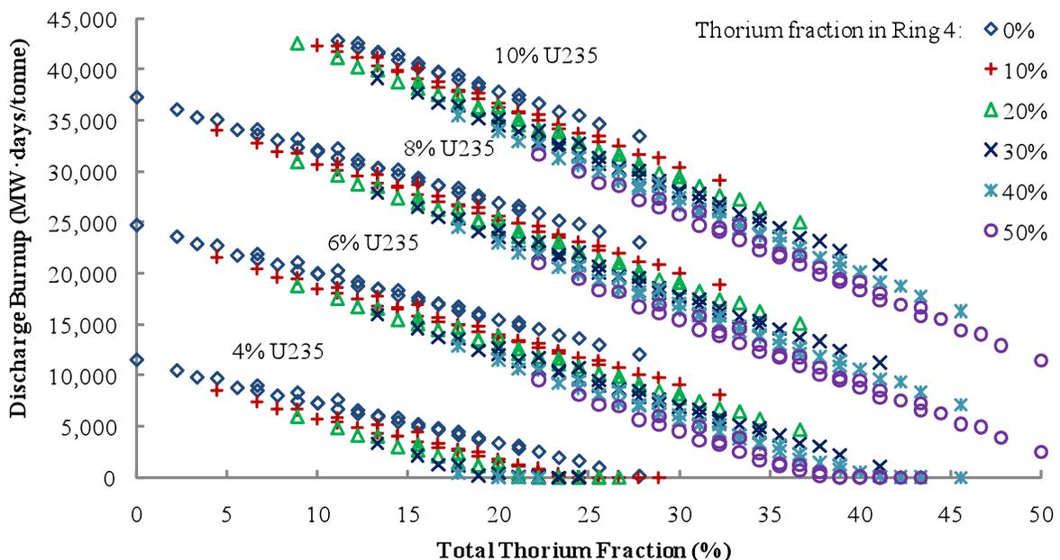
Figure 4: Discharge burnup as a function of total thorium content and content in ring four
