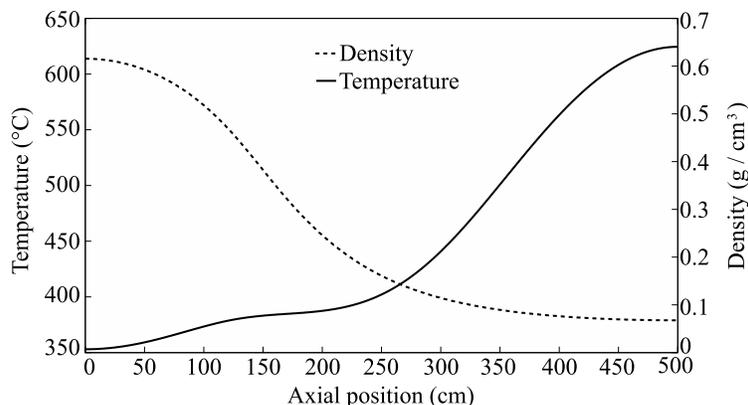
Figure 1 Coolant properties along a pressure tube SCWR fuel channel
