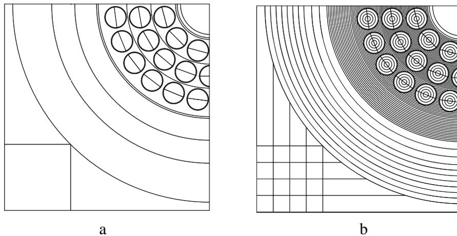
Figure 3 Geometries used for the resonance self-shielding (a) and the main flux (b) calculations
