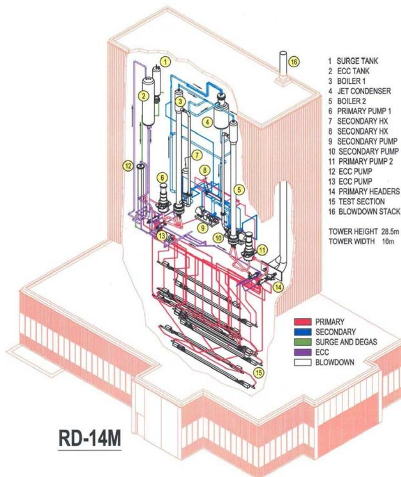
Figure 1 RD-14M loop layout
