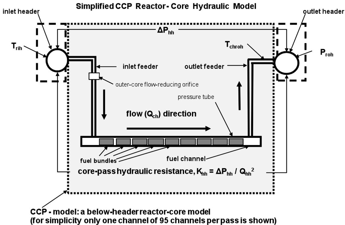
Figure 2 Simplified CCP reactor-core hydraulic model
