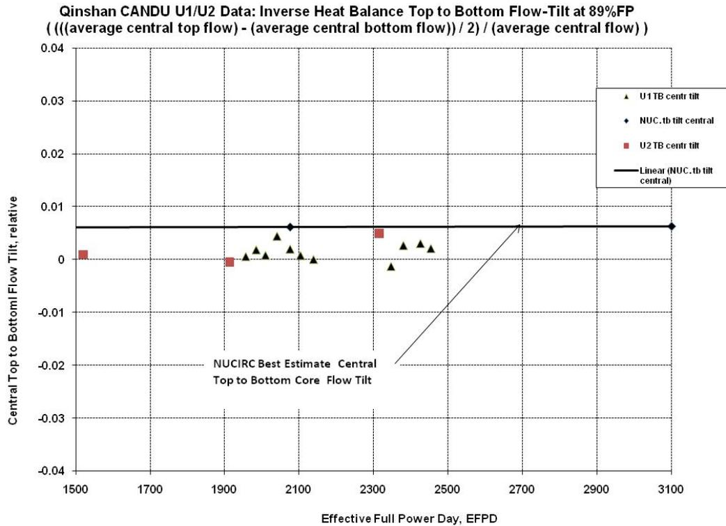
Figure 9 Central top to bottom flow tilt at 89% FP and model reference
