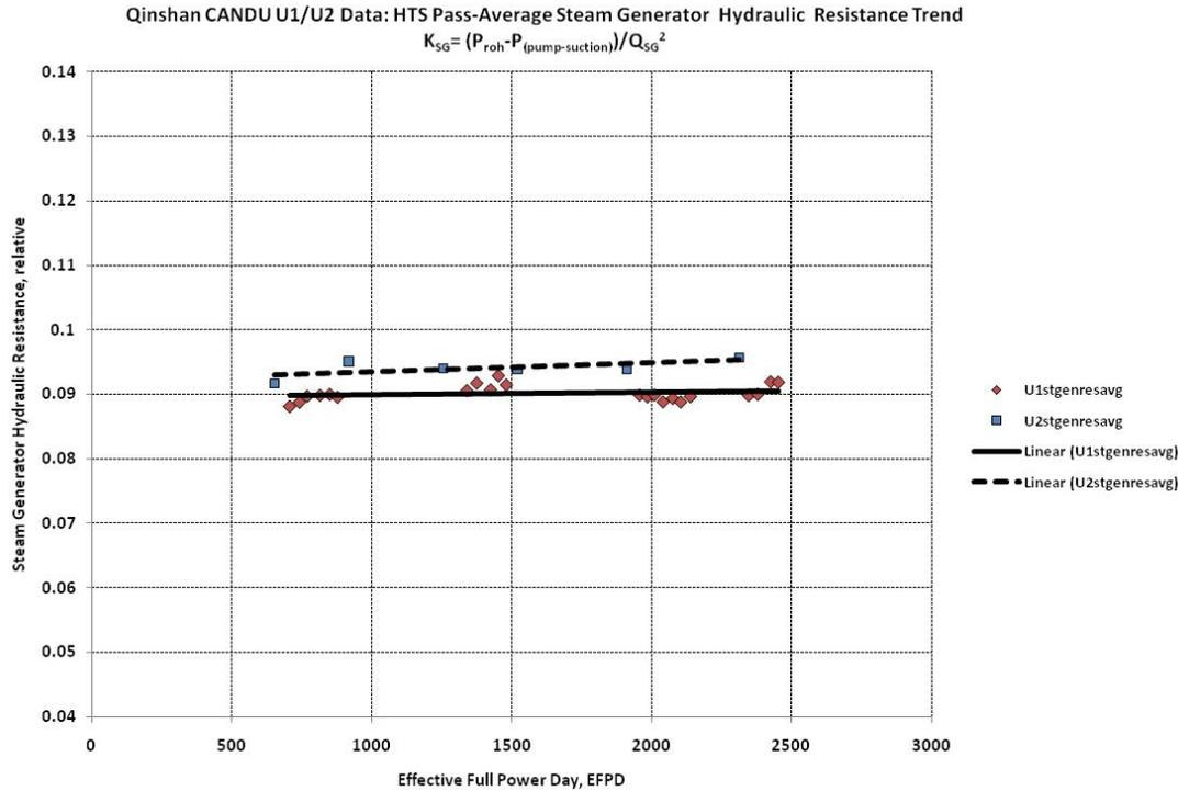
Figure 3 Steam generator hydraulic resistance
