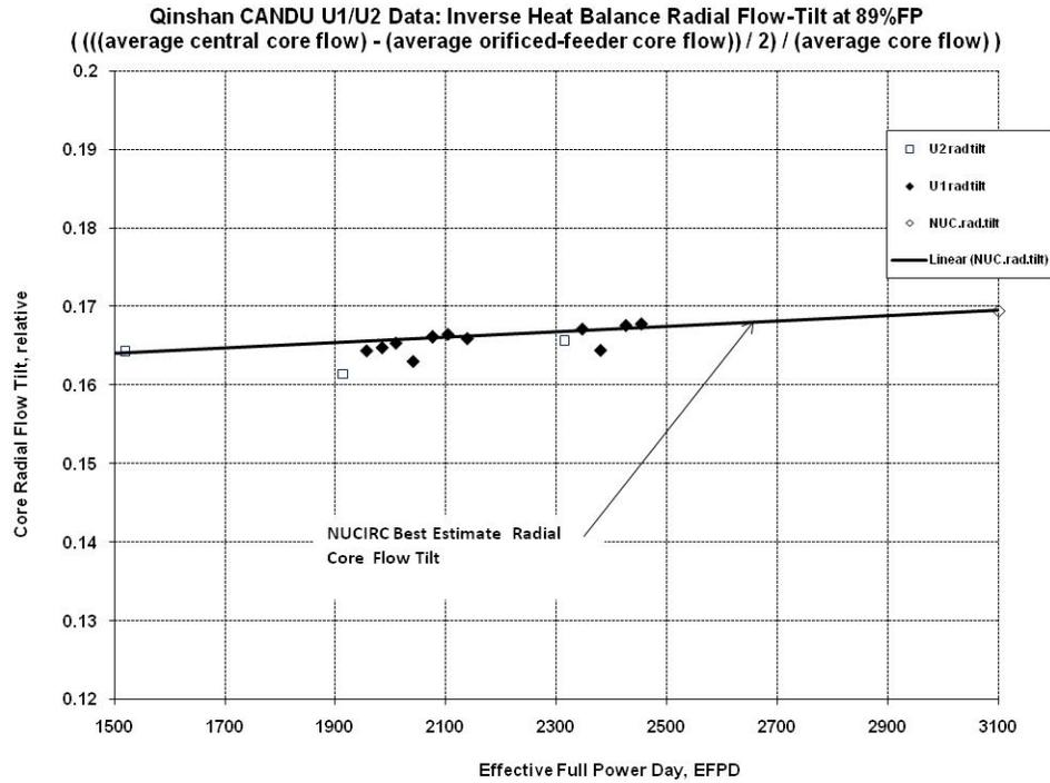
Figure 8 Core radial flow tilt at 89% FP and model reference
