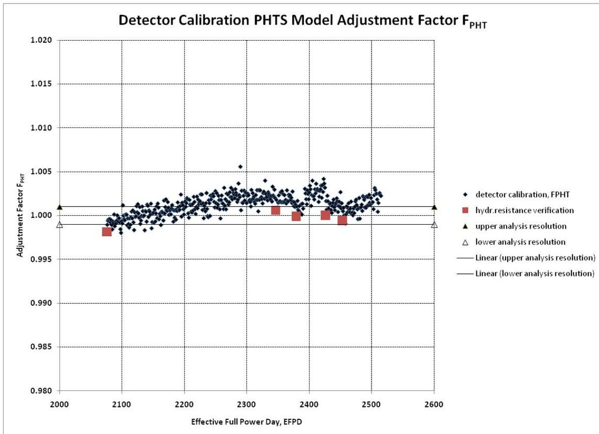
Figure 10  $F_{PHT}$  detector calibration adjustment between 2000 EFPD and 2600 EFPD
