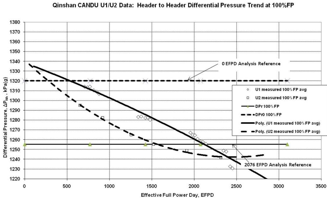
Figure 6 Header to header differential pressure and model references
