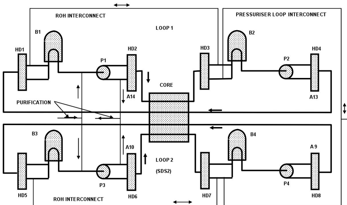
Figure 1 CANDU 6 simplified HTS flow diagram
