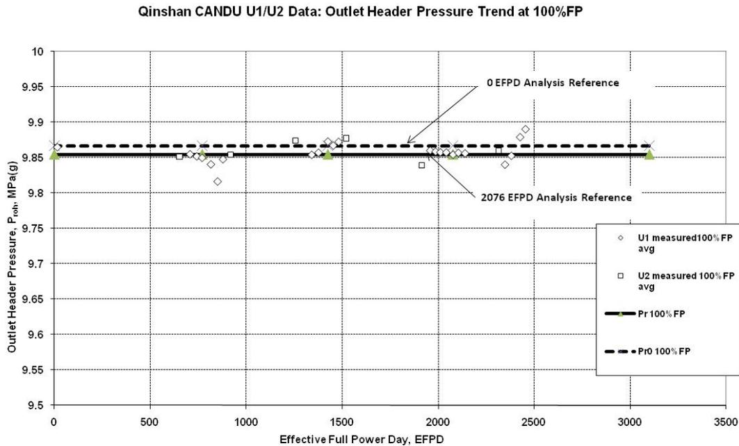
Figure 5 Outlet header pressure and model references
