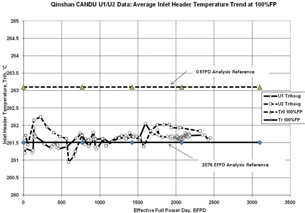
Figure 4 Inlet header temperature and model references
