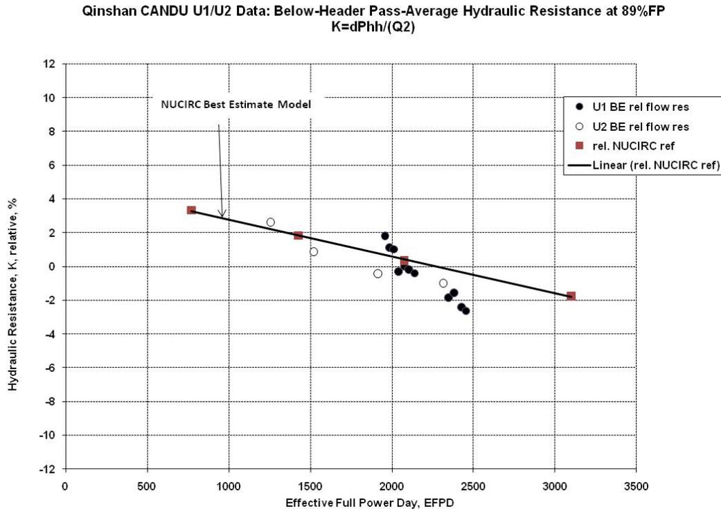
Figure 7 Reactor core hydraulic resistance at 89% FP and model reference
