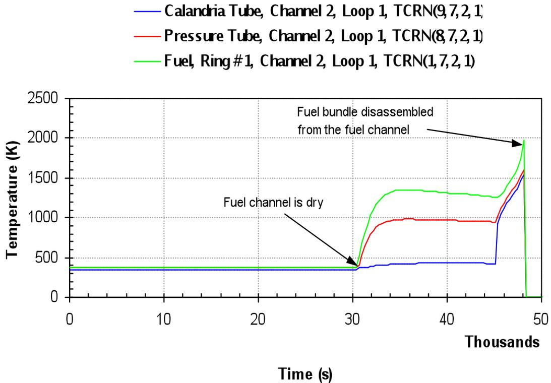
Figure 6 Fuel and Fuel Channel Temperatures: Bundle 7, Channel 2, Loop 1 (0 - 50,000 s)
