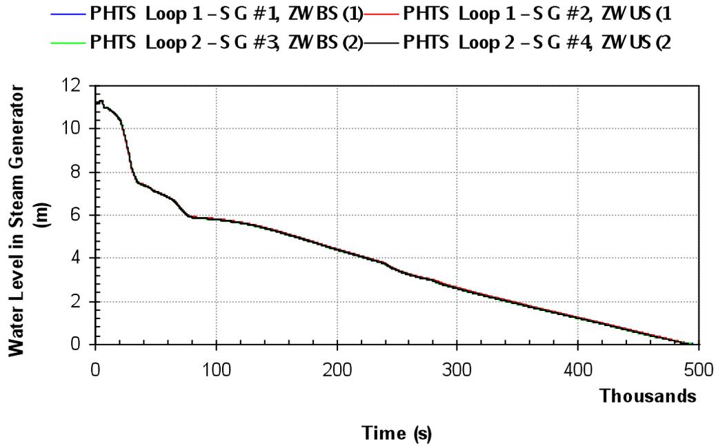
Figure 5 Steam Generator Water Level (0 - 500,000 s)
