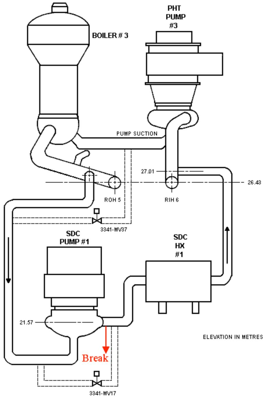
Figure 2 CANDU Shutdown Cooling System Elevations
