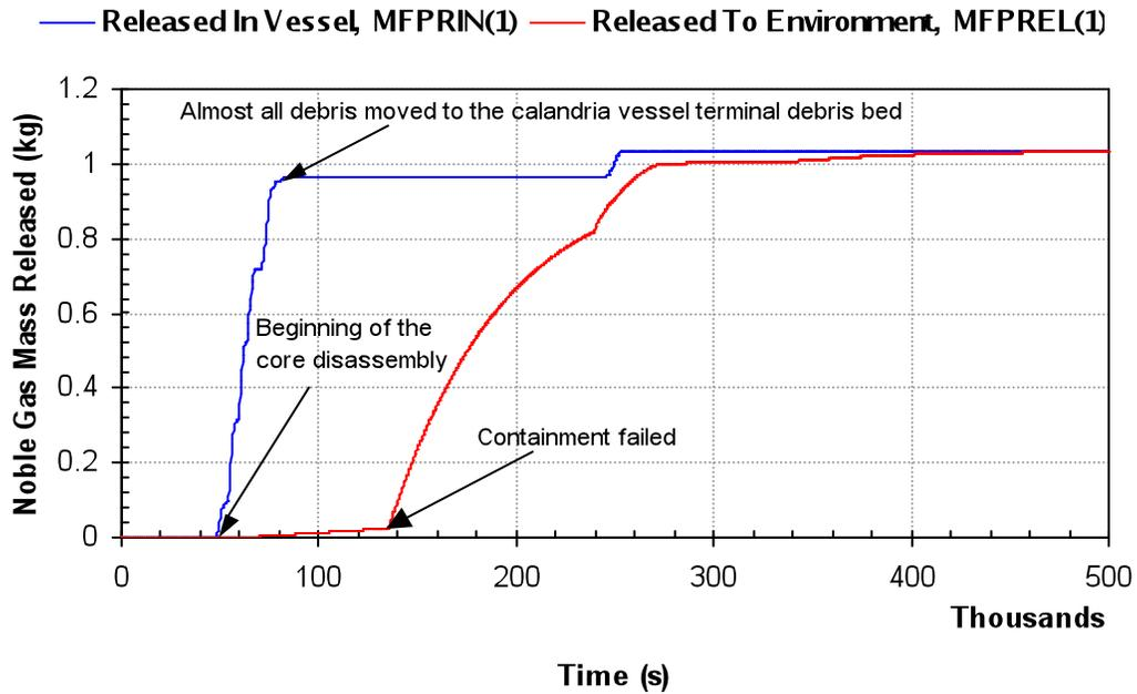
Figure 11 Mass of Noble Gases Released (0 - 500,000 s)
