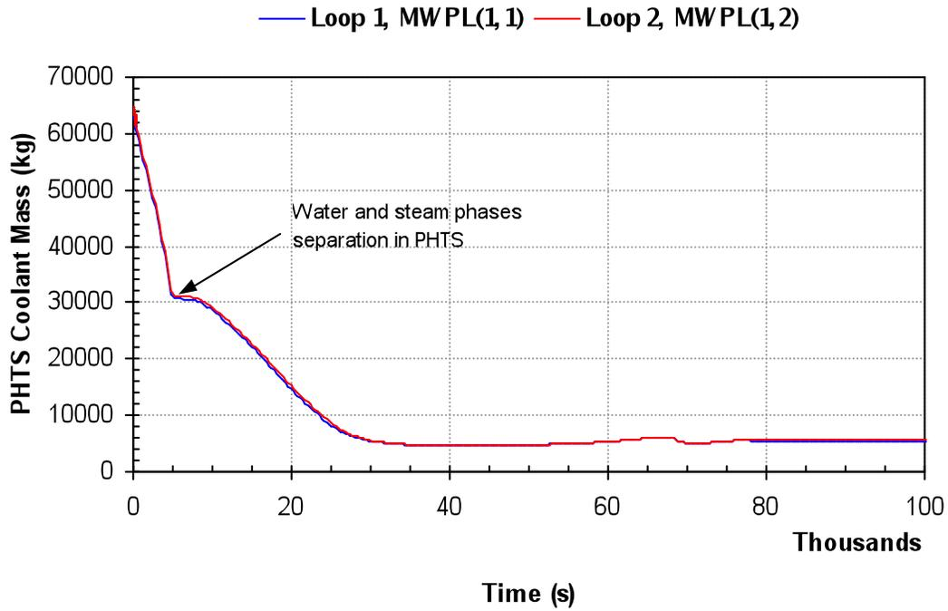
Figure 3 Primary System Water Masses in both Loops (0 - 100,000 s)
