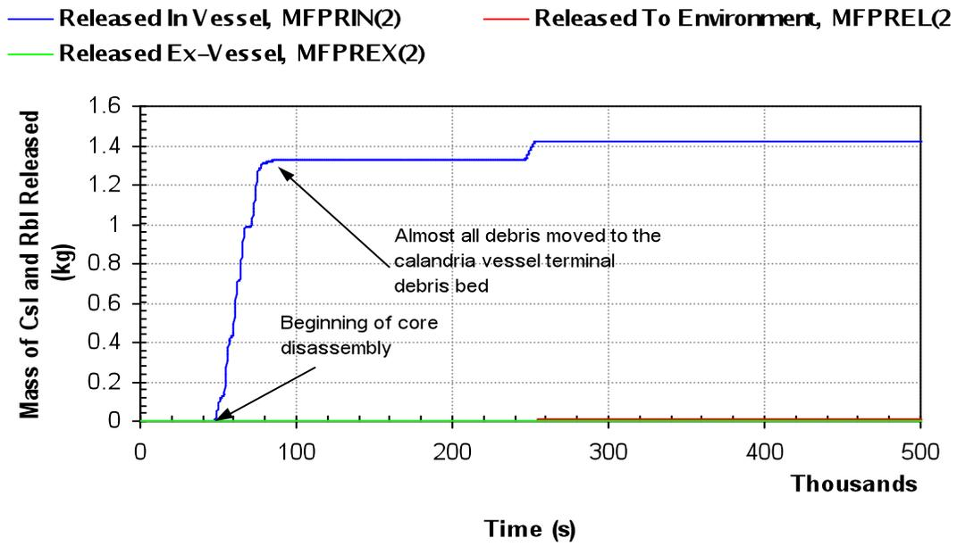
Figure 12 Mass and Location of Iodides Release (0 - 500,000 s)
