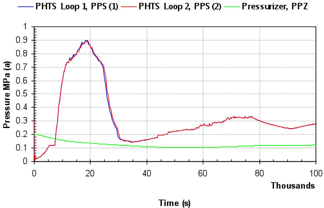
Figure 4 Primary System Pressure (0 - 100,000 s)
