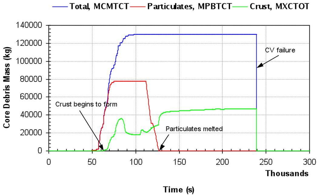
Figure 9 Mass of Corium (Crust, Particulates and Total) in the Calandria Vessel (0 - 300,000 s)
