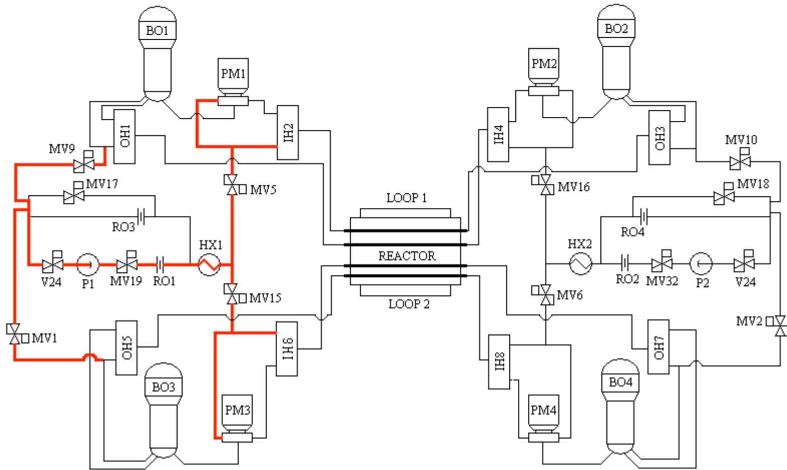
Figure 1 CANDU Shutdown Cooling System Connections (in Red)
