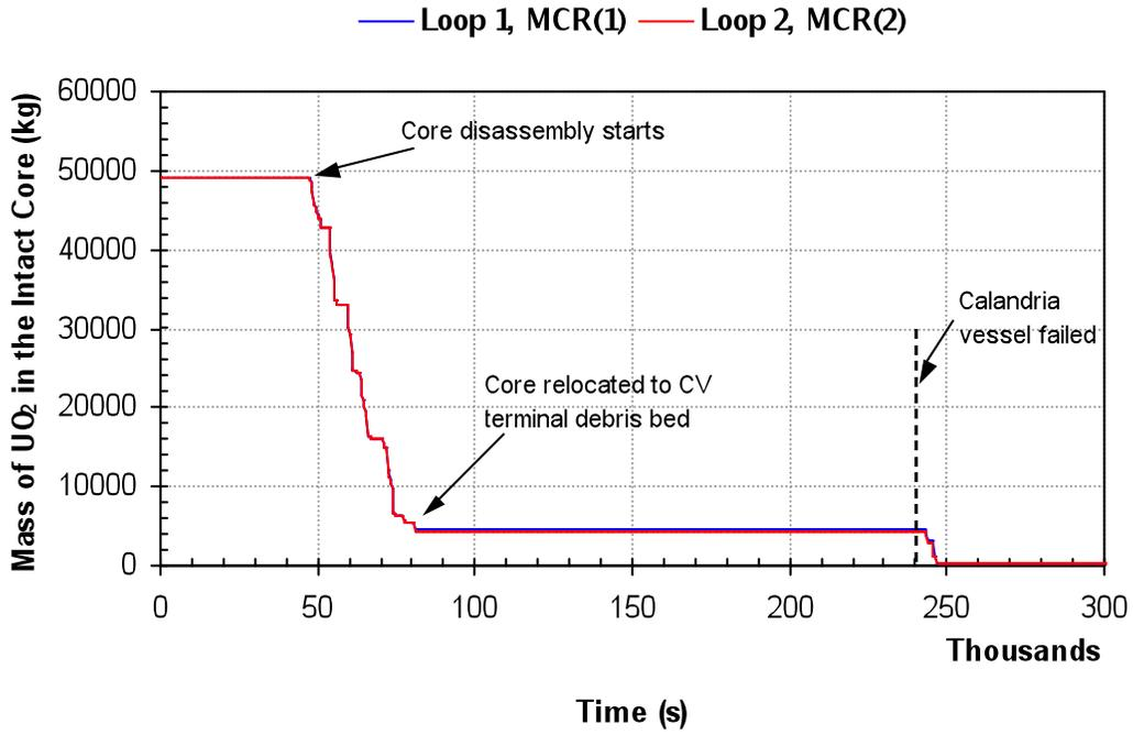
Figure 7  $UO_2$  Mass remaining in the Intact Fuel Channels (0 - 300,000 s)
