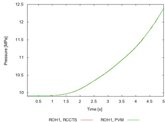
Figure 12 Reactor Outlet Header Pressure, CATHENA coupled to \*CERBERUS.
