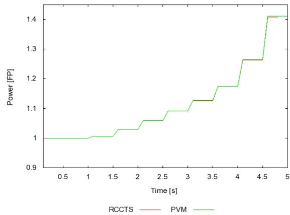
Figure 10 Bulk Reactor Power, CATHENA coupled to \*CERBRRS.
