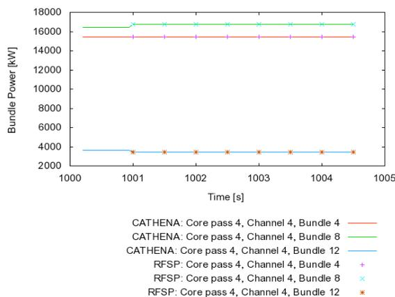
Figure 6 Testing Data Exchange: Bundle Powers in CATHENA and RFSP
