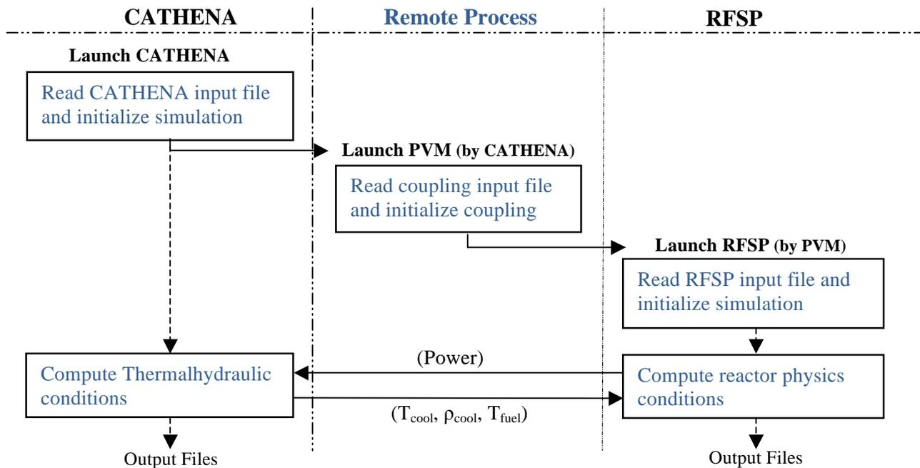
Figure 4 General PVM-based Coupling Calculation Scheme.
