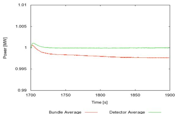
Figure 7 Steady-state: Total Reactor Power, CATHENA coupled to \*CERBRRS.
