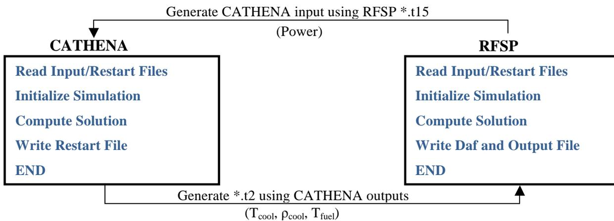
Figure 1 Script-based Coupling Calculation Scheme.
