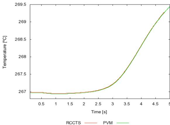
Figure 11 Reactor Inlet Header Temperature, CATHENA coupled to \*CERBERUS.
