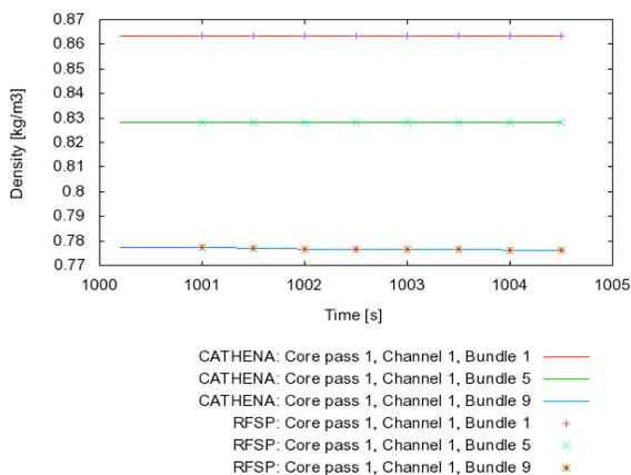
Figure 5 Testing Data Exchange: Coolant Densities in CATHENA and RFSP
