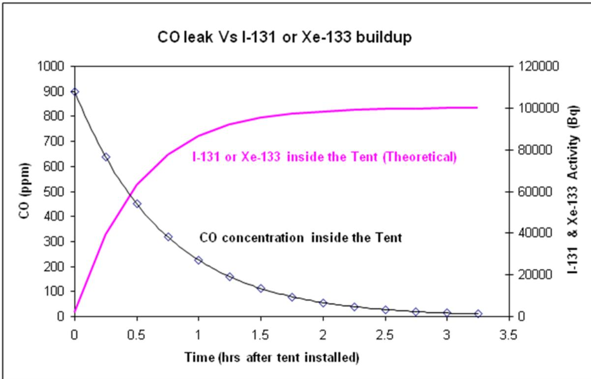
Figure 3 Theoretical diagram of CO leak Vs I-131 or Xe-133 buildup
