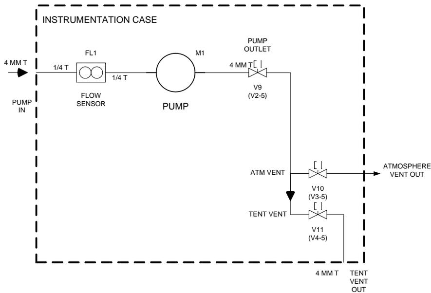
Figure 8 Instrumentation case process diagram
