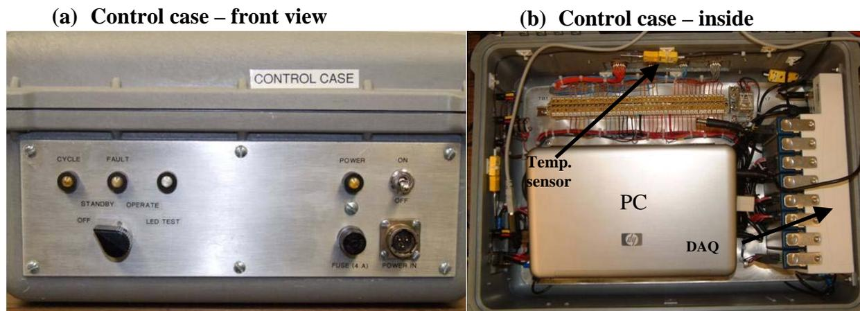
Figure 9 (a) Control case front view consists of operator console, accessed through the view port of the tent. (b) Control case consists of a PC, controller and 3 temperature sensors.
