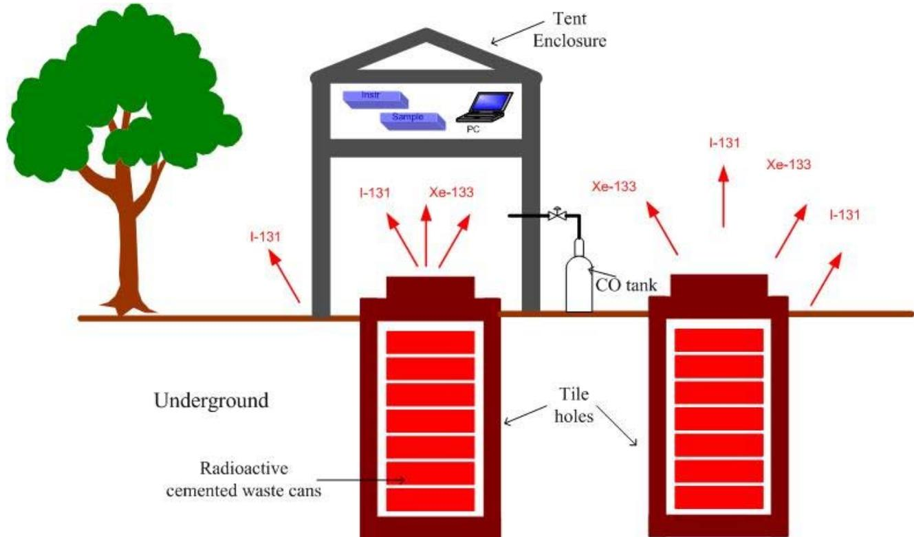
Figure 2 Schematic representation of I-131 and X-133 from tile holes, and the tent enclosure setup on a tile hole
