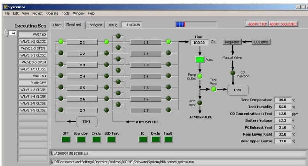
Figure 10 HMI (Human Machine Interface) screen shot showing the process controls and the sensor readings
