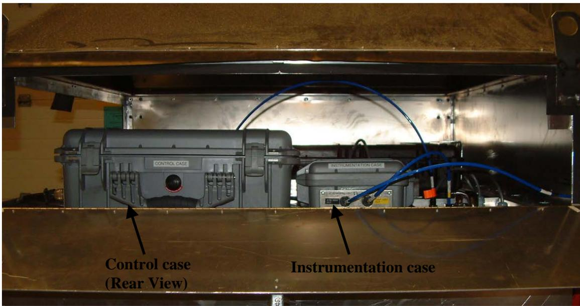
Figure 7 Instrumentation case and control case placed in instrumentation compartment
