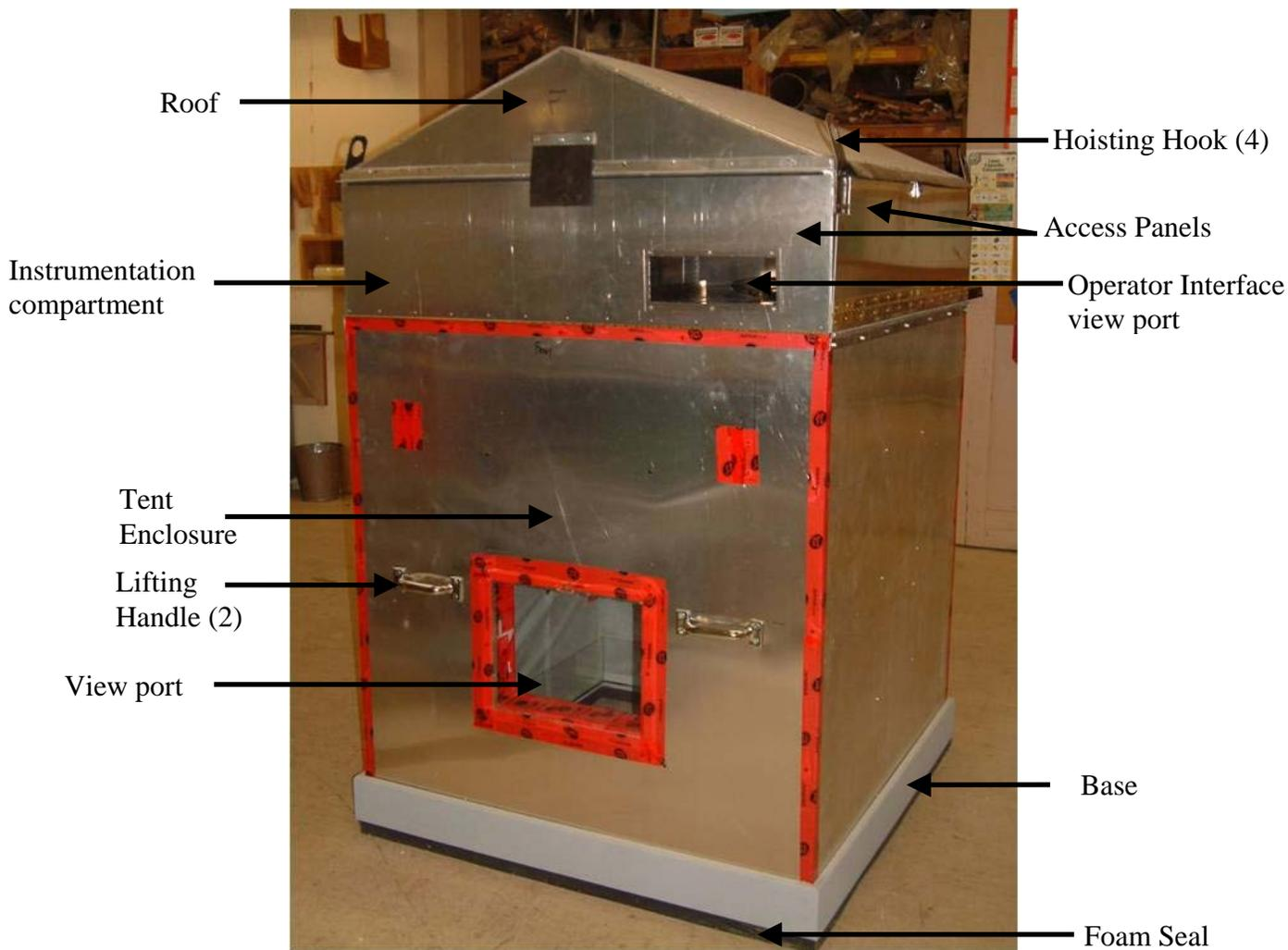
Figure 5 Tent Enclosure that placed on top of a tile hole or shipping flask to capture  $^{131}\text{I}$  and  $^{133}\text{X}$
