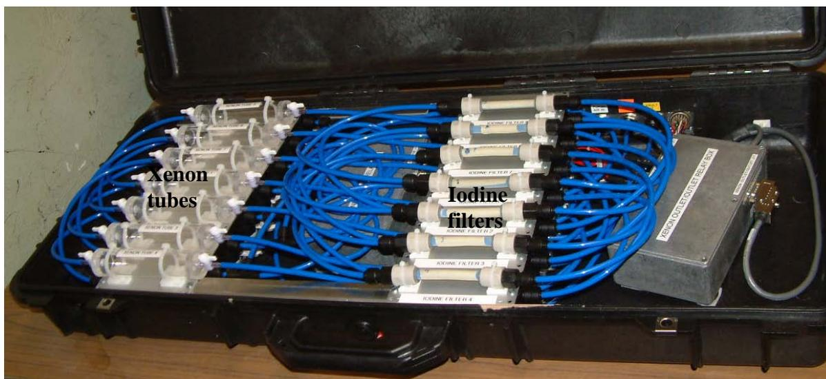
Figure 6 Sample Vault that contains 7 sets of iodine filters and xenon tubes
