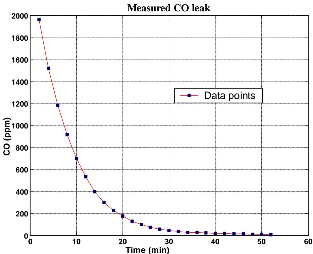
Figure 4 CO concentration in the tent measured by the system under development
