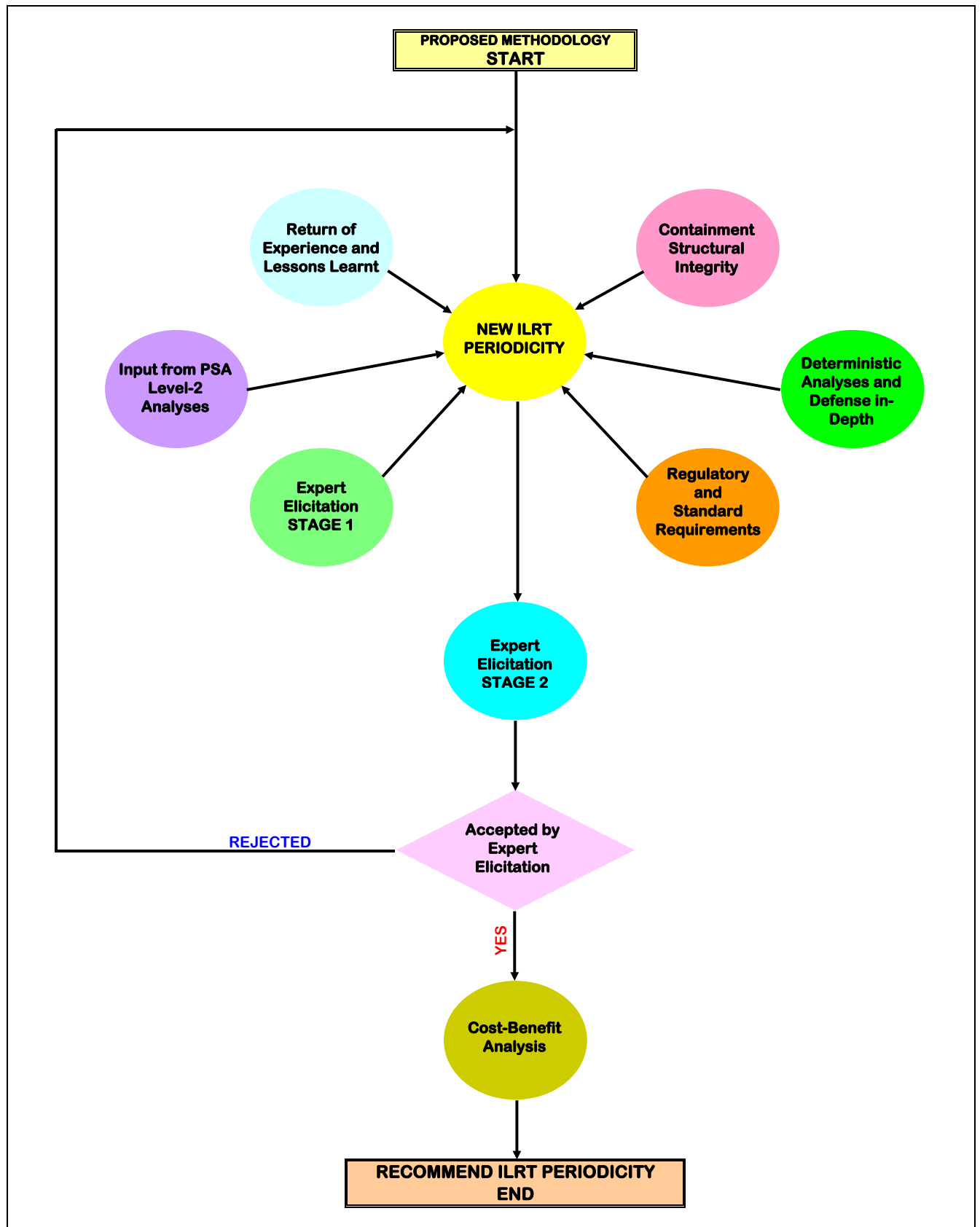
Figure 02: Flowchart of the Proposed ILRT Frequency Determination Methodology
