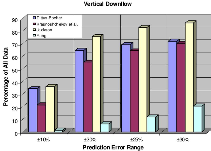
Figure 5 Percentage of All Vertical Downflow Data Predicted within Various Error Ranges
