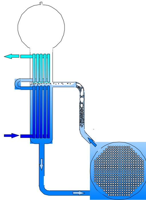
Figure 8 Schematic Diagram of the Passive Moderator Cooling System
