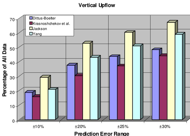
Figure 4 Percentage of All Vertical Upflow Data Predicted within Various Error Ranges
