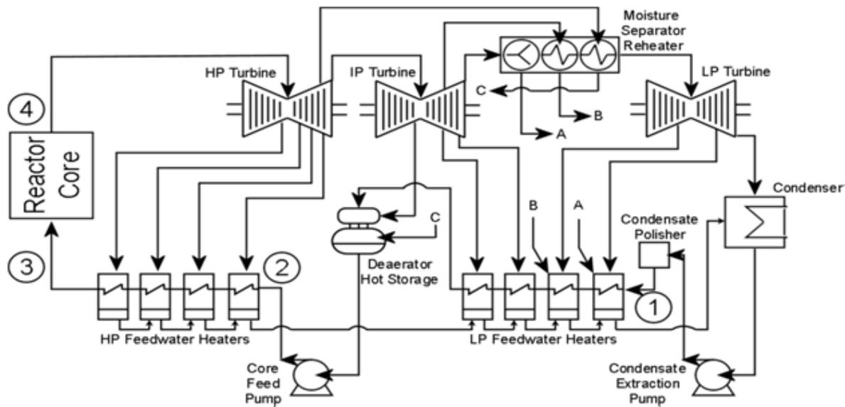
Figure 3 A hypothetical conceptual layout of an SCWR with indirect or steam reheat (for illustration purposes only). The four key locations for chemistry monitoring and control are noted.
