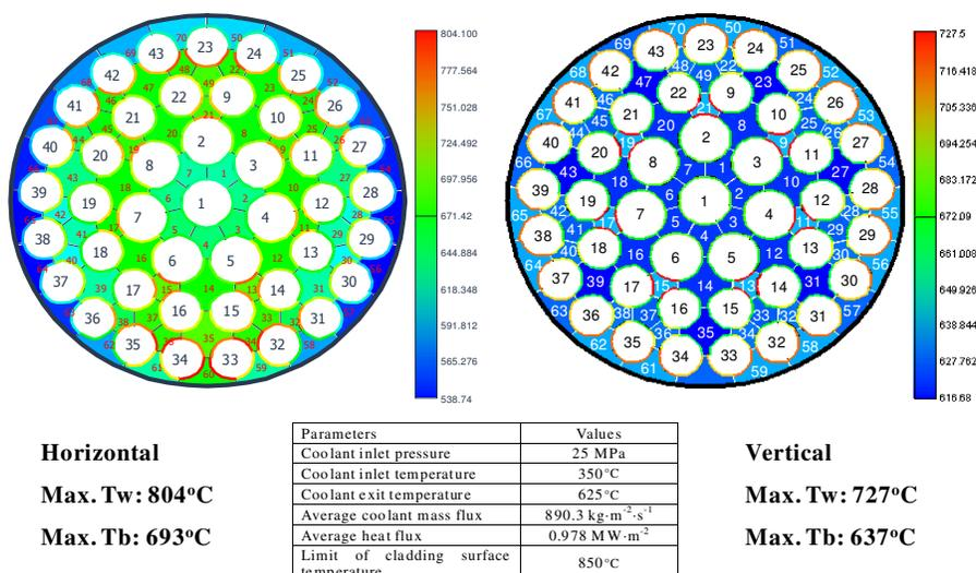
Figure 6 Cladding and Coolant Temperature Distributions in Subchannels of Reference (Uniform Enrichment) and Optimized (Graded Uranium) CANFLEX Bundles
