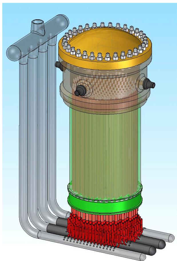
Figure 1 Schematic Diagram of One Design Concept of CANDU SCWR
