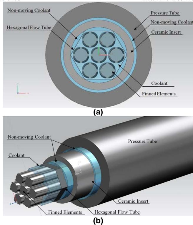
**Figure 3. Cross-section (a) and 3-D image (b) of the Dyadyakin and Popov test bundle installed inside pressure tube [3].**
