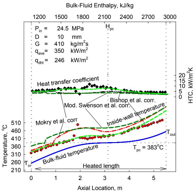
Figure 13: Temperature and HTC variations along vertical tube (5-m heated length and 10-mm ID):  $P_{in} = 24.5$  MPa,  $G = 410$  kg/m²s, and  $q_{avg} = 350$  kW/m² [15].
