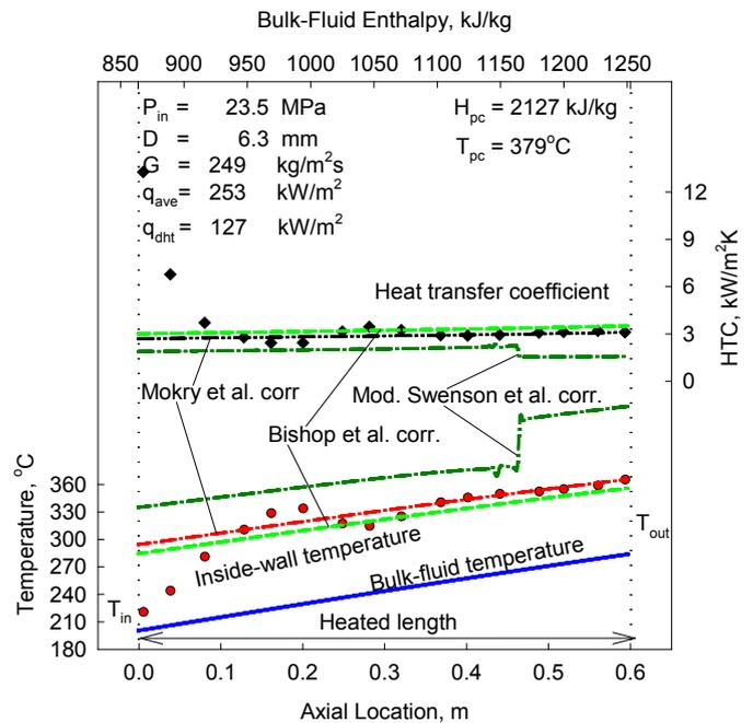
**Figure 8: Temperature and HTC variations along vertical tube (0.6-m heated length and 6.3-mm ID):  $P_{in} = 23.5$  MPa,  $G = 249$  kg/m²s, and  $q_{avg} = 253$  kW/m² [14].**
