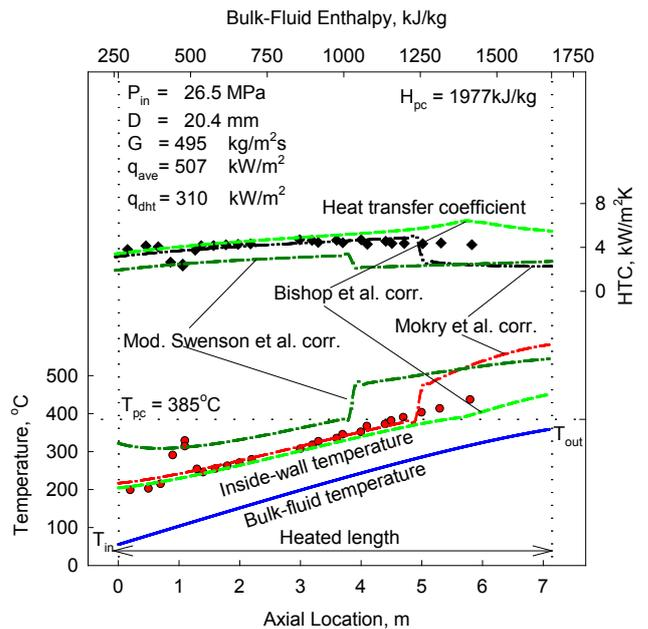
Figure 15: Temperature and HTC variations along vertical tube (7-m heated length and 20.4-mm ID):  $P_{in} = 26.5$  MPa,  $G = 495$  kg/m²s, and  $q_{avg} = 507$  kW/m² [16].
