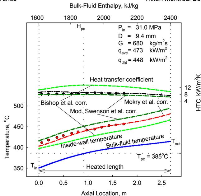
**Figure 20: Temperature and HTC variations along vertical tube (2.5-m heated length and 9.4-mm ID):  $P_{in} = 31$  MPa,  $G = 680$  kg/m<sup>2</sup>s, and  $q_{avg} = 473$  kW/m<sup>2</sup> [18].**
