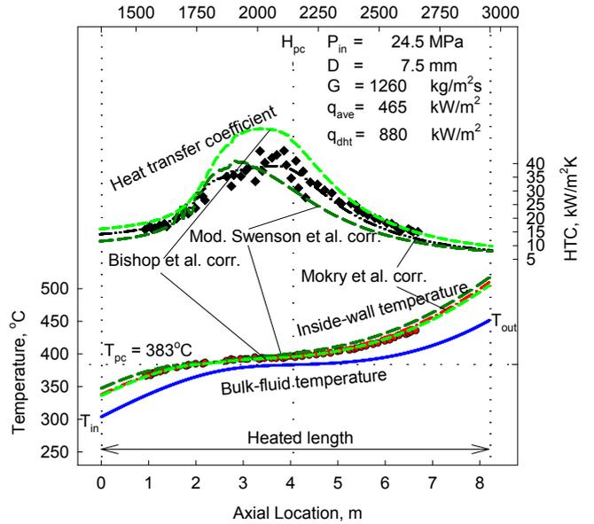
**Figure 18:** Temperature and HTC variations along vertical tube (8-m heated length and 7.5-mm ID):  $P_{in} = 24.5$  MPa,  $G = 1260$  kg/m<sup>2</sup>s, and  $q_{avg} = 465$  kW/m<sup>2</sup> [17].
