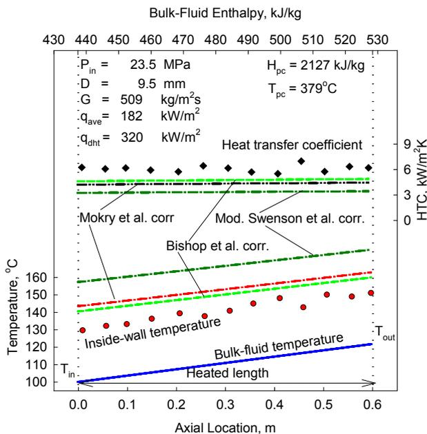
**Figure 10: Temperature and HTC variations along vertical tube (0.6-m heated length and 9.5-mm ID):  $P_{in} = 23.5$  MPa,  $G = 509$  kg/m<sup>2</sup>s, and  $q_{avg} = 182$  kW/m<sup>2</sup> [14].**
