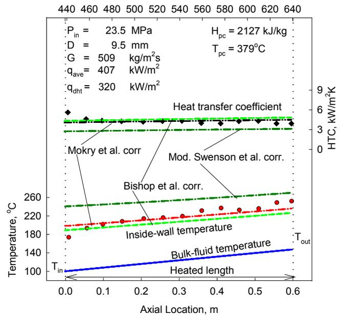
**Figure 11: Temperature and HTC variations along vertical tube (0.6-m heated length and 9.5-mm ID):  $P_{in} = 23.5$  MPa,  $G = 509$  kg/m<sup>2</sup>s, and  $q_{avg} = 407$  kW/m<sup>2</sup> [14].**
