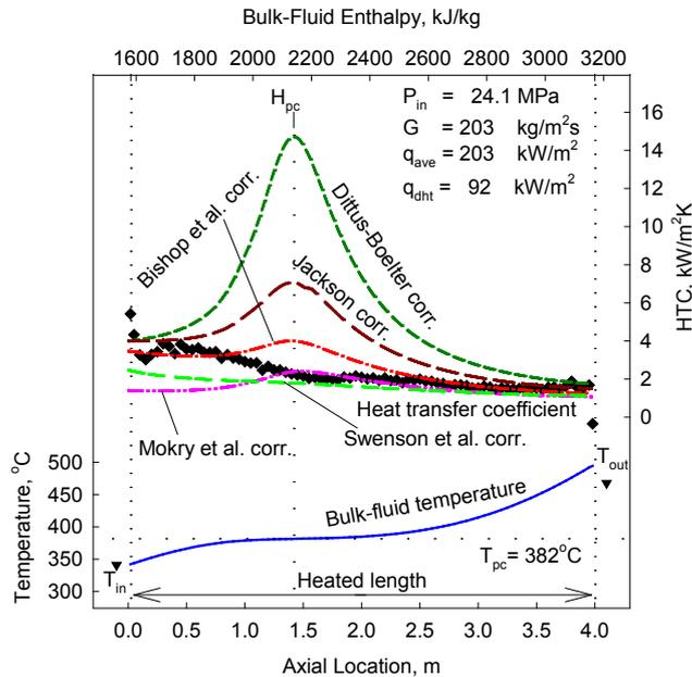
**Figure 1: Temperature and HTC variations along vertical tube (4-m heated length and 10-mm ID):**
