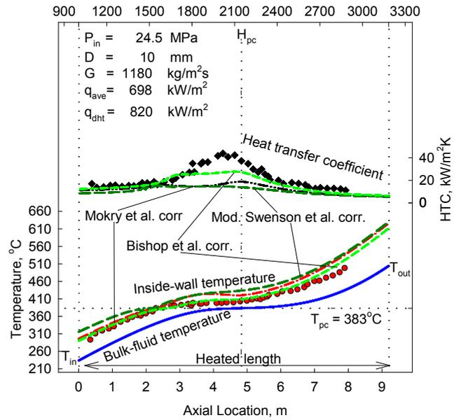
Figure 14: Temperature and HTC variations along vertical tube (9-m heated length and 10-mm ID):  $P_{in} = 24.5$  MPa,  $G = 1180$  kg/m²s, and  $q_{avg} = 698$  kW/m² [15].
