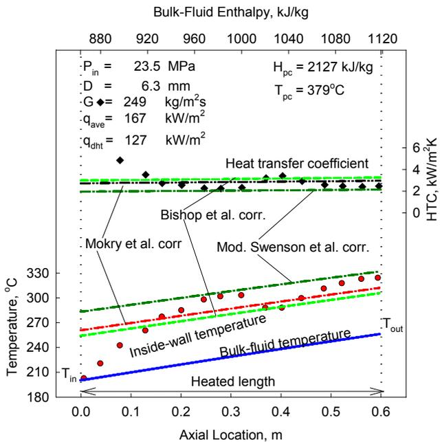
**Figure 6: Temperature and HTC variations along vertical tube (0.6-m heated length and 6.3-mm ID):  $P_{in} = 23.5$  MPa,  $G = 249$  kg/m²s, and  $q_{avg} = 167$  kW/m² [14].**
