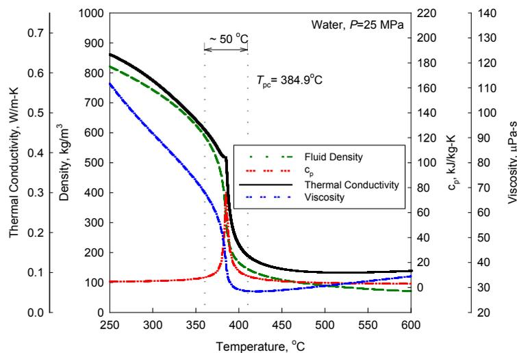
**Figure 2. Selected properties of supercritical water at pseudocritical point.**
