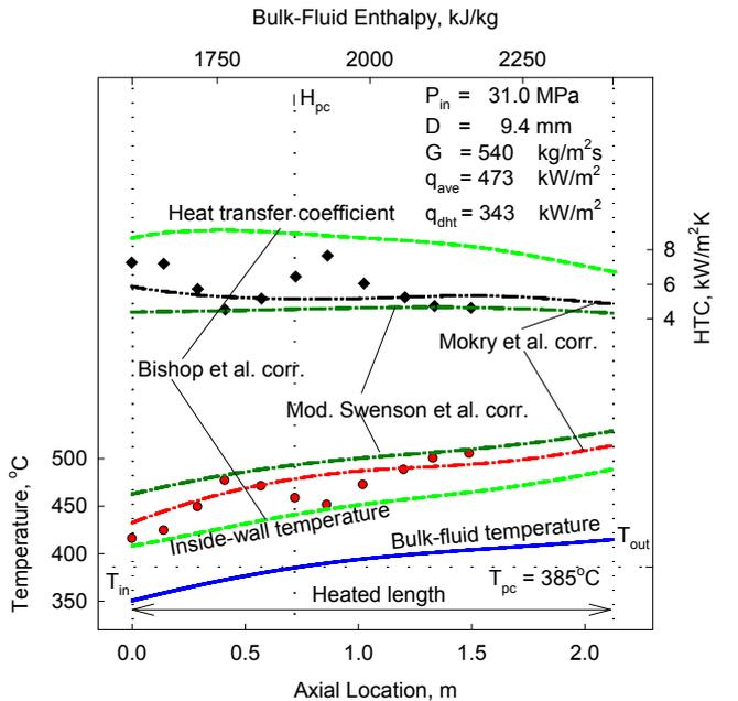
**Figure 19:** Temperature and HTC variations along vertical tube (2-m heated length and 9.4-mm ID):  $P_{in} = 31$  MPa,  $G = 540$  kg/m<sup>2</sup>s, and  $q_{avg} = 473$  kW/m<sup>2</sup> [18].
