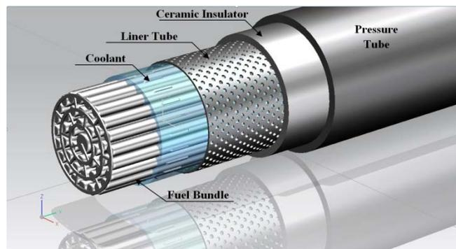
**Figure 4. 3-D image of SCW CANDU-reactor fuel channel with bundle inside.**
