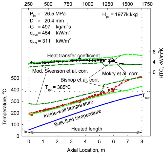
**Figure 16:** Temperature and HTC variations along vertical tube (8-m heated length and 20.4-mm ID):  $P_{in} = 26.5$  MPa,  $G = 497$  kg/m<sup>2</sup>s, and  $q_{avg} = 454$  kW/m<sup>2</sup> [16].
