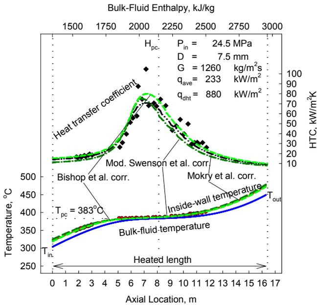
**Figure 17:** Temperature and HTC variations along vertical tube (16-m heated length and 7.5-mm ID):  $P_{in} = 24.5$  MPa,  $G = 1260$  kg/m<sup>2</sup>s, and  $q_{avg} = 233$  kW/m<sup>2</sup> [17].
