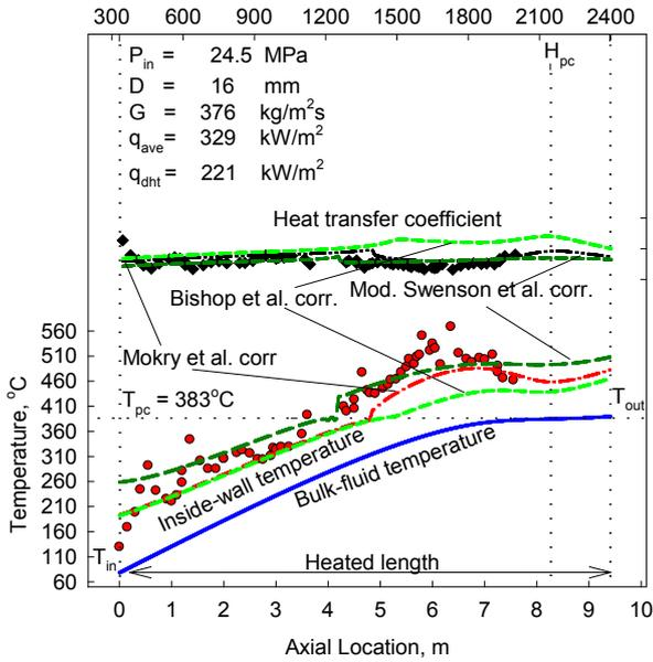
Figure 12: Temperature and HTC variations along vertical tube (9-m heated length and 16-mm ID):  $P_{in} = 24.5$  MPa,  $G = 376$  kg/m²s, and  $q_{avg} = 329$  kW/m² [15].
