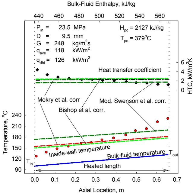
**Figure 5: Temperature and HTC variations along vertical tube (0.6-m heated length and 9.5-mm ID):  $P_{in} = 23.5$  MPa,  $G = 248$  kg/m²s, and  $q_{avg} = 118$  kW/m² [14].**
