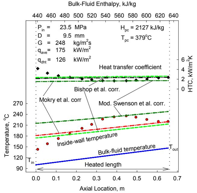
**Figure 7: Temperature and HTC variations along vertical tube (0.6-m heated length and 9.5-mm ID):  $P_{in} = 23.5$  MPa,  $G = 248$  kg/m²s, and  $q_{avg} = 175$  kW/m² [14].**
