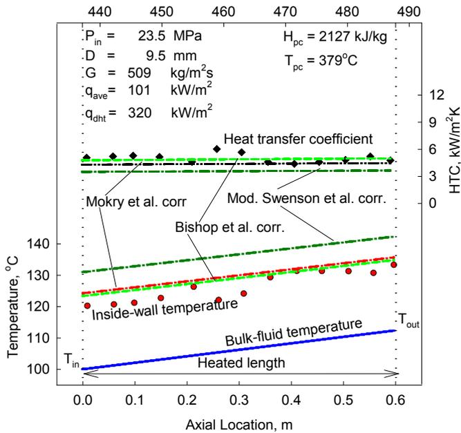
**Figure 9: Temperature and HTC variations along vertical tube (0.6-m heated length and 9.5-mm ID):  $P_{in} = 23.5$  MPa,  $G = 509$  kg/m<sup>2</sup>s, and  $q_{avg} = 101$  kW/m<sup>2</sup> [14].**
