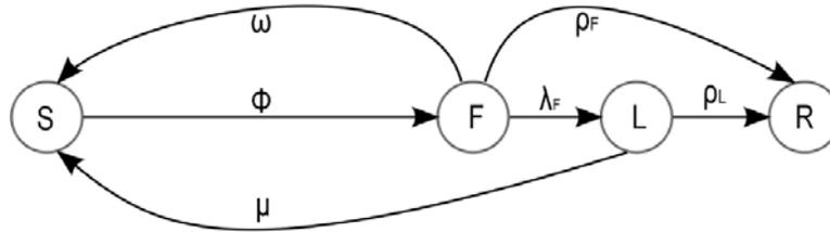
Figure 1. Four-state transition model for nuclear piping system degradation
