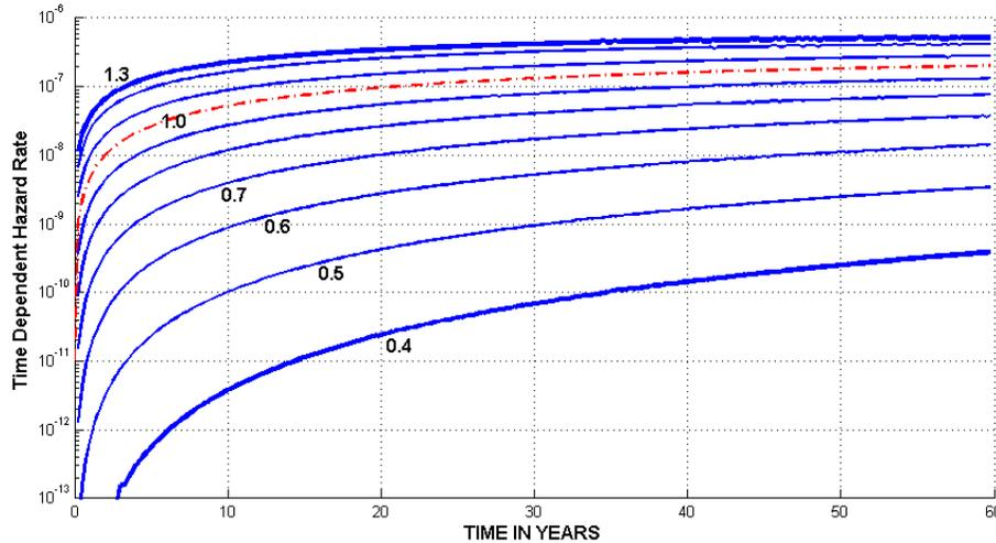
**Figure 5. Hazard rate of rupture with repair.**
