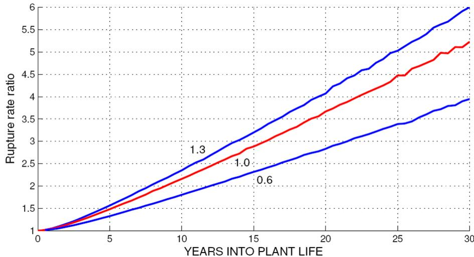
**Figure 7. Ratio of rupture rate without repair to rupture rate with repair**
