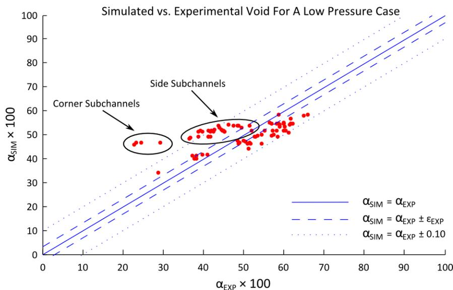
Figure 3 - Predicted vs. Measured Void Fraction for the Reference Case
