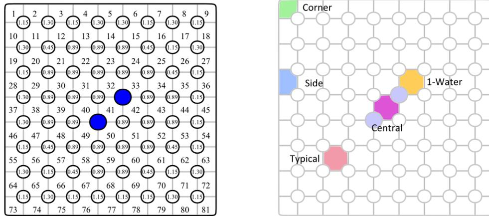
**Figure 1 - Bundle cross section with relative rod power and subchannel indices listed (left) and subchannel types of interest (right).**
