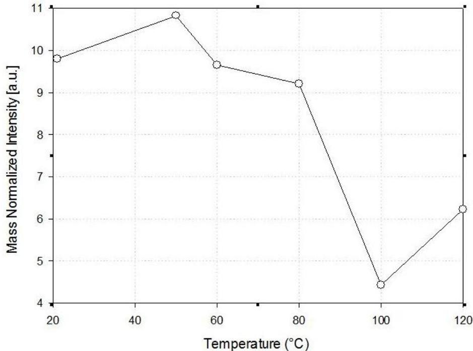
Isochronal heating curve using whole untreated drywall as background signal
