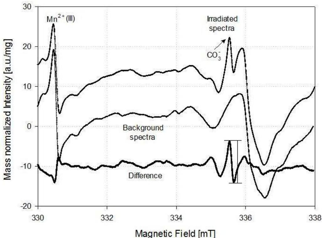
**Figure 1** Stacked EPR plot of irradiated ( $47.9 \pm 3.0$  Gy), unirradiated drywall and the difference. The EPR line of the radiation induced  $\text{CO}_3^-$  radical appears at a magnetic field of 335.54 mT. EPR scan parameters: 9 mW,  $334 \pm 4$  mT, 0.1 mT, 1x30 s, 0.1 s, 140 a.u.
