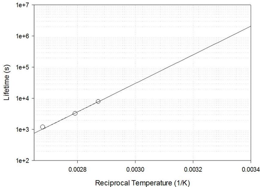
**Figure 5** Lifetime in seconds is plotted versus reciprocal temperature. For first-order (exponential) decay, a linear function should be observed. A linear fit was applied and extrapolated to room temperature ( $1/T=0.0034 \text{ K}^{-1}$ ).
