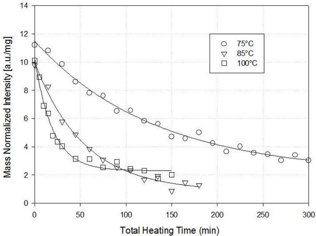
**Figure 3** The decay of intensities of the carbonate EPR line from heating temperatures of 75 °C, 85 °C and 100 °C. The most rapid decay is for the 100 °C heating temperature.
