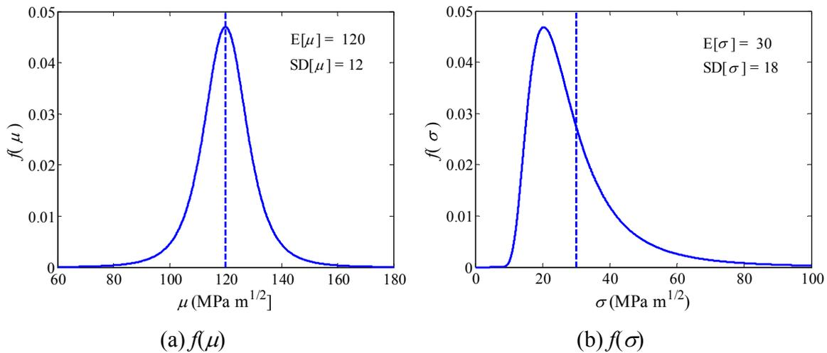
**Figure 3: Prior distributions of mean ( $\mu$ ) and standard deviation ( $\sigma$ ) of  $K_c$**
