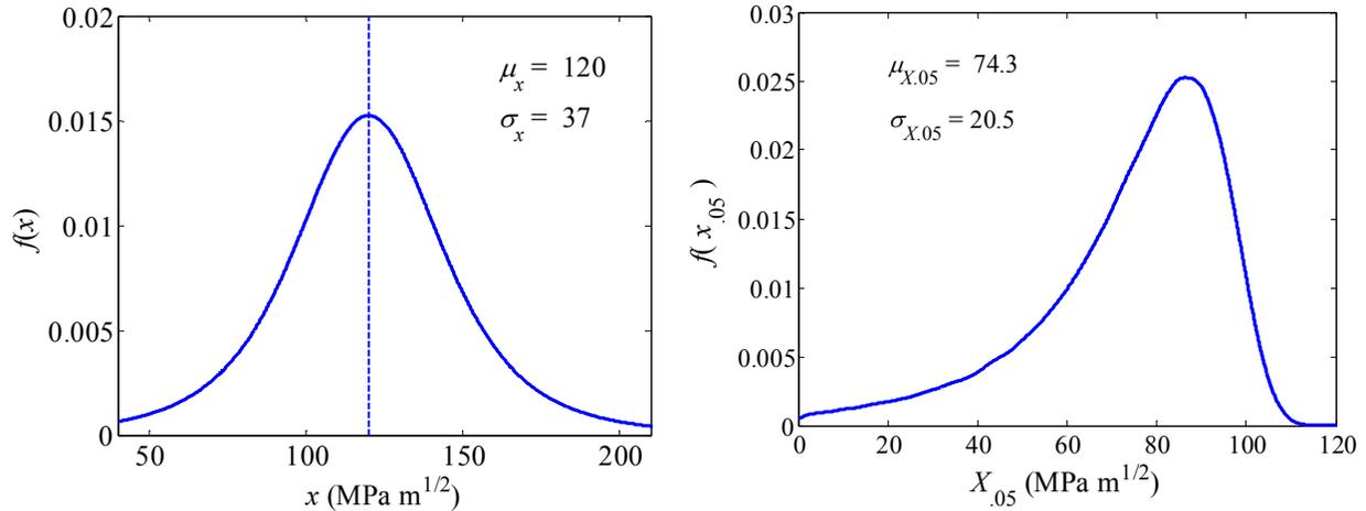
**Figure 4: Prior distributions of (a)  $K_c$  and (b) 5% percentile of  $K_c$**
