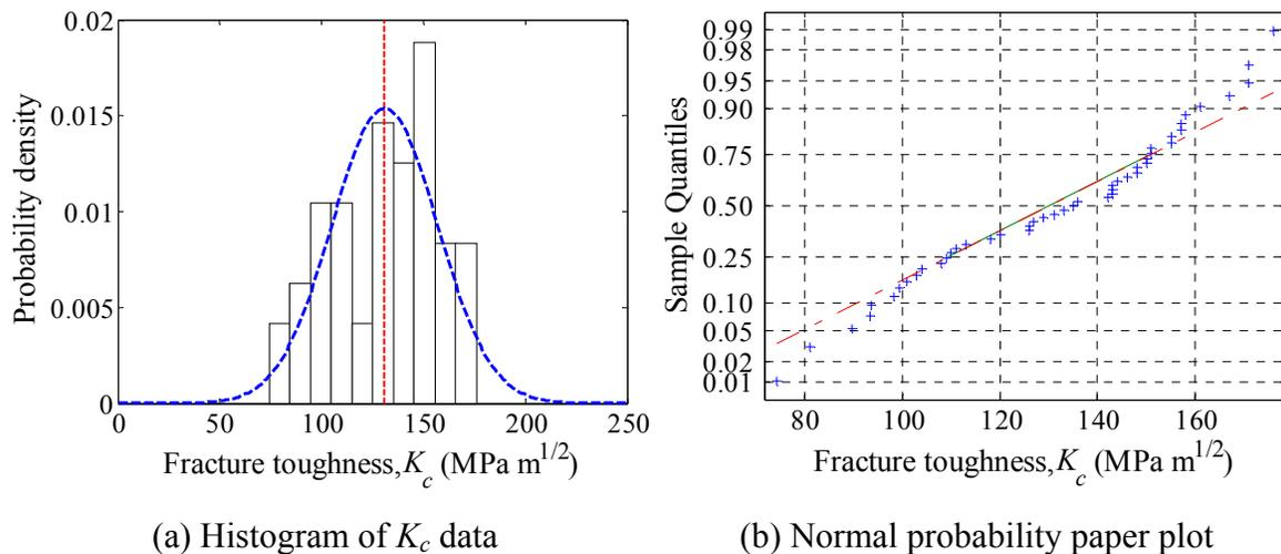
**Figure 2: Illustration of a sample of fracture toughness data**
