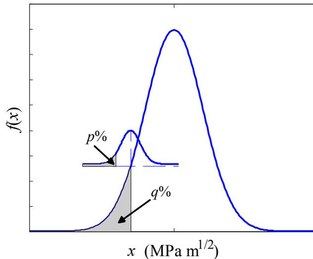
Figure 1: Proposed definition of the probabilistic lower bound of fracture toughness
