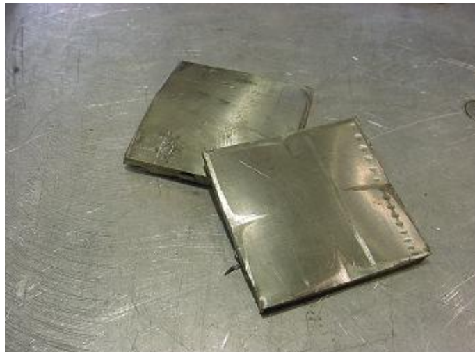
Figure 8 Two Pressure Tube Coupons Processed by the Volume Reduction Press
