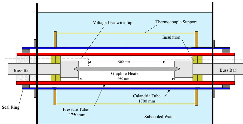
**Figure 2 Schematic of Apparatus Used for Q-Series Contact Boiling Test (not to scale)**
