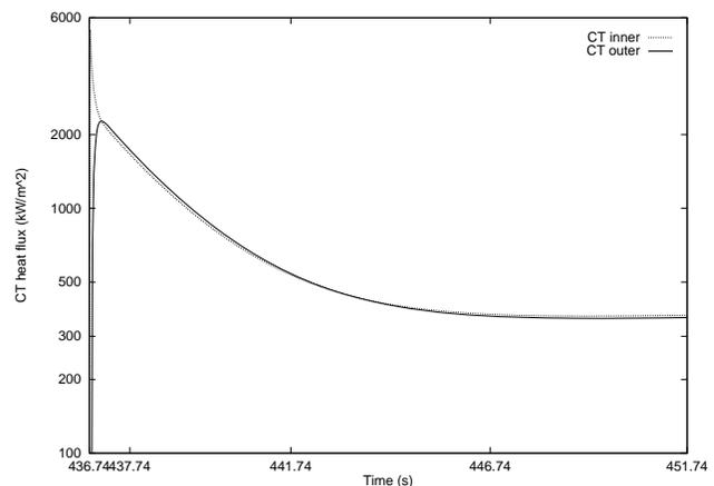
**Figure 5 Calculated Heat Flux on CT Inner and Outer Surfaces in a Typical Q-series Test**
