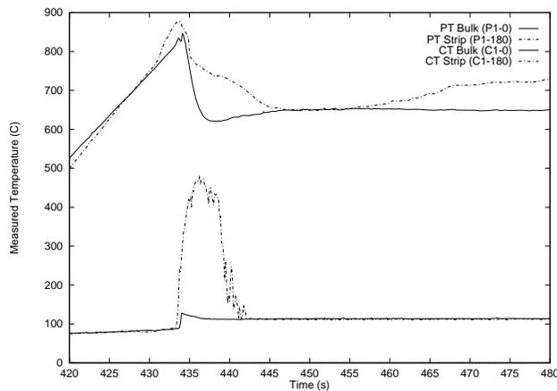
**Figure 4 PT and CT Temperature Measurement in a Typical Q-series Test**
