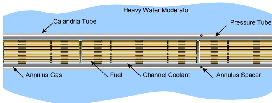
**Figure 1 Schematic Diagram of the CANDU Fuel Channel**
