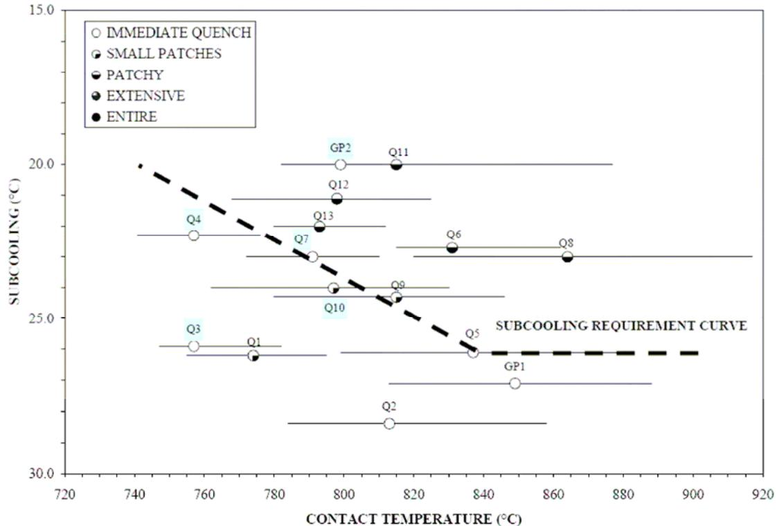
**Figure 6 Moderator Subcooling Requirement Curve Using Glass-Peened Calandria Tubes**
