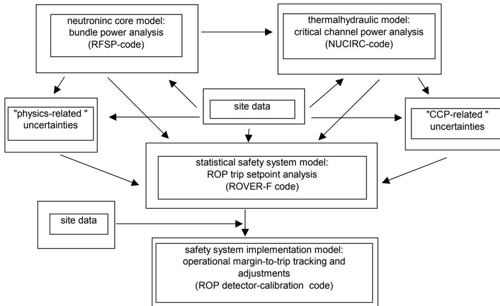
Figure 2 Simplified ROP Analysis Interfaces
