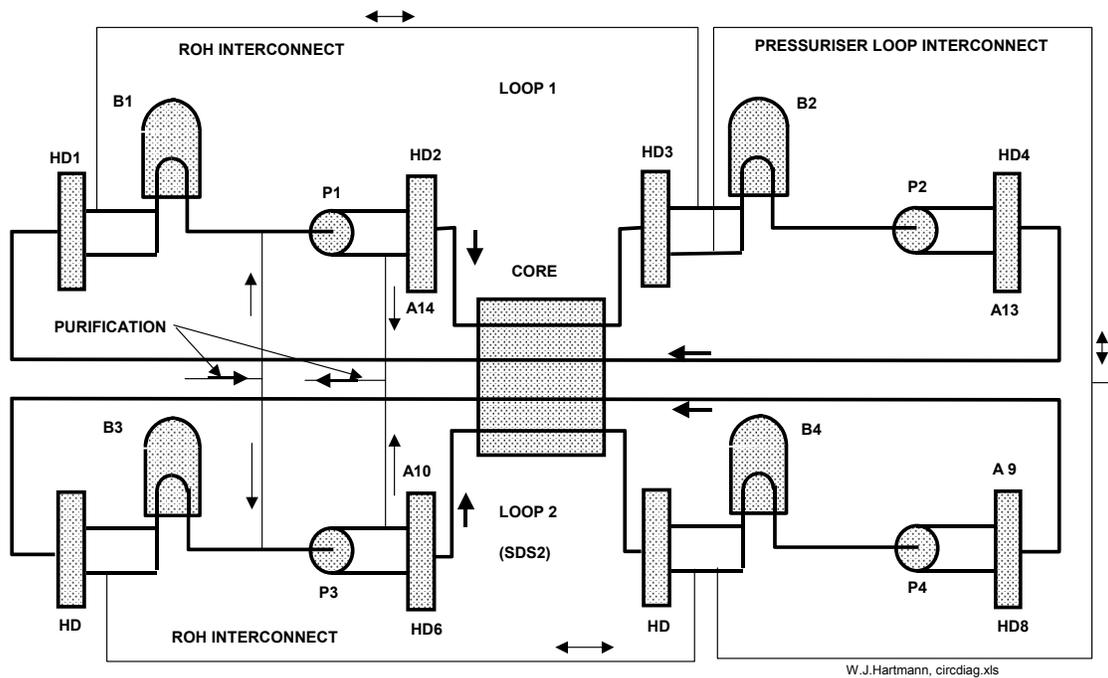
Figure 1 Typical CANDU 6 Simplified HTS Flow Diagram
