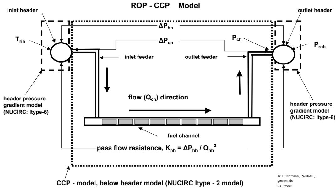
Figure 3 Simplified ROP-CCP Below-Header Hydraulic Model
