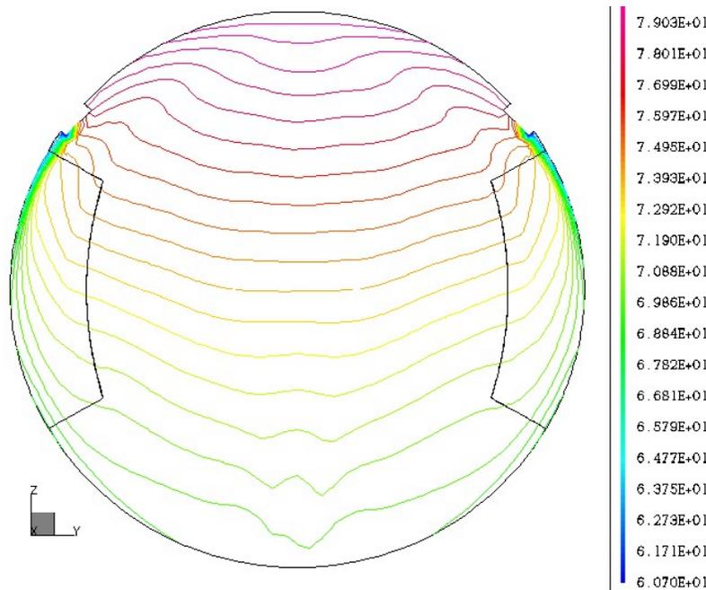
Figure 5 Temperature (°C) Isotherms in x=1.08 m Plane (Inlet Nozzle), for Case 1
