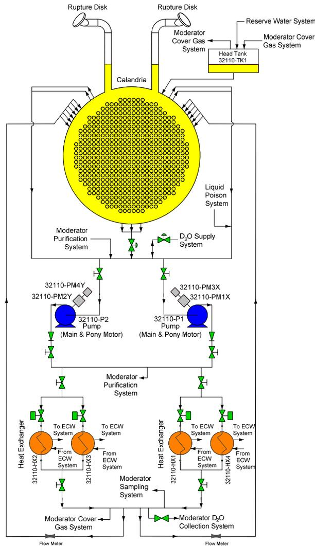
Figure 1 ACR-1000 Moderator System Flow Diagram
