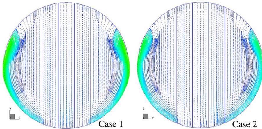
Figure 6 Velocity Fields in  $X = 2.97\text{m}$  Middle Planes, for Case 1 & 2
