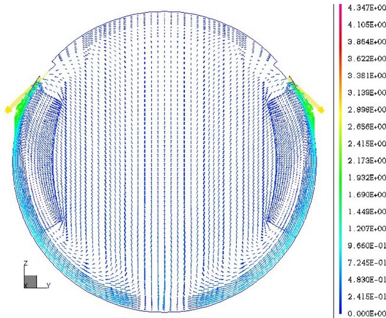
Figure 4 Velocity Field (m/s) in x=1.08 m Plane (Inlet Nozzle Plan), for Case 1
