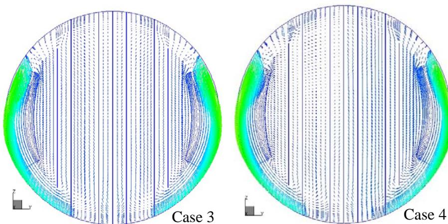
Figure 8 Velocity Fields in  $X = 2.97\text{m}$  Middle Planes, for Case 3 & 4
