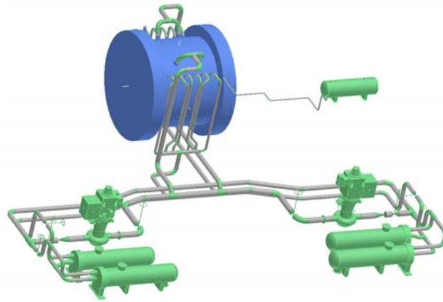
Figure 2 Moderator System Configuration
