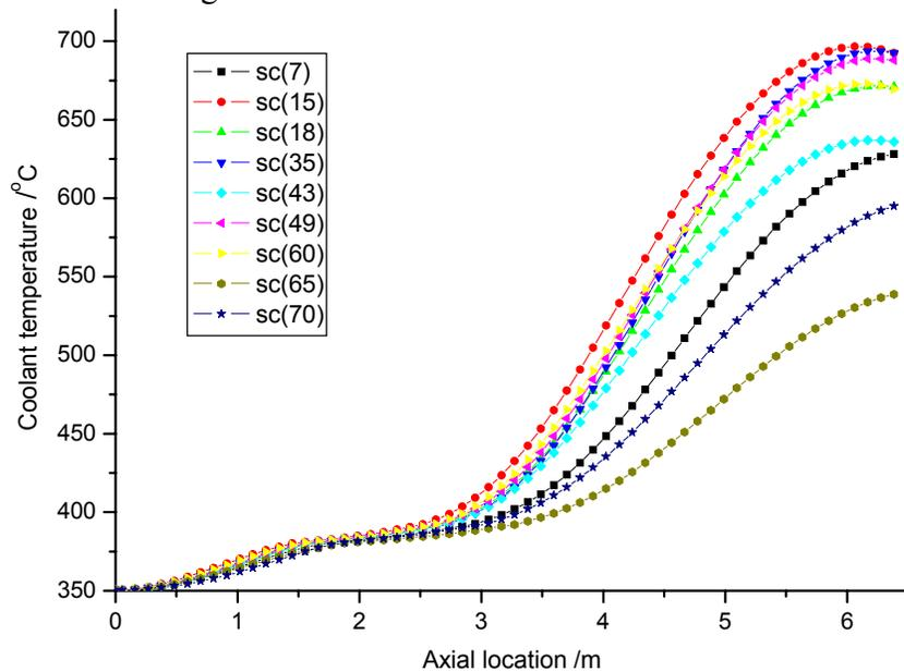
Figure 5 Subchannel Coolant Temperature Distribution Along Axial Nodes.
