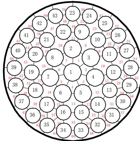
Figure 2 Subchannel Identification in a CANFLEX fuel bundle.
