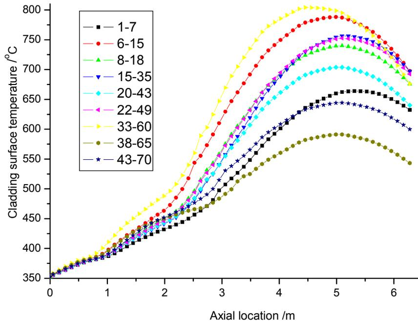
Figure 6 Cladding Surface Temperature of Typical Locations along Axial Nodes (1-7 denotes the fragment of rod 1 that facing subchannel 7)
