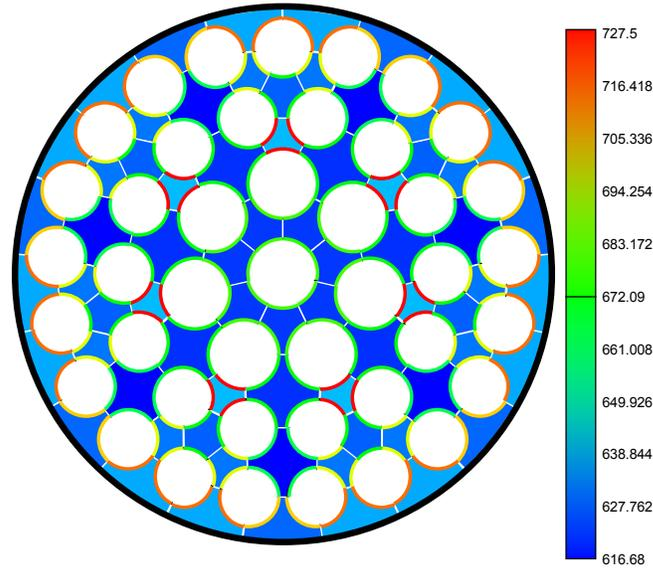
Figure 7 Distributions of Maximum Cladding Surface Temperatures and Outlet Coolant temperature after optimization
