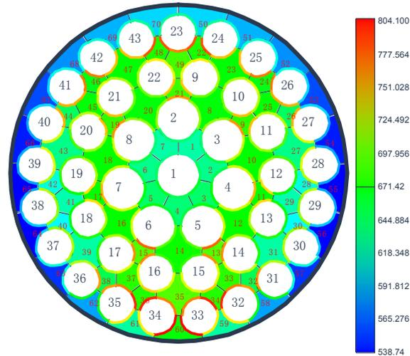
Figure 3 Distributions of Maximum Cladding Surface Temperatures and Outlet Coolant temperature.
