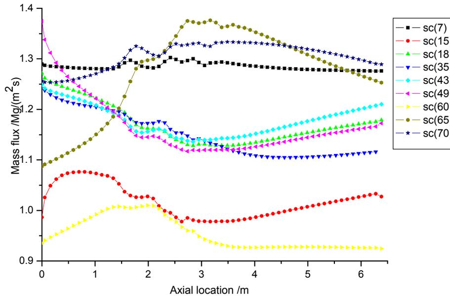
Figure 4 Subchannel Coolant Mass Flux Distribution along Axial Nodes.
