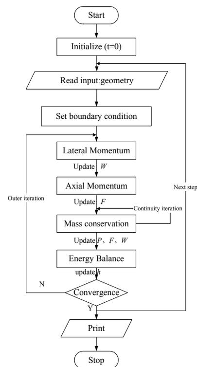
Figure 1 Evaluation Scheme of ATHAS Subchannel Code.
