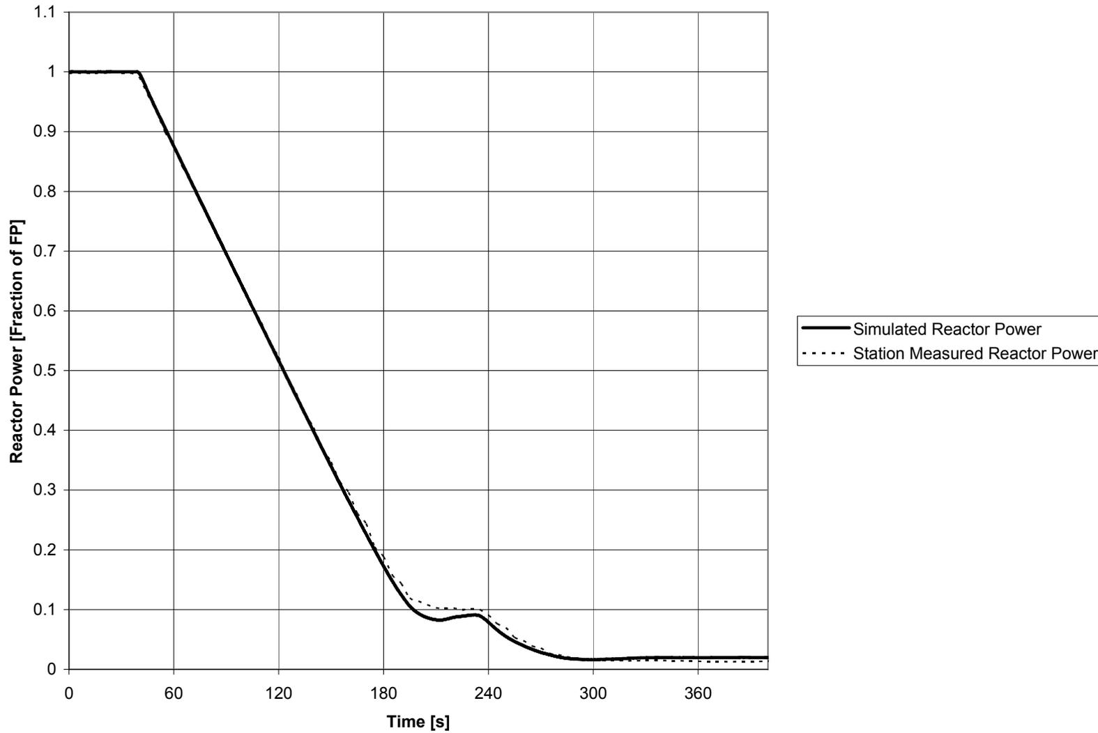
**Figure 3 – Comparison between Simulated Reactor Neutronic Power and PNGSB Unit 5 Measured Reactor Neutronic Power**
