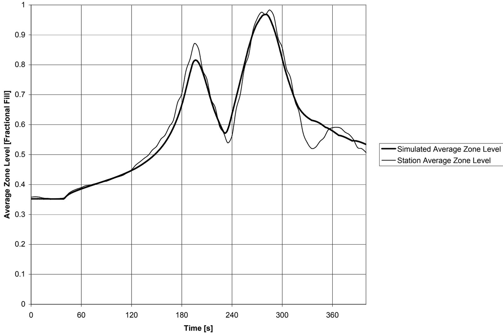
**Figure 5 – Comparison between Simulated Average Zone Level and PNGSB Unit 5 Measured Average Zone Level**
