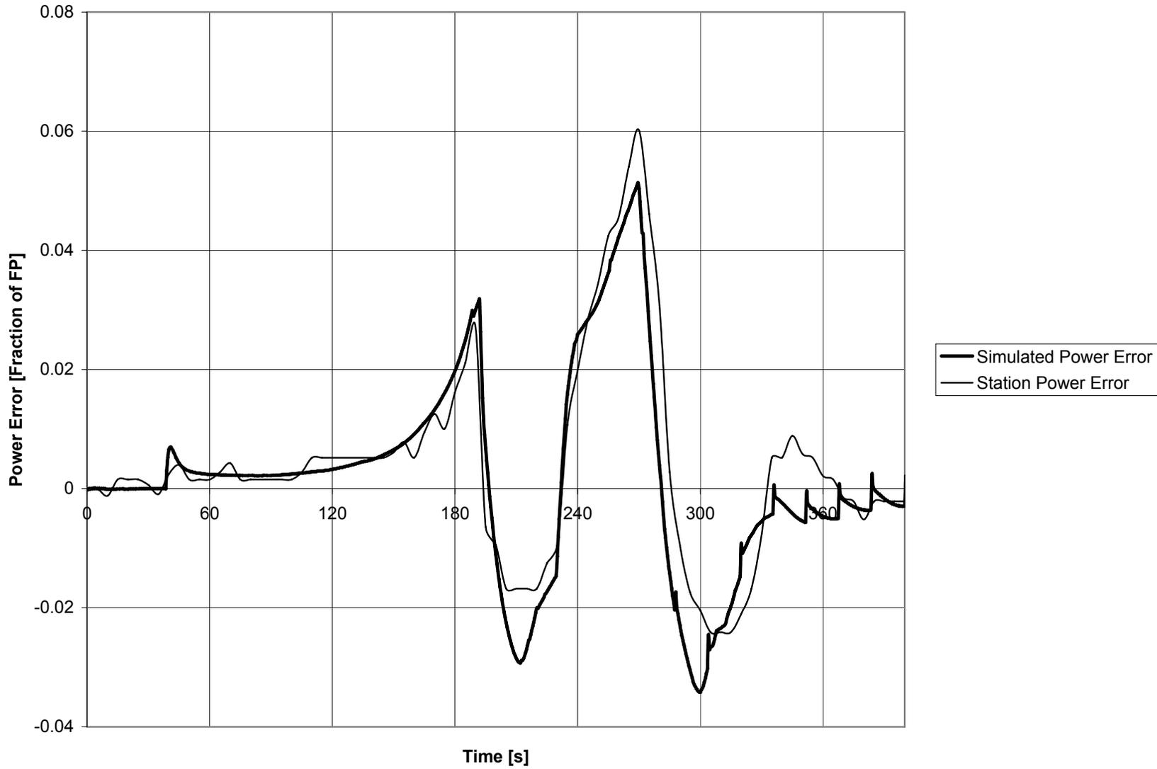
**Figure 4 – Comparison between Simulated Power Error and PNGSB Unit 5 Measured Power Error**
