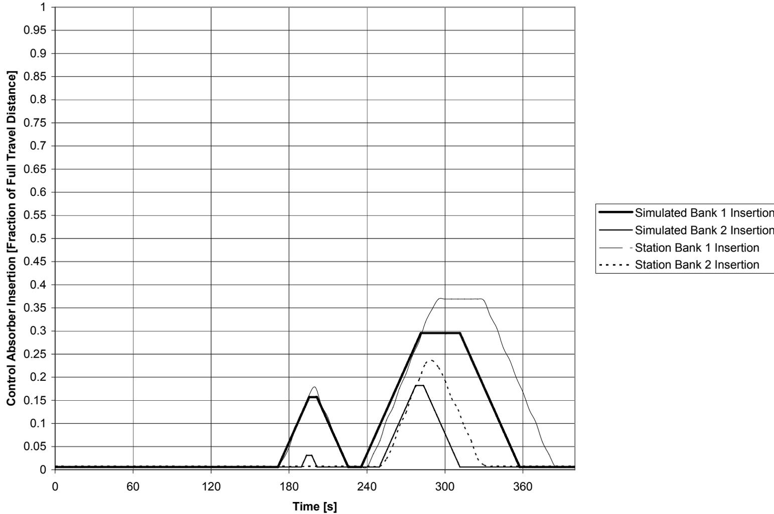
**Figure 6 – Comparison between Simulated Control Absorber Insertion and PNGSB Unit 5 Measured Control Absorber Insertion**
