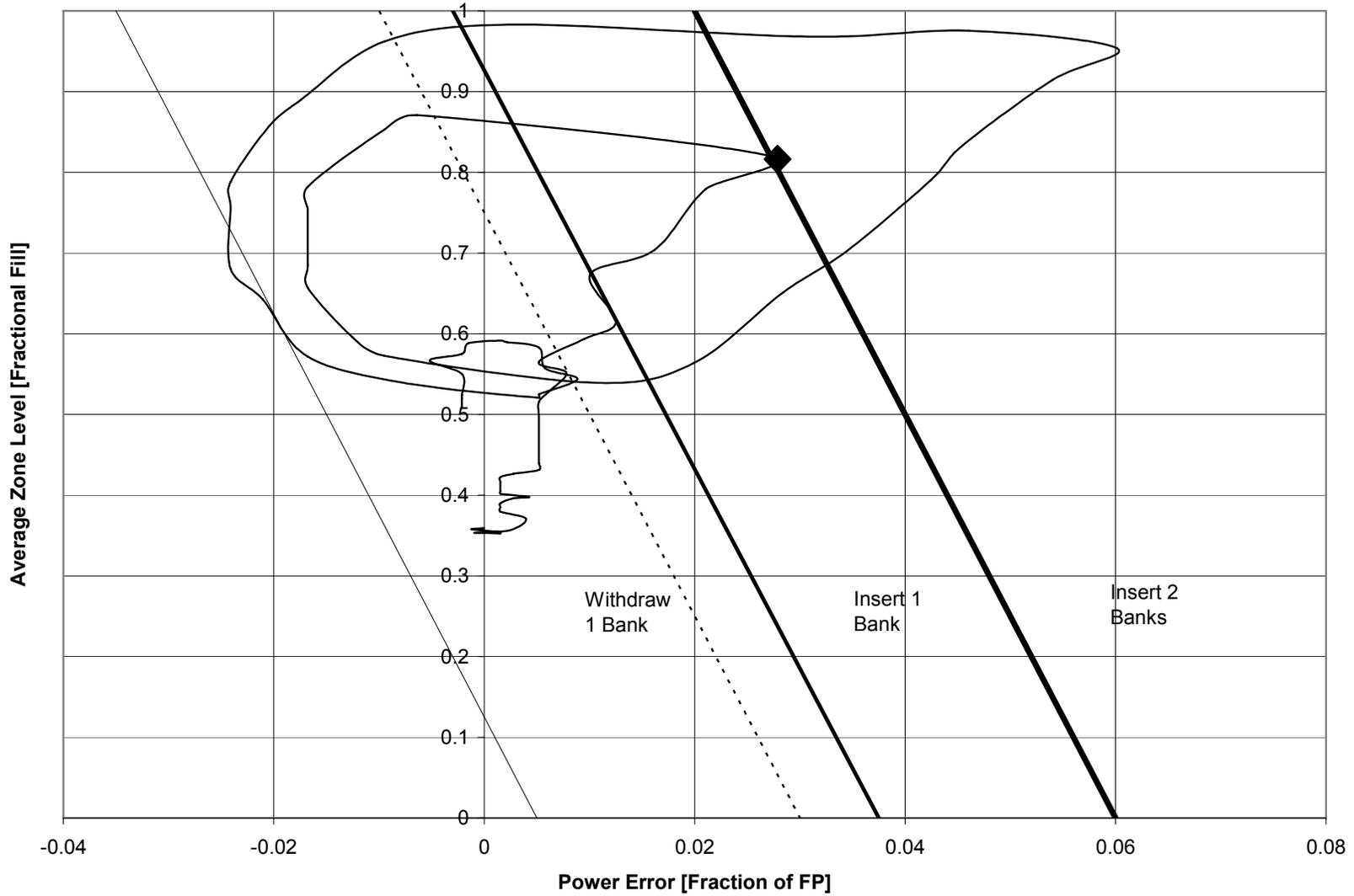
**Figure 7 – PNGSB Unit 5 Station Setback Transient Limit Controller Diagram**
