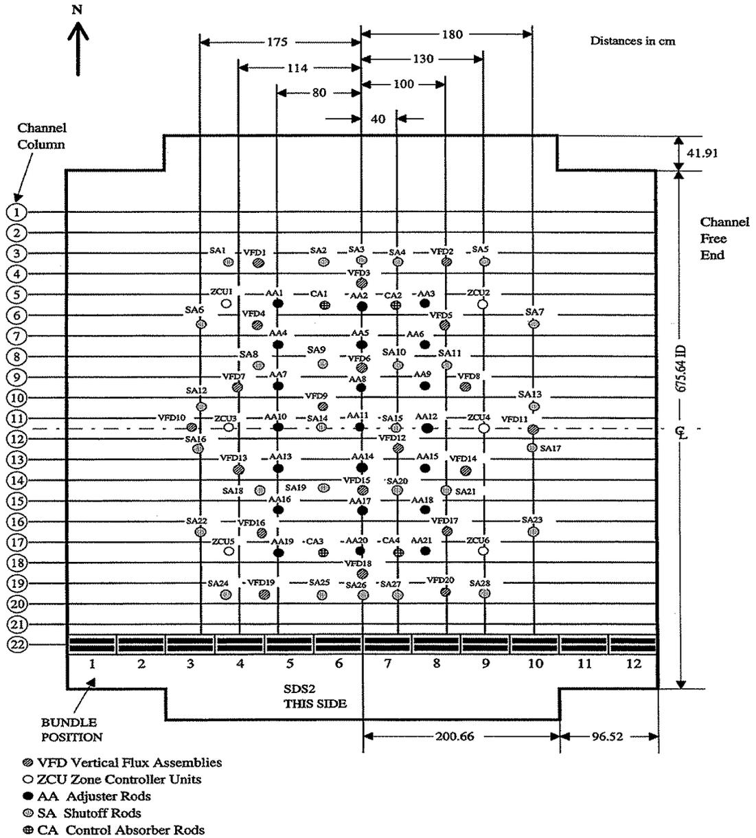
**Figure 1 – Location of Vertical Reactivity control Units**
