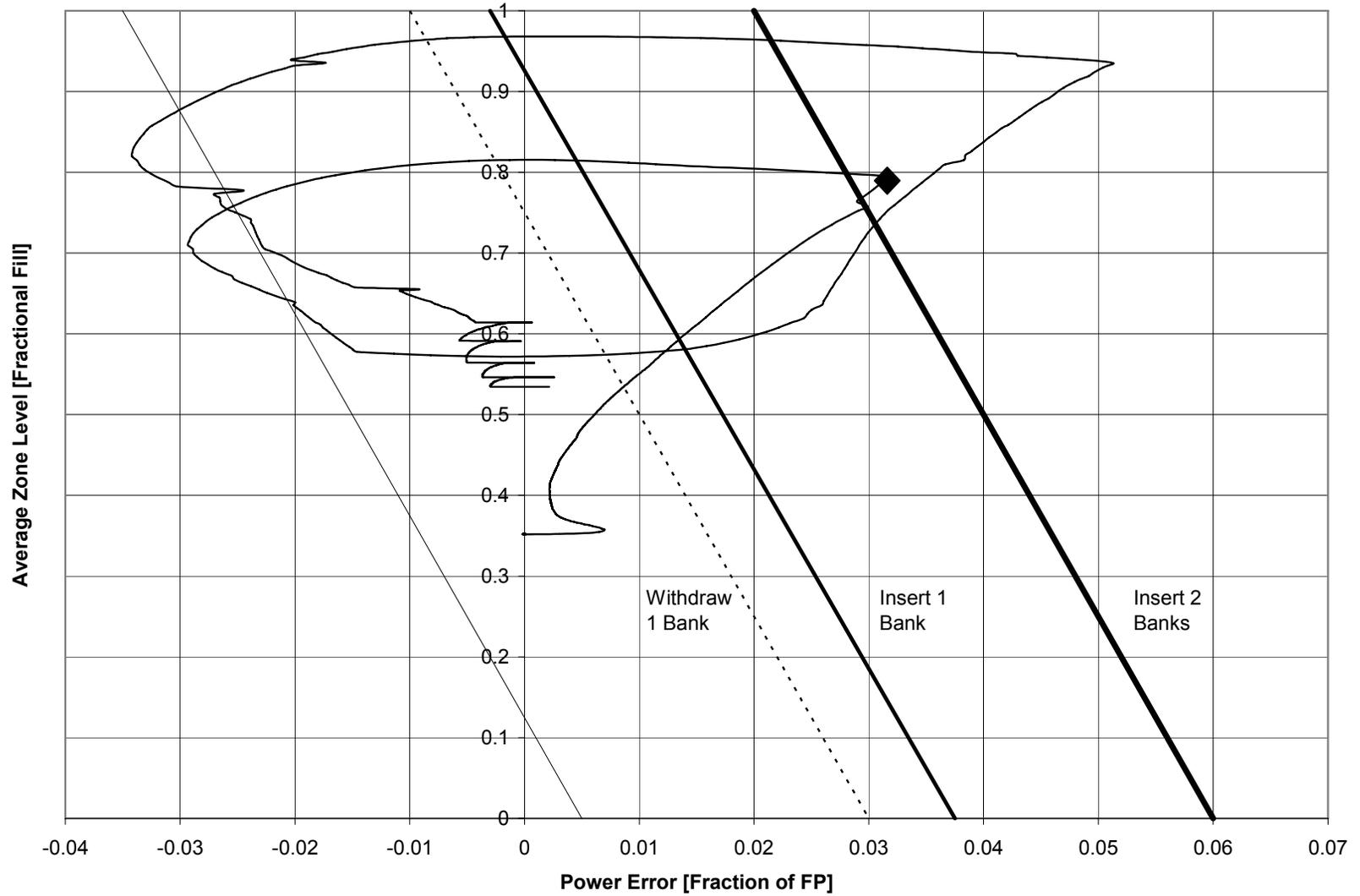
**Figure 8 – Simulated Station Transient Limit Controller Diagram**
