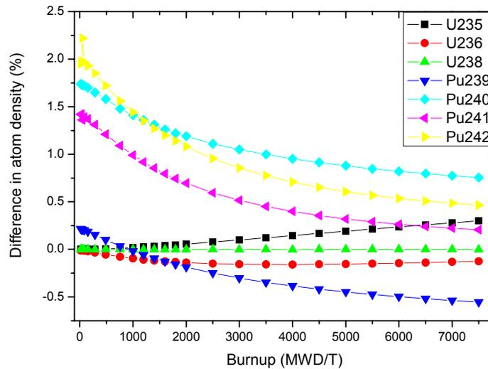
Figure 8 Impact on the actinide density (5% creep, HELIOS calculation).
