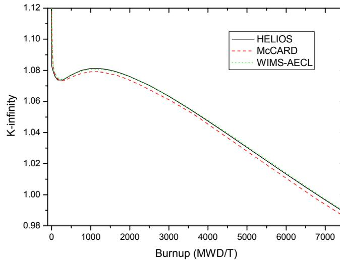
Figure 2 Comparison of the lattice reactivity vs. burnup.
