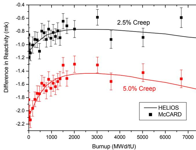
Figure 3 Comparison of the lattice reactivity vs. burnup.
