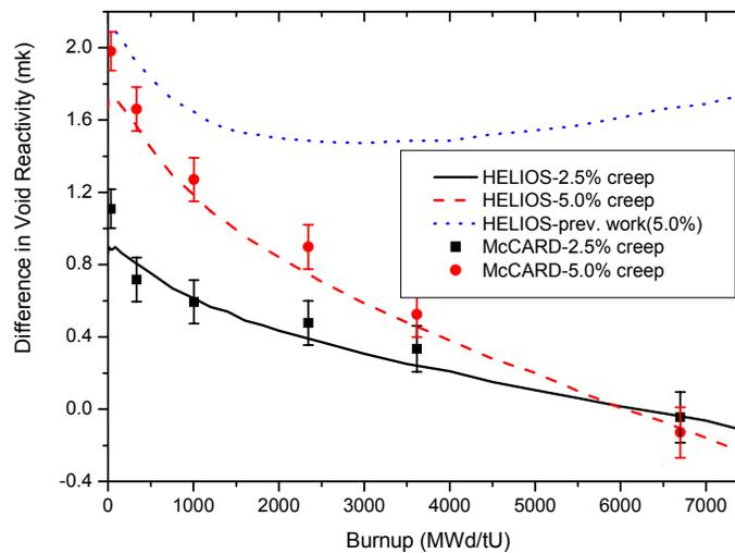
Figure 5 Difference in coolant void reactivity.
