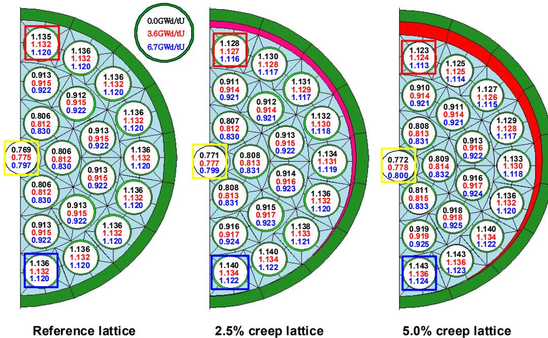
Figure 7 Impact on the pin-power distribution.
