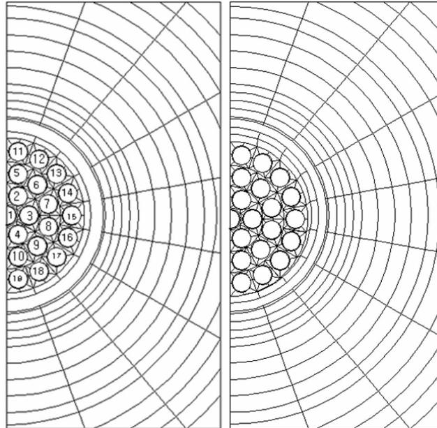
Figure 1 Nominal and perturbed lattice models.
