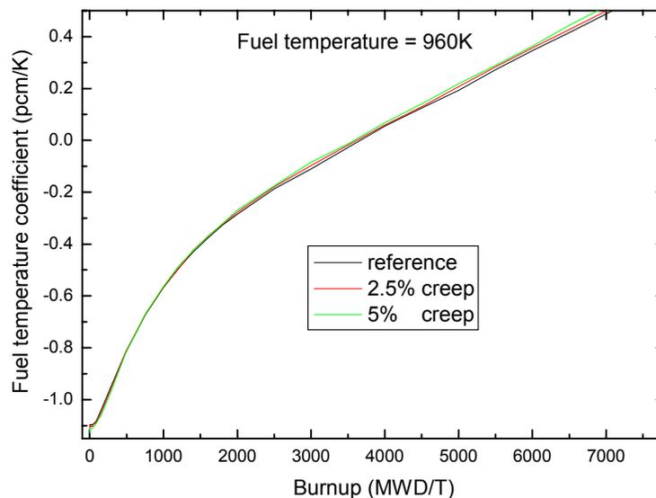
Figure 6 Impact on the fuel temperature coefficient.
