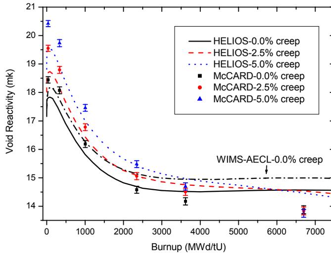
Figure 4 Impact on the coolant void reactivity.
