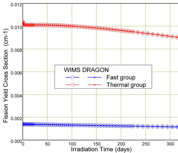
Figure 14 WIMS and simulated DRAGON results of fission yield cross section.
