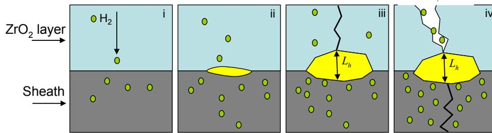
Figure 6: Steps to massive hydriding and secondary failure of sheath in water cooled reactors.
