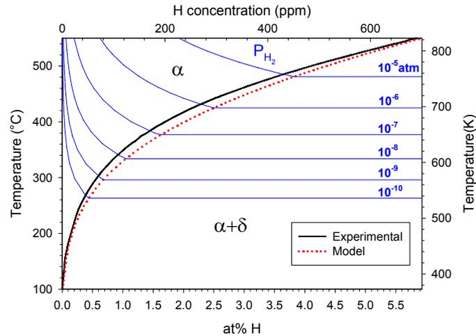
Figure 5: Model comparison of critical  $\alpha/\alpha+\delta$  phase boundary with  $H_2(g)$  isotherms which bears comparison to Figure 2.
