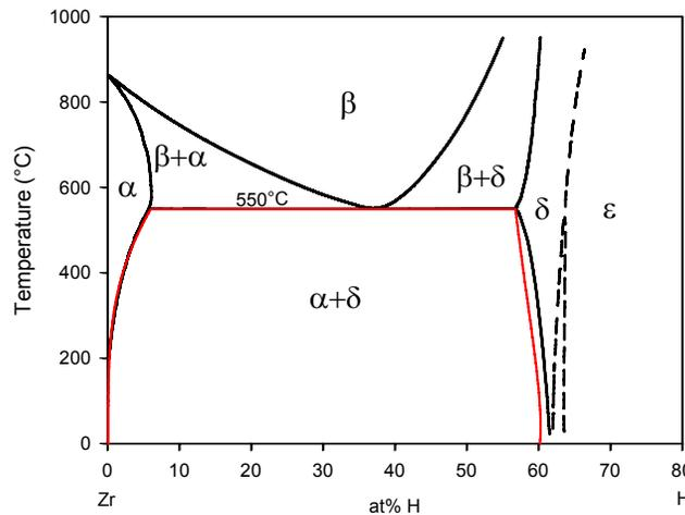
Figure 4: Thermodynamic model and experimental data comparison of  $\alpha/\delta$  equilibrium.
