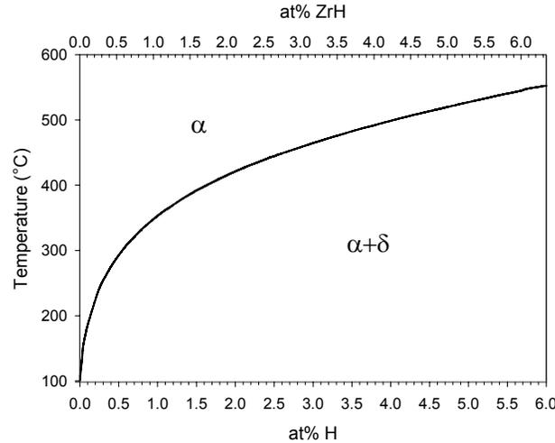
Figure 3: Plot of  $\alpha/\alpha+\delta$  phase boundary with both the atomic percent H and ZrH composition scales.
