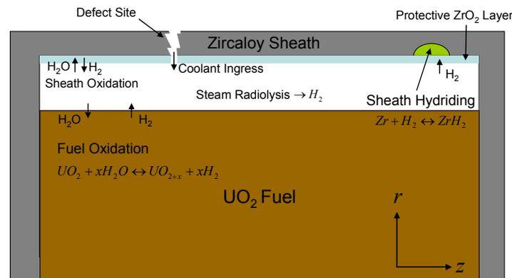
Figure 1: Schematic of the sheath hydriding process (modified from [1]).
