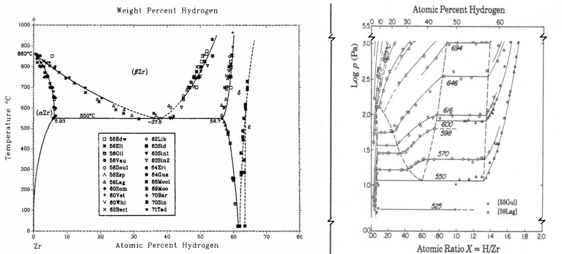
Figure 2: Zr-H binary phase diagram and graph of partial pressure isotherms of H<sub>2</sub>(g) in contact with zirconium at various H/Zr ratios from experimental data of [3].
