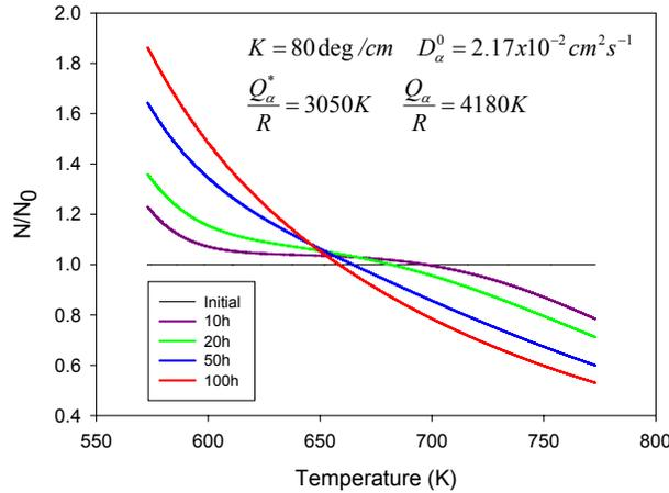
Figure 7: Numerical solution to Eq. (27) ( $T = 573\text{K}$  to  $773\text{K}$ ) using parameters given above.
