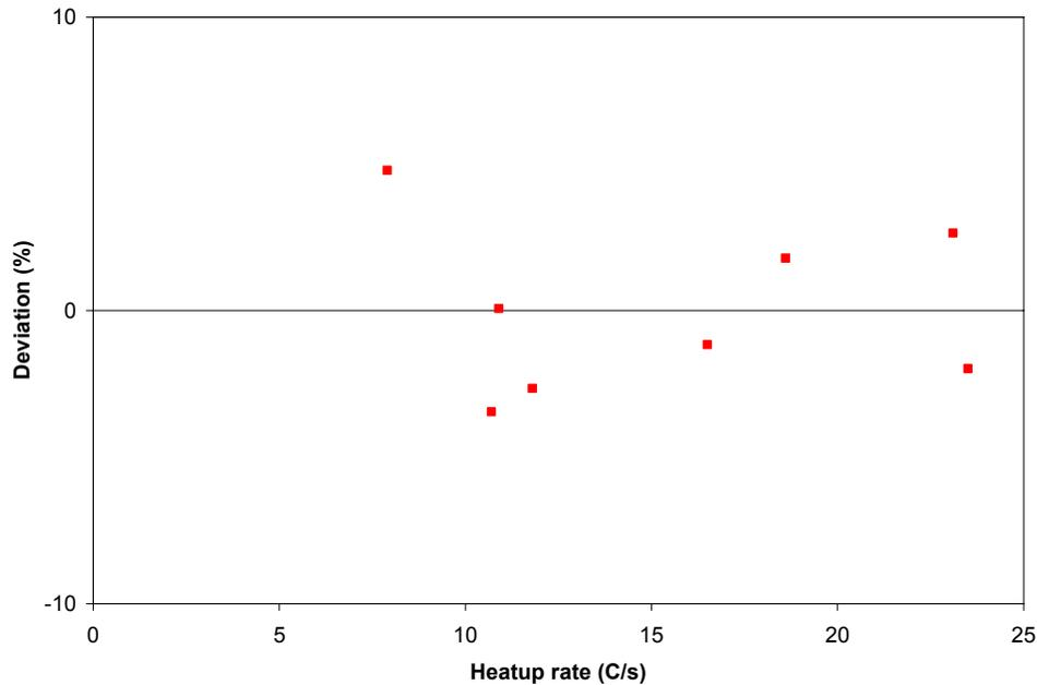
Figure 13 Deviations of data from linear fit of contact temperatures vs. heatup rates for internal pressures around 5.0MPa
