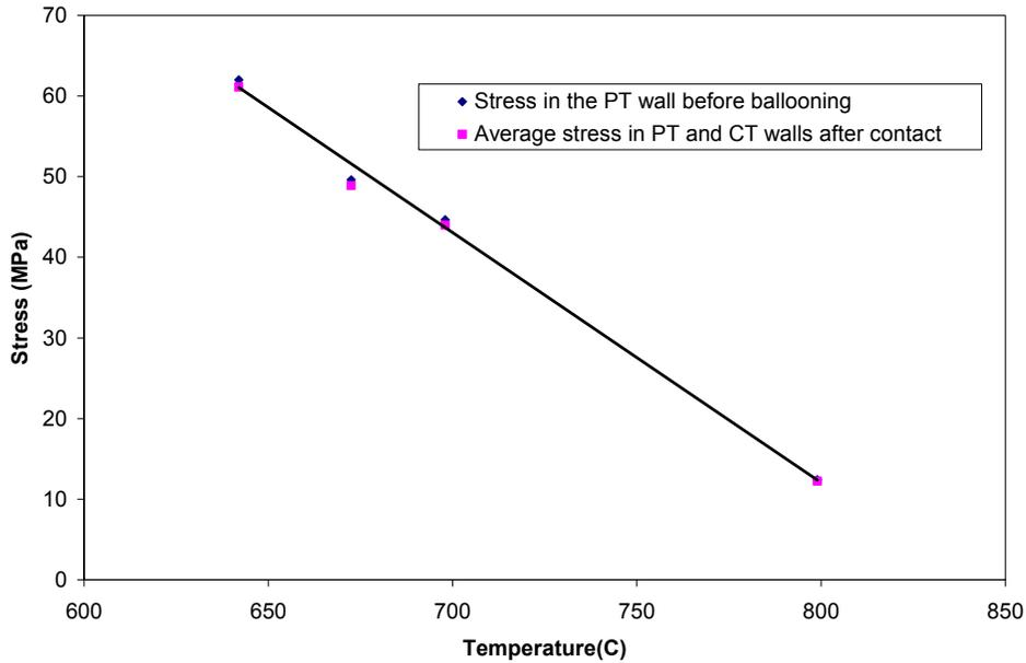
Figure 17 Pressure tube hoop stresses before and after ballooning contact
