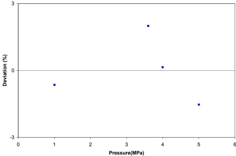
Figure 15 Deviations of pressure tube ballooning temperatures from linear fit vs. pressures
