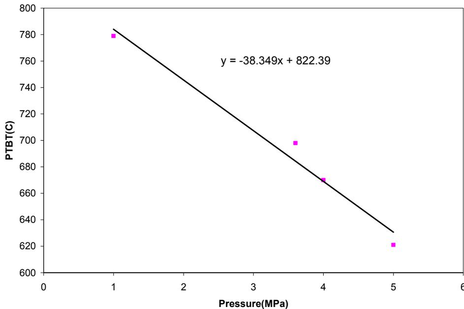
Figure 14 Relationship between pressure tube ballooning temperatures vs. internal pressures
