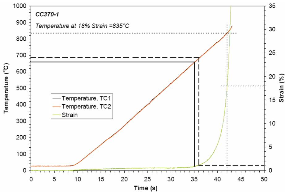
Figure 16 Measured temperatures and strains for sample CC370-1 (Figure C1 in Reference [7], and the thick dashed lines were added for discussion of this work)
