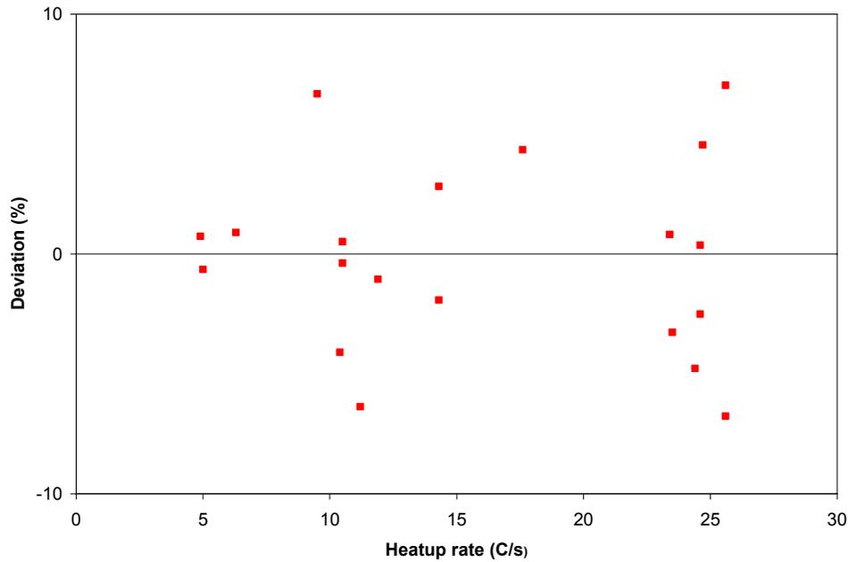
Figure 7 Deviations of data from linear fit of contact temperatures vs. heatup rates for internal pressures around 4.0MPa
