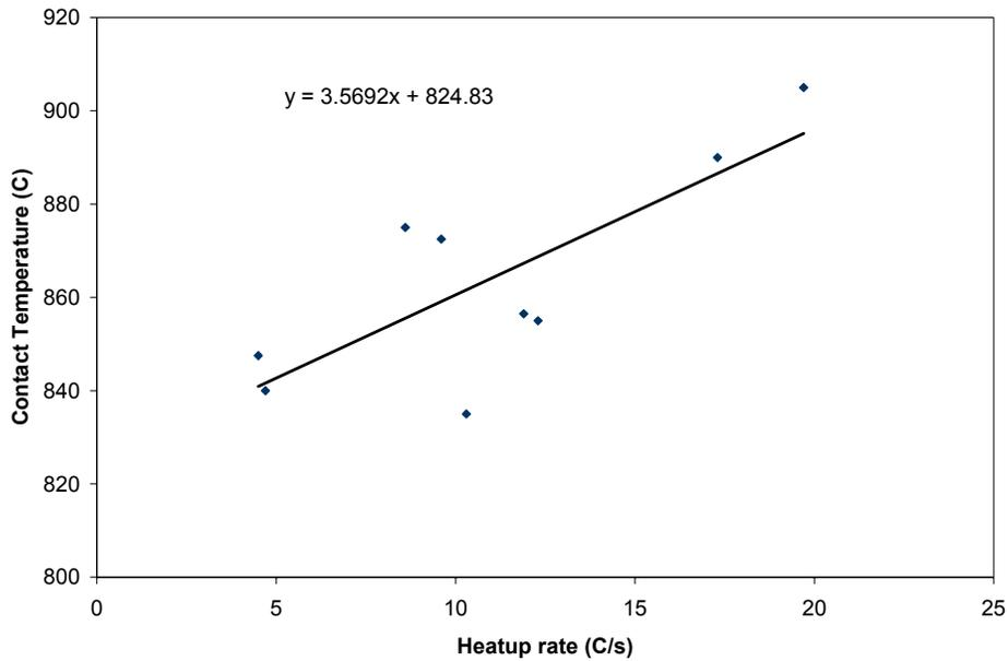
Figure 10 Relationship between average contact temperatures versus heatup rates with internal pressures around 1.0MPa
