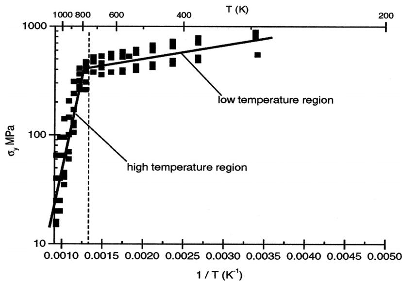
Figure 4 Dependence of the Zr-Nb%2.5 yield stress on the inverse of absolute temperature (Figure 9 in Reference [5])
