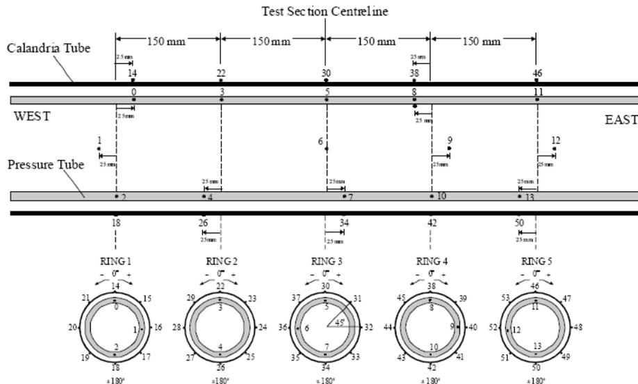
Figure 2 Demonstration of thermal couple arrangement for PT/CT contact experiment (Reference [2])
