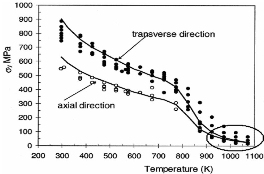
Figure 3 Dependence of the Zr-Nb%2.5 yield stress on absolute temperature for pressure tube material tested in the axial and transverse directions (Figure 8(a) in Reference (5)).
