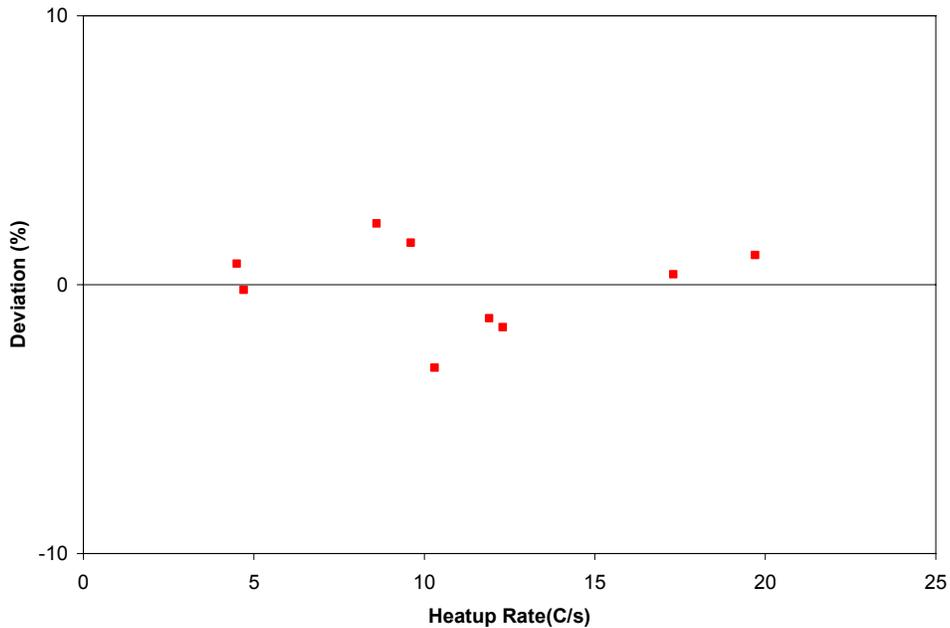
Figure 11 Deviations of data from linear fit of contact temperatures vs. heatup rates for internal pressures around 1.0MPa
