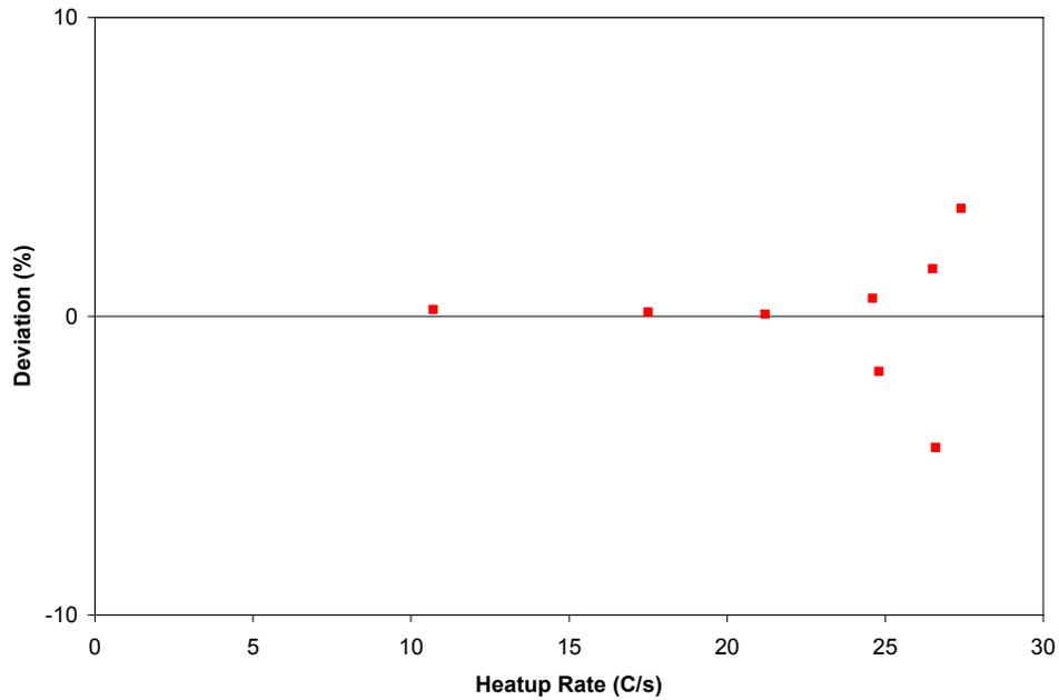
Figure 9 Deviations of data from linear fit of contact temperatures vs. heatup rates for internal pressures around 3.6MPa
