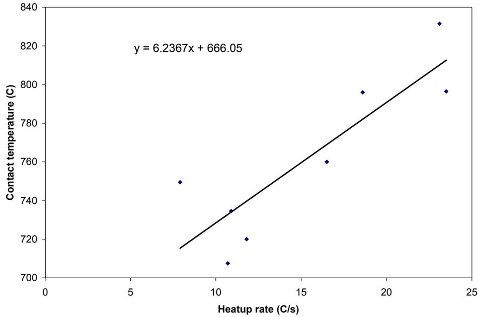
Figure 12 Relationship between average contact temperatures vs. heatup rates with internal pressures around 5.0MPa
