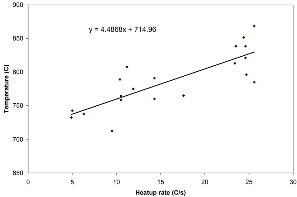
Figure 6 Relationship between average contact temperatures vs. heatup rates with internal pressures around 4.0MPa
