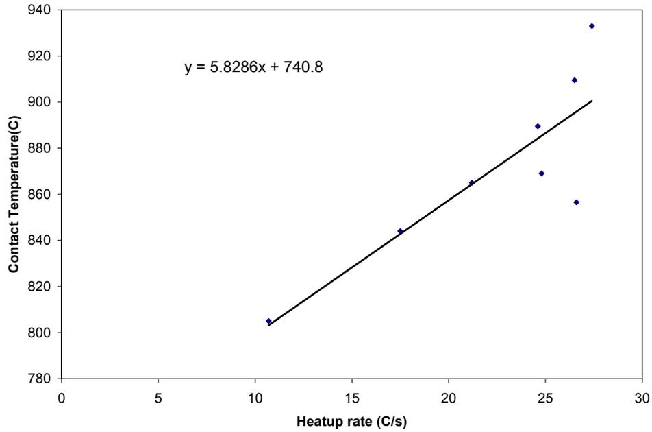
Figure 8 Relationship between average contact temperatures vs. heatup rates with internal pressures around 3.6MPa
