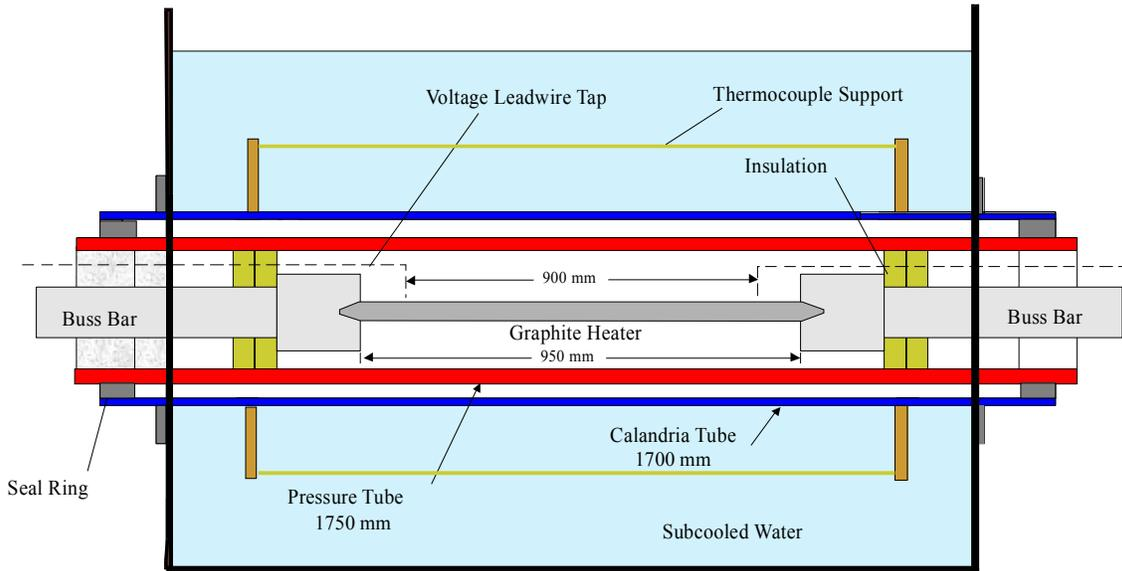
Figure 1 A simplified schematic of PT/CT contact experiment facility (Reference [2])
