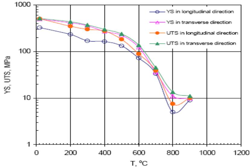
Figure 5 Zr-2.5%Nb alloy temperature dependence of yield strength (YS) and ultimate strength (UTS) (Figure 2(a) in Reference [6])
