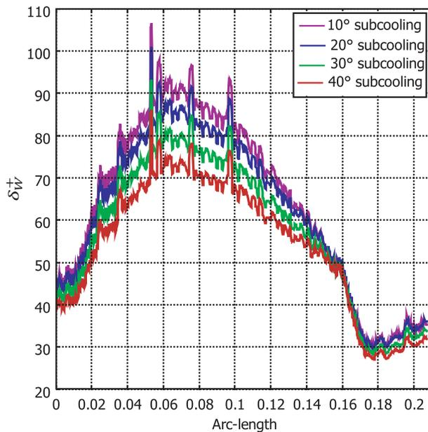
Figure 4. Wall offset in viscous units at the CT surface for various subcoolings
