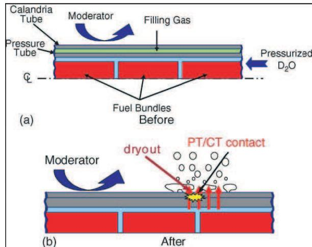
Figure 2. PT/CT contact phenomena: (a) before and (b) after <sup>[13]</sup>
