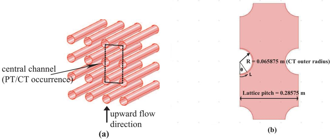
Figure 3. a) part of calandria tubes in 3D, b) the model geometry in 2D
