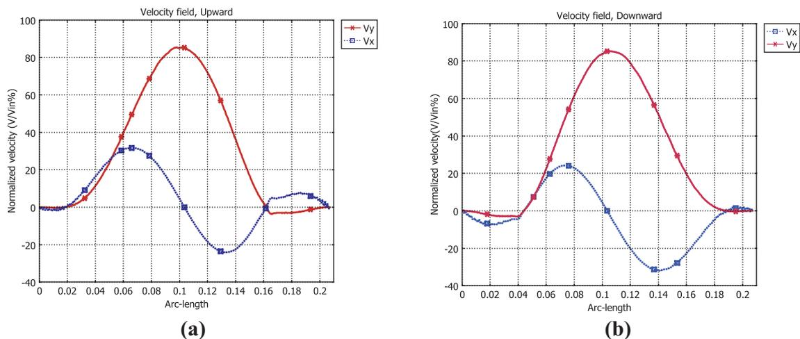
Figure 7. Velocity field around the CT for a) upward and b) downward flows
