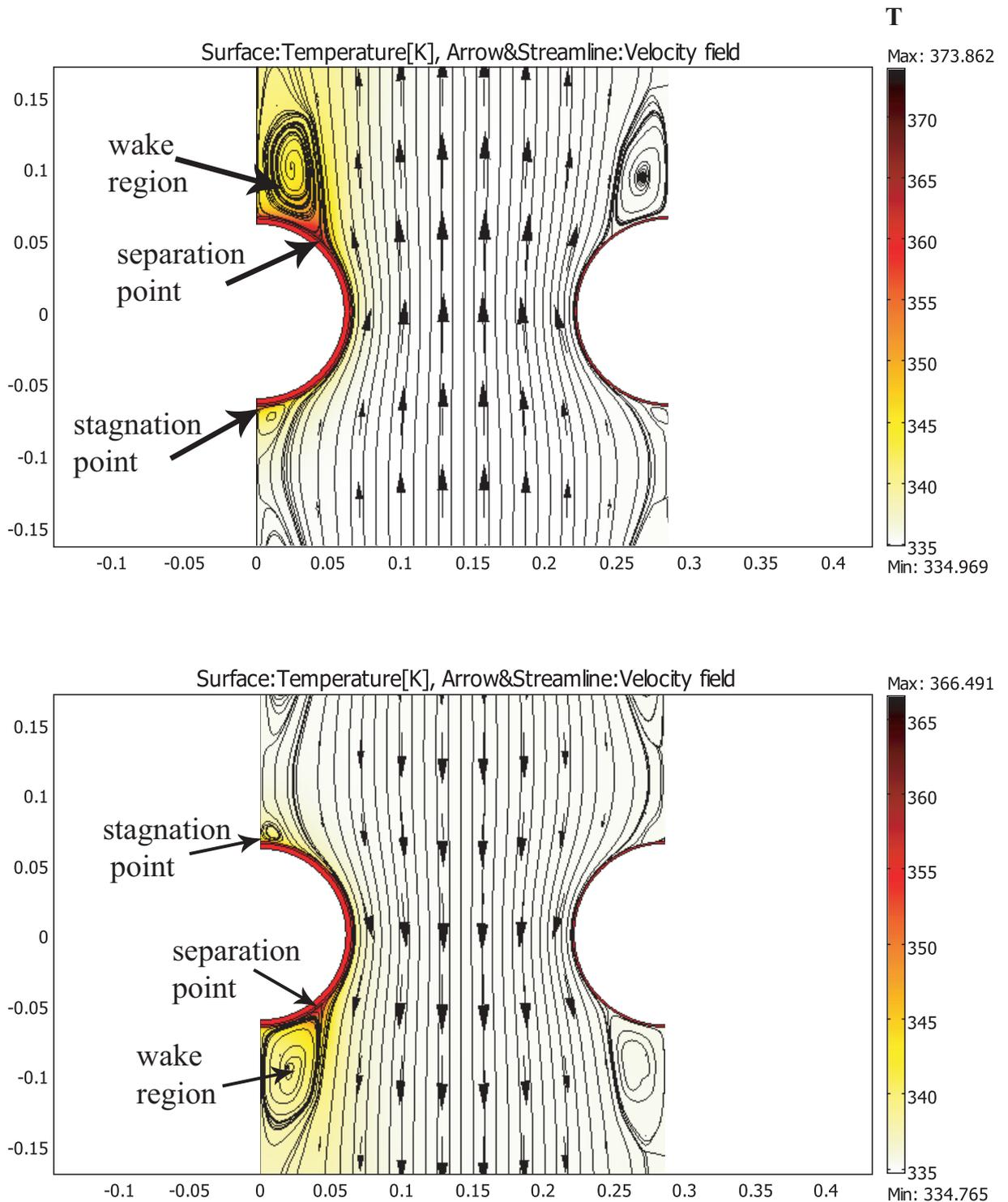
Figure 6. Velocity field around the CT for upward and downward flows
