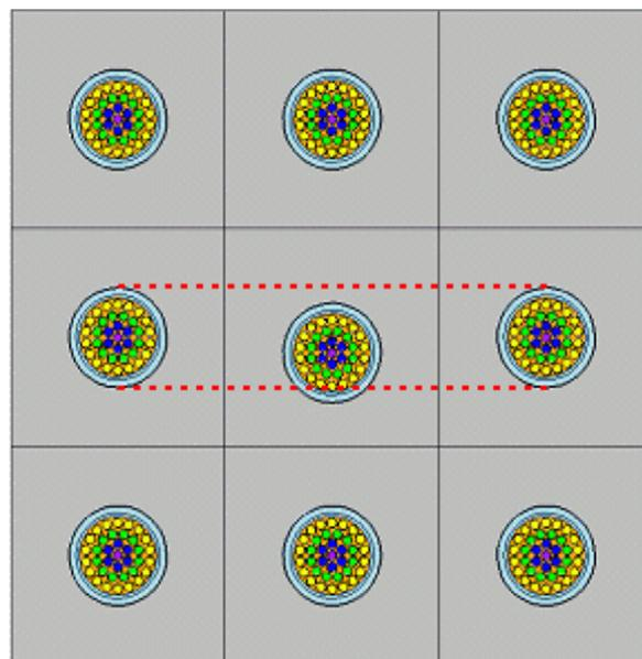
Figure 1 Example of MCNP Geometry for a Sagged Calandria Tube
