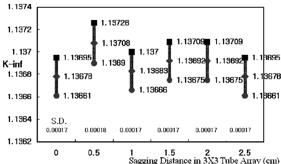
Figure 2 Comparison of k-inf of Sagged Calandria Tube Array
