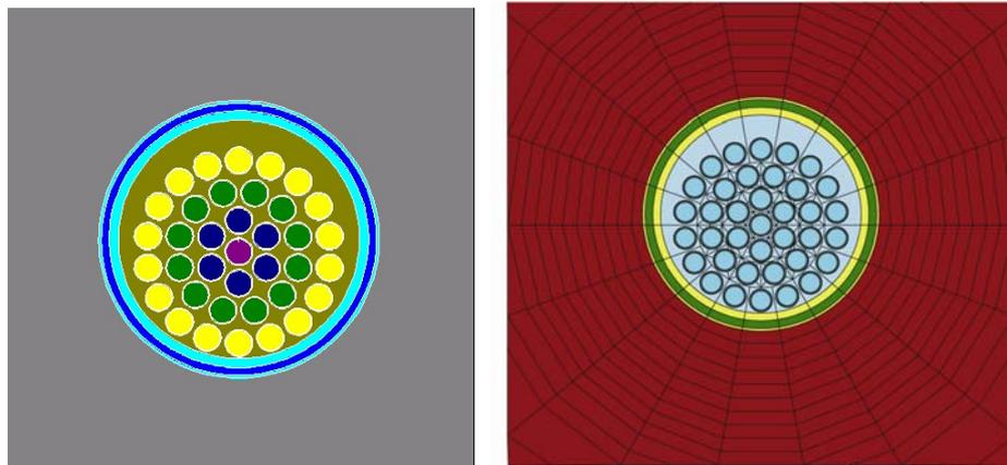
Figure 3 Geometrical Modeling of Deformed Fuel Channels in MCNP & HELIOS
