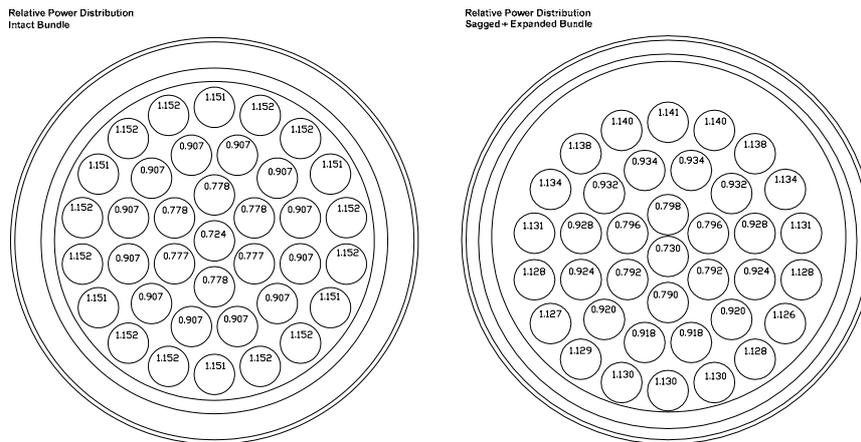
Figure 7 Comparison of Pin Power Distribution (Left: Intact Fuel, Right: Sagged Fuel)
