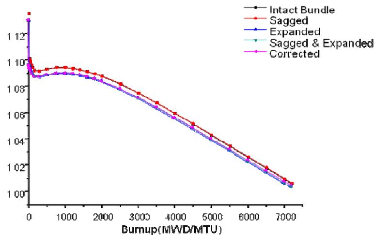
Figure 5 Excess Reactivity of Deformed Fuel Channels vs. Burnup
